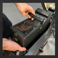
6. When fully charged the battery charger will show a green light. Disconnect the charger from power source and re-insert the battery and connect the power cable.
