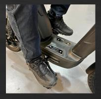
7. Pedal normally, this will engage the motor to the top speed of 15.5 mph.
