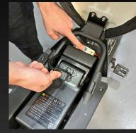
3. Turn the circuit breaker to off and then unplug the power cable from the battery
