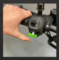
6. **Release** the walk mode button when you have reached a speed up to 4 mph / 6 km/h, then start to pedal.
