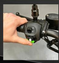
5. **Press** and **Hold** the green walk mode button to get up to 4 mph / 6 km/h.
