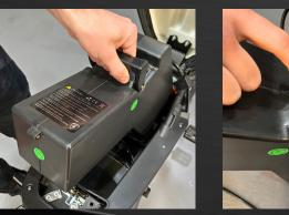
4. Using the handle pull 5. Connect the battery the battery out. 5. to the charging unit an
