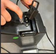
5. Connect the battery to the charging unit and plug into 13 amp electrical socket. Only use the charging unit provided.
