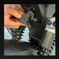
Connect the charging unit to this port on the rear of the SX-250.
