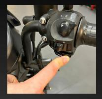
Press the black horn button to sound the horn.
