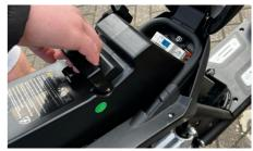
6. When fully charged re-insert the battery and connect the power cable
