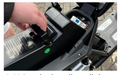
4. Using the handle pull the battery out
