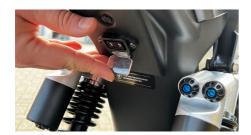
Connect the charging unit to this port on the rear of the bike
