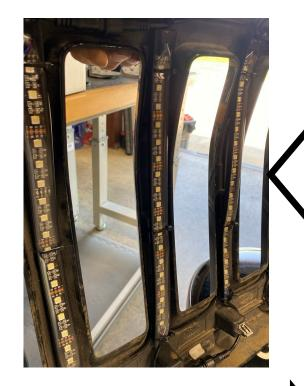
This image shows JL/JT grille with the mesh removed. Attach the strips using zip ties to the sub frame as shown.
