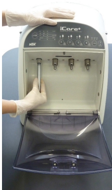
Fig.14 – Connection des turbines
