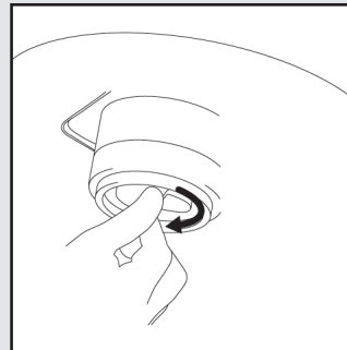
Remove the reverse-threaded impeller
