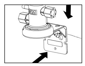
**STEP 8** Install the head and bracket onto the fasteners.
