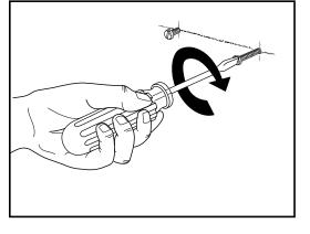
**STEP 7** Allow 1/4"-3/8" (6-10 mm) of each fastener to protrude from the surface.
