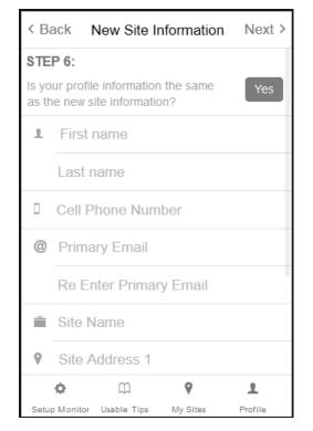
Wi-Fi Monitor Setup - STEP 6 Complete form and then press Next.
