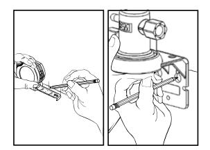
**STEP 5** Mark the locations for the fasteners either by measuring the distance between the bracket holes or using the bracket itself.
