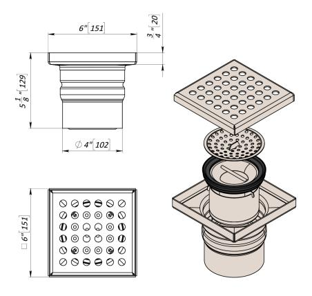
**General:** Floor drain shall be Vodaland Canada FD 6SS Floor Drain as manufactured by Vodaland or approved equal.
