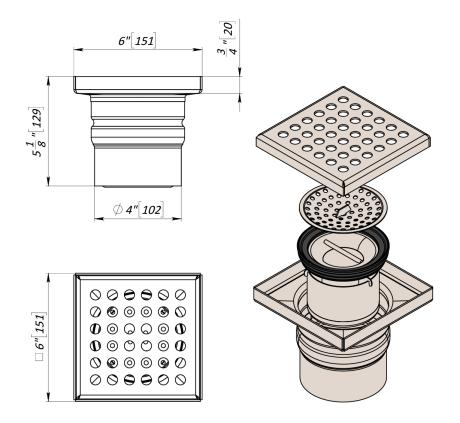
**General:** Floor drain shall be Vodaland Canada 150 FDSS Floor Drain as manufactured by Vodaland or approved equal.
