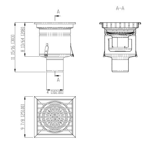
**General:** Floor drain shall be Vodaland Canada FD 250SS Floor Drain as manufactured by Vodaland or approved equal.
