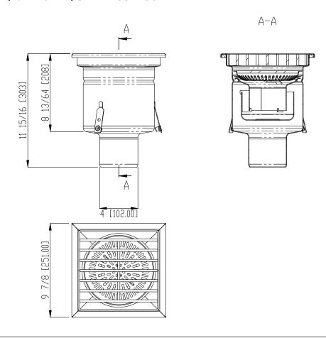
**General:** Floor drain shall be Vodaland Canada FD 10SS Floor Drain as manufactured by Vodaland or approved equal.
