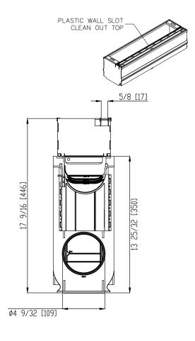
**General:** The SLOT Drain clean-out system by Vodaland Canada consists of the BASE 100P sand trap body with a SLOT removable clean-out top. The trap consists of a polypropylene plastic sand trap, basket, and channel connection adapters, all manufactured by Vodaland Canada.
