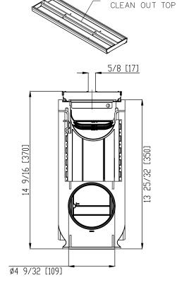
**General:** The SLOT Drain clean-out system by Vodaland Canada consists of the BASE 100P sand trap body with a SLOT removable clean-out top. The trap consists of a polypropylene plastic sand trap, basket, and channel connection adapters, all manufactured by Vodaland Canada.
