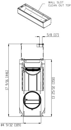
**General:** The SLOT Drain clean-out system by Vodaland Canada consists of the BASE 100P sand trap body with a SLOT removable clean-out top. The trap consists of a polypropylene plastic sand trap, basket, and channel connection adapters, all manufactured by Vodaland Canada.
