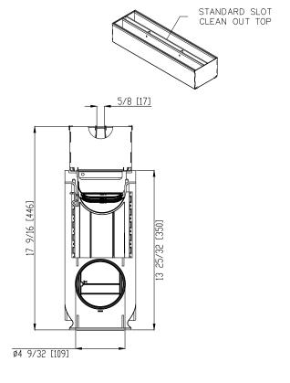
**General:** The SLOT Drain clean-out system by Vodaland Canada consists of the BASE 100P sand trap body with a SLOT removable clean-out top. The trap consists of a polypropylene plastic sand trap, basket, and channel connection adapters, all manufactured by Vodaland Canada.
