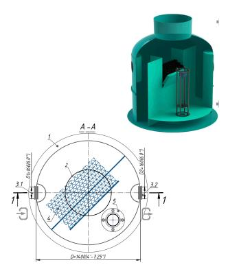
General: The oil water separator shall be Vodaland Canada OILBASE100-6 as manufactured by Vodaland or approved equal.
