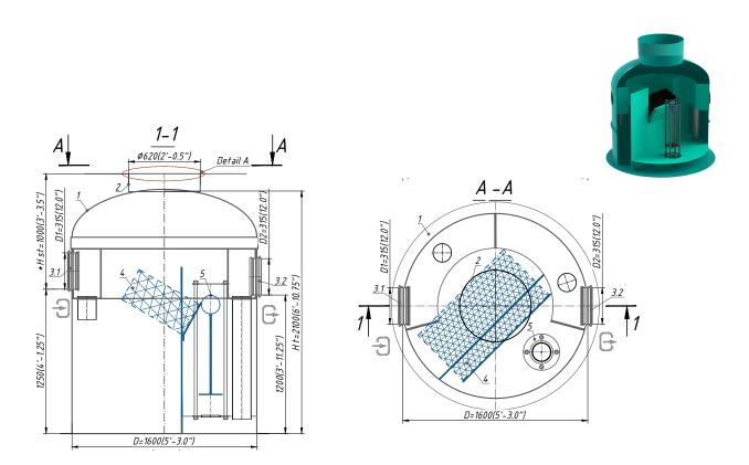
**General:** The oil water separator shall be Vodaland Canada OILBASE100-10 as manufactured by Vodaland or approved equal.
