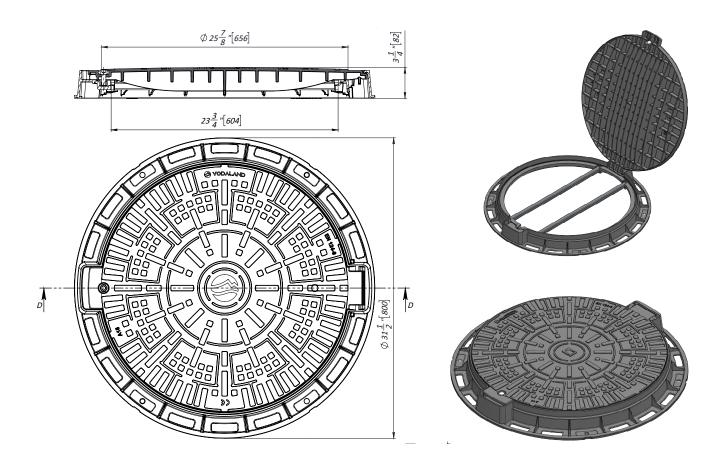
**General:** The manhole cover shall be Vodaland Canada Round Manhole cover as manufactured by Vodaland or approved equal.
