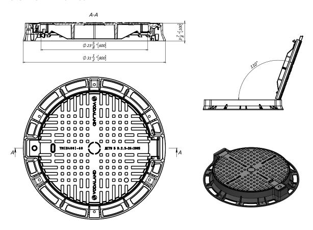
**General:** The manhole cover shall be Vodaland Canada Cast-Iron Manhole cover as manufactured by Vodaland or approved equal.
