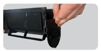
2 Slide end cap from bottom upwards
