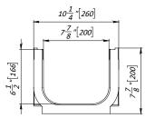
General: The trench drain shall be Vodaland Canada BASE 200P as manufactured by Vodaland or approved equal.
