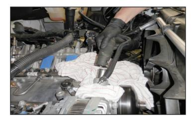
5. Continue with the supercharger installation once you have installed the new water pump and the new A/C belt.
