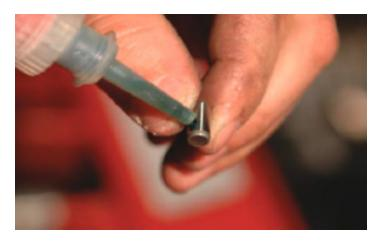
7. Re-install the supplied OEM crank bolt and torque to 239 ft-lbs. Verify your torque wrench setting. We fabricated a tool to hold the crank while torquing the bolt.
