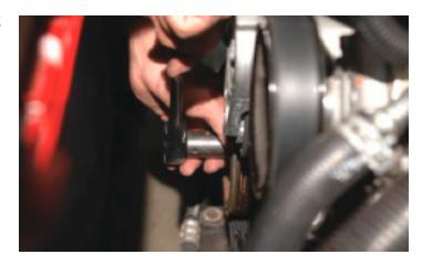
Install the crank pin drill guide with the provided M16x100mm bolt. It's convenient to align the two holes for the crank pins in the drill guide horizontally for ease of access. Torque the temporary bolt holding the drill guide to 40 ftlbs.
