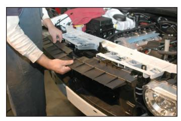
44. For vehicles with hydraulic power steering: The power steering cooler is held to the upper section of the AC condenser with two plastic clamps. Release the clamps by depressing the locking tabs behind the tube and pull the power steering cooler off the mounting tabs.
