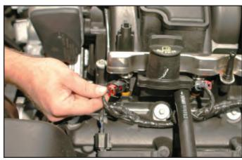
55. On the very back of the OEM intake manifold on the passenger side is the MAP sensor. Disconnect this plug and the mounting push pin clip as well.
