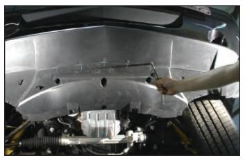
29. Pull the front splash shield from the vehicle. Set aside for re-installation at a later time.
