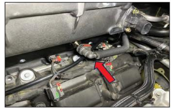
177. Select the coolant reservoir mounting bracket PN 65-26-61-029 and (2) M8X1.25X16 fasteners PN 71-08-12-016. Install the bracket to the LH side of the supercharger using the 2 fasteners as shown. Torque the fasteners to 11 ft-lbs.
