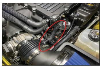
204. If your vehicle has a Mopar cold air intake kit installed, install the ½" rubber plug onto the air box fitting in the location shown. Note: cold air kit upper lid that fastens to the underside of the hood must be removed (insufficient clearance to supercharger)
