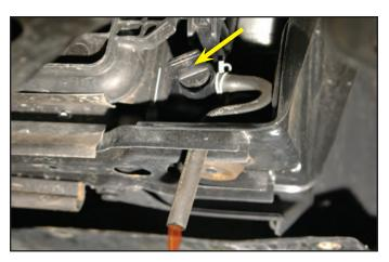
48. Remove the radiator fill cap to relieve back pressure and facilitate drainage.
