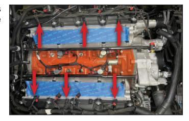
142. Carefully cut and remove the zip tied connections from the harness at all (6) locations.
