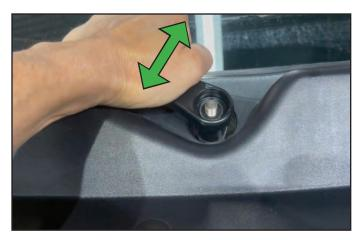
8. Gently remove the fir tree connectors from the top corners of both sides of the cowl.
