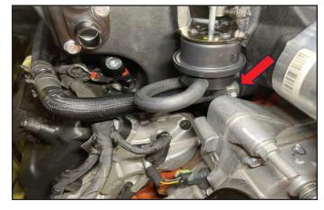
189. Select the length of ½" bulk hose (highlighted in green) from the kit. Install a 21mm constant tension clamp from the kit onto one end of the hose. Apply Lubriplate to the final remaining hose connection on the LH side of the oil separator. Secure the hose to the oil separator using the clamp.
