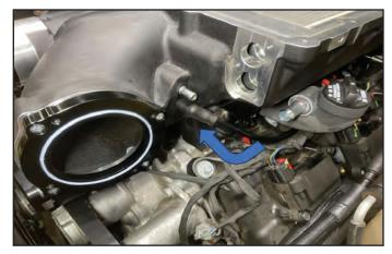
174. Install a 3/8" mender PN 48-46-00-058 (red arrow location) and constant tension clamp (green arrow) onto the end of the brake booster hose. The brake booster hose extension that will be shown in the next step is already attached at the other side of the mender.
