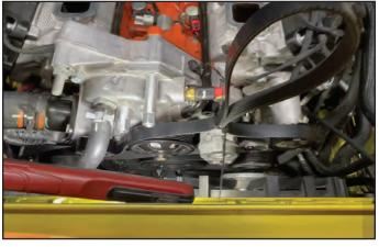
165. Install the bracket sub-assembly onto the front of water pump housing, ensuring the spacers stay on the fasteners. Ensure the belt is routed below the LH stand-off and in between the two idler pulleys as shown. Torque (3) bracket bolts 18 ft-lbs.
