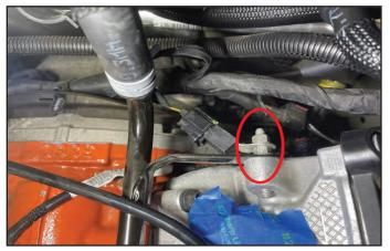
149. Remove the heater tube from the water pump and position it out of the way temporarily.
