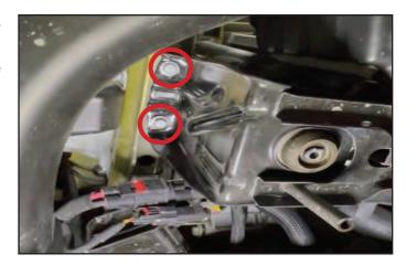
98. The circled threaded hole location will be used for securing the pump mount in the next step.
