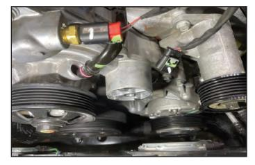
150. Remove the tensioner from the front of the engine using a 16mm socket.
