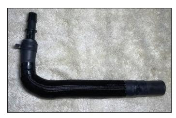
188. Cut approximately 1 inch off the long end of the hose. Install the long end of the hose onto the tube below the supercharger bypass valve in the location shown in the photo. Secure the hose using a small gear clamp.
