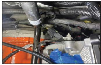
159. Re-install the factory tensioner using a 16mm socket. **Torque the tensioner to 33 ft-lbs.**
