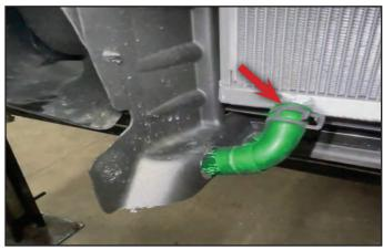
123. Lubricate and install the 4 ft. long section of 1/4" bulk hose onto the bleed port at the top of the LTR. Secure the hose using a constant tension clamp.
