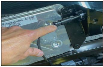
17. Take the PCM to a work bench and remove the (2) nuts that secure it to the bracket. Carefully package the PCM and ship it out to be updated as per the instruction.
