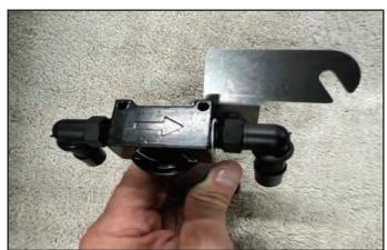
179. Install the vinyl-coated clamp around the base of the separator body in the orientation shown. Select (1) M6X1.0X12mm long fastener and the aluminum bracket from the separator kit. Apply blue Loctite and install the fastener through the vinyl coated clamp and into the rivnut on the bracket. Orient the parts as shown in the photos.
