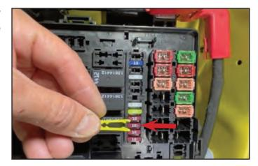
114. Select the new 10amp fuse P/N 82-55-50-210. Slip the fuse into the slot in the end of the brass connector on the yellow trigger lead.
