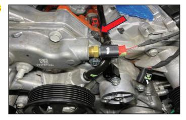
158. Re-install the radio capacitor onto the stud at the back of the LH cylinder head. Secure the sensor with the original nut. Torque the nut to 96 in-lbs.
