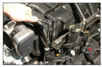
61. Pull the OEM intake manifold forward a bit to gain access to the brake booster hose plugged into the back of the manifold. Disconnect this hose from the rear of the intake manifold. There is also a wire loom clamp located at the back of the intake manifold that needs to be pulled free or cut off.
