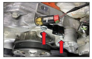
154. Lubricate the o-ring on the heater tube and re-install it into the water pump housing.
