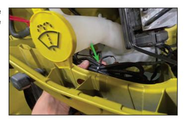
108. Remove the fuse box cover by squeezing the tabs on each side. Set the cover aside.
