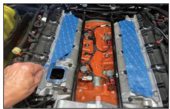
167. With the aid of a helper, install the supercharger onto the engine
