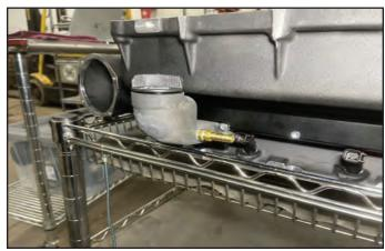
135. Sub-assemble o-ring PN 80-59-10-128 onto the PCV adaptor shown below. Install the PCV adaptor onto the RH side of the supercharger, with the hole angled upward using (4) M6X1.0X20mm long fasteners PN 71-06-10-020. Torque bolts to 96 in-lbs.
