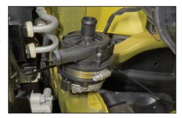
102. Select the intercooler pump relay harness. Route the end with the connector in front of the windshield washer bottle and across the front of the vehicle above the radiator then down toward the plug on the pump. Zip tie the I/C harness to the existing wiring and/or hood latch cable as necessary.
