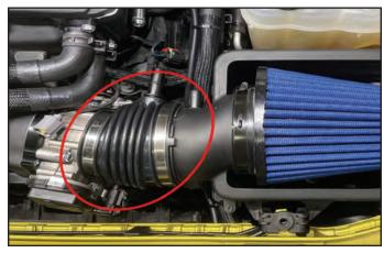
203. Install the 6 inch long piece of 5/8" I.D. rubber hose between the clean air tube and the oil fill adaptor. Secure the rubber hose using (2) 5/8" constant tension clamps as shown.
