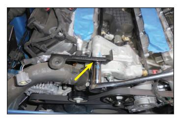
68. To facilitate the hose install, use a long 3/8" drive ratchet to spring the tensioner and remove the OEM fan belt. This belt will not be reused.
