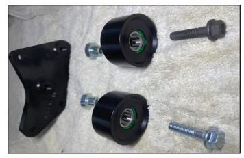
146. Idlers must be installed with the snap ring facing the stand-off on the idler bracket. Clamp the idler and bracket sub-assembly in a vice to secure it then torque the fasteners to 27 ft-lbs.
