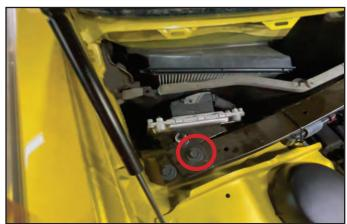
15. Lift the PCM up and out of its mounting location. Depress the locking tabs and cycle both connectors to remove them from the PCM.
