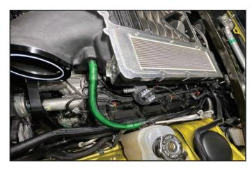
176. Re-connect the fuel line to the fuel rail on the LH side of the supercharger. Ensure the connector is fully seated, you will hear it click into place. Cycle the red lock on the connector. Pull back on the connector ensuring it does not come off.
