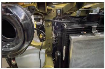
103. Plug the I/C pump harness/adaptor into the pump.
