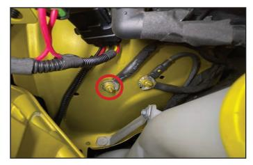
110. Install the BLACK ground wire onto the factory ground stud. Re-install the nut the tighten it.
