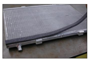
88. Cut the adhesive backed rubber strips and affix to the inside surface of two of the supplied heat exchanger mounting hooks. Apply a strip of the adhesive backed foam to the remaining heat exchanger mounting hook.
