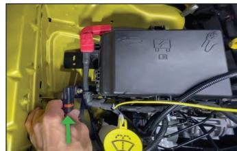
107. Zip tie any extra harness and secure it to the existing vehicle harness by the windshield washer tank.
