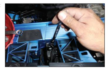
94. Attach the remaining carriage bolt to the passenger side mounting slot on the bottom of the heat exchanger. The remaining vibration damper foam backed bracket will clamp over the bottom of the air conditioning condenser and be secured to the carriage bolt just installed using the remaining 12mm headed nut.
