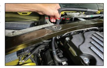
186. Tape back the protective sleeve as shown, then install a 21 mm constant tension clamp to the hose end. Apply Lubriplate to the RH barb on the separator then install the hose over the barb and secure it with the clamp as shown.
