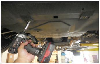
25. Start removing the push pin rivets by prying out on the center spreader and then pull the rivets free. There are 3 push pin rivets on the driver's side and 4 on the passenger side. Now remove the two 10mm headed bolts joining the two main components together. Next remove the two rear 10mm headed bolts from the back splash shield.
