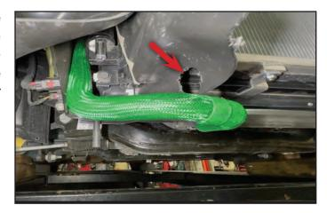
122. Route the hose (highlighted in green) from the last step through the hole, install a constant tension clamp to the end then install the hose onto the LTR. Secure the hose using the clamp.
