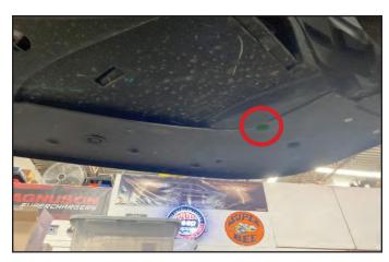
28. Remove the seven 7mm bolts from the front of the splash shield where it joins the spoiler.
