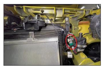
104. Using an M6 X 20mm long bolt and nut from the kit, secure the intercooler relay and fuse to the end of the black bracket next to the fuse box as shown.
