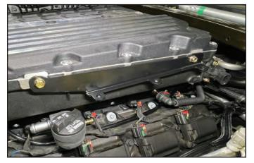
178. Select the oil separator assembly from the kit. Note the airflow direction on the top of the separator.
