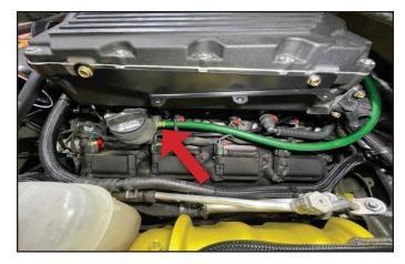
182. Install the opposite end of the hose (highlighted in green) from the last step to the bottom port of the separator ensuring it is fully seated.
