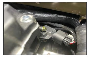
193. Gather the supercharger coolant reservoir. Use (3) M6X1.0X16mm long fasteners PN 71-06-10-016 to secure it to the bracket on the LH side of the supercharger.
