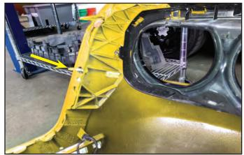
35. Carefully but firmly pull outward on the fascia near the side reflector to disengage the plastic mounting clips on each side of the vehicle.
