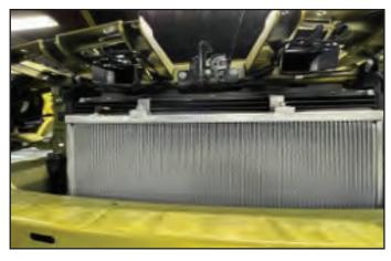
96. Here is the final bottom LTR mounting location with the two shorter brackets. Note: Some vehicles may have a longer condenser and require the use of 2 long mounting tabs, which are included in this kit.
