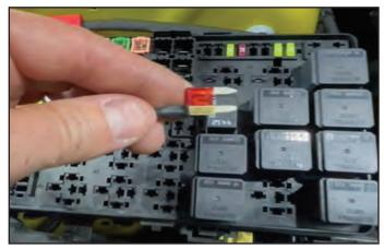
115. Re-install the new fuse/tap assembly back into the factory location, ensuring it is fully seated. Route the yellow trigger wire through the fuse box as shown. Notch the edge of the box to allow the wire to exit at the arrow location.
