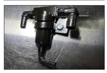
180. On the vehicle, remove the factory bolt securing the wiper assembly to the cowl in the location shown. Install the separator assembly under the steel washer then reinstall the factory bolt and tighten it to secure the separator.
