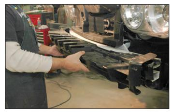
41. Pull out the center post of the plastic push pin rivets and remove the 4 rivets shown here.
