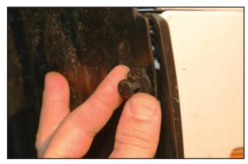
33. Once the rivets are out, pull back on the wheel well shroud to expose the bolt by the junction of the fender and the fascia and use a 10 mm wrench to remove the bolt on each side of the vehicle.
