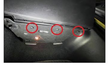
20. Hinge the cover plate down to provide access to the underside of the dash. Locate the factory CAN-BUS connector in the encircled area. Plug the small white connector from the supplied cable into the factory CAN-BUS system in any open port.
