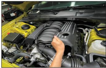
51. Unplug the IAT from the intake air tube. Note: If equipped with a PCV fresh air line running to the airbox, disconnect it now.
