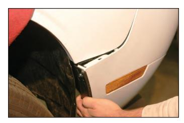
36. From the top of the vehicle, where the corner of the fender by the hood attaches to the fascia with a 10mm nut on the fascia mounted stud loosen this nut/washer and remove from each side of the vehicle.
