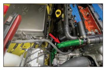
121. The hooked end of the hose from the last step is shown in the location below the vehicle where it is routed. Drill a hole in the plastic shield at the bottom right corner of the radiator (red arrow) to allow the intercooler hose to pass through.
