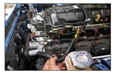
58. CAUTION: Fuel line may hold residual pressure. Wear safety glasses to protect your eyes. Use shop towels to capture any residual fuel and dispose of it properly. Remove the fuel line from the fuel manifold on the driver side. For earlier models you will press on the blue tabs of the fuel line locking clip and then pull the line free. For late models see the step below.
