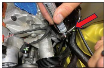
155. Re-install the factory bolt securing the heater tube to the water pump housing but do not tighten it.
