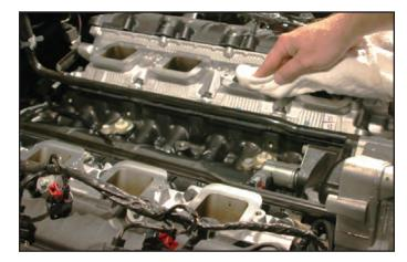
66. Use tape or shop rags to cover the exposed ports and prevent debris from entering the ports.
