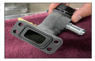
134. Install the oil fill adaptor to the LH side of the supercharger using (4) M6 X 1.0 X 20mm long fasteners PN 71-06-10-020. Torque bolts to 96 in-lbs. Prototype shown.
