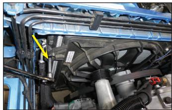
71. Remove the fan shroud from the bottom. The assembly will be reused. NOTE: Loosen the 4 (13mm socket) bolts holding the lower radiator bracket to the frame. Remove 1 bolt on each side. This will allow room for the shroud to be removed.
