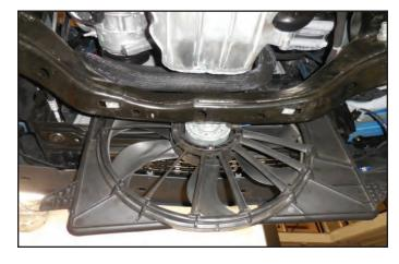
85. Anchor the fan shroud in place using the two OEM mounting bolts.
