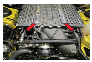
192. **6.4L engines Only:** install MAP sensor jumper harness PN 82-55-80-042 between the new sensor at the LH rear of the supercharger and the factory connector at the RH rear of the engine compartment.
