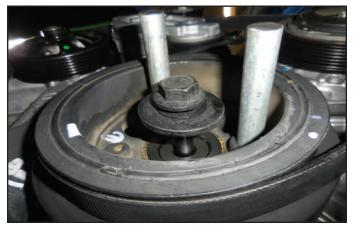
73. Use a pry-bar or long heavy duty screwdriver to anchor the pulley using alternate sides of the dowels you pushed in the pulley holes as shown. This will give you a lever to stop the pulley from turning. Now, use a 21mm wrench to remove the crank harmonic balancer pulley bolt. Set aside for later use along with the two provided dowels.
