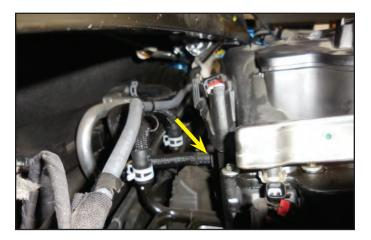
62. Carefully lift the OEM intake assembly from the vehicle.
