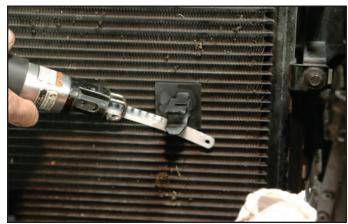
47. Ensure that the engine has had time to cool before draining the coolant. Open the drain valve on the bottom of the passenger side radiator. Collect the drained fluid in a clean pan and set aside for later re-use.
