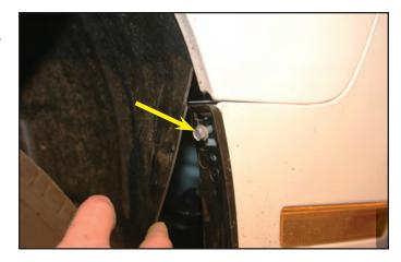
34. Using a 10 mm socket remove the bolt on each side of the fascia midway up. It is easiest to reach it from the bottom side of the vehicle. (Fascia shown off vehicle for bolt location clarity)
