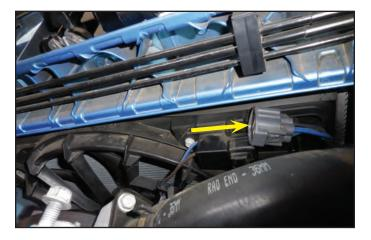
70. Use an 8mm wrench to remove the two fan shroud mounting bolts, there is one bolt on each side of the shroud.
