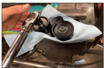
147. Remove the fastener holding the heater tube to the water pump casting in the location shown.
