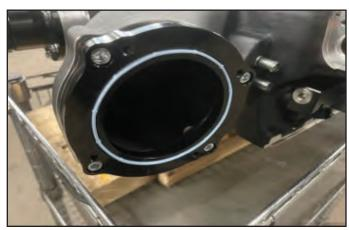
140. Select the supercharger pulley PN 57-03-06-090-BL and (4) fasteners PN 71-06-10-016. Apply blue Loctite to the fasteners then install the pulley onto the front of the supercharger. Torque the fasteners to 106 in-lbs.
