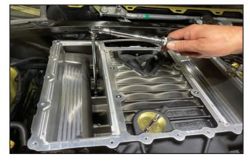
169. Re-install the charge air coolers into the supercharger ensuring the coolant ports line up with the holes in the front of the housing. Apply blue Loctite to (6) inboard CAC fasteners and re-install them. Torque them to 84 in-lbs. Ensure the (4) black o-rings are in place as shown in the photo.
