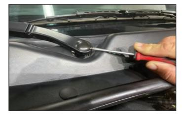
6. Using a 15mm socket, remove the nuts that secure both wiper arms to the posts.
