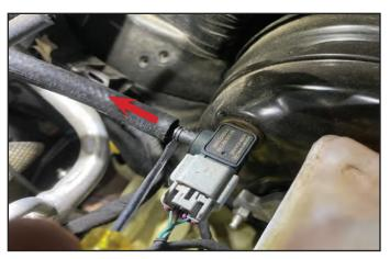
144. Flip the hose 180 degrees and install the opposite end to the booster so that it routes toward the LH front of the engine.
