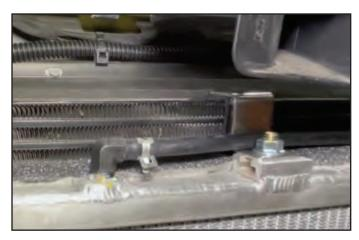
124. Route the hose (highlighted in green) along the top of the LTR and toward the LH side of the vehicle, then through the radiator cradle at the top left corner of the radiator. Final routing and connection of the hose will be detailed in a subsequent step.
