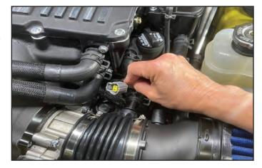
206. **6.4L Engines Only:** Route the jumper harness under the front of the supercharger and over to the sensor located on the RH front corner, under the bypass valve. Plug the harness into the sensor ensuring it locks into place.
