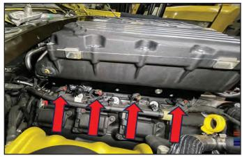
173. Route the fuel vapor line along the LH side of the engine toward the front of the supercharger. Cyl. #3 coil fasteners may be required to be removed to allow the vapor line to route under the engine oil fill adaptor. Install the fuel vapor line onto the lower port of the supercharger as shown. Re-install the coil bolts if removed. Torque 89 in-lbs.
