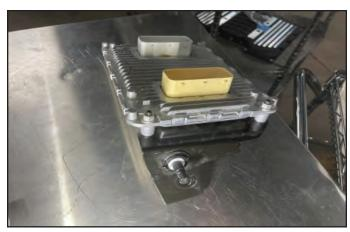
208. Re-install the PCM / bracket sub-assembly back in the RH side of the cowl. Re-attach both PCM connectors and the hood latch sensor connector.
