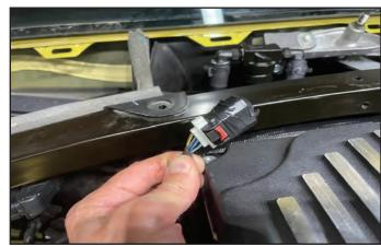
211. Re-install the cowl cover, ensuring the clips locate back into their respective locations. Re-install all push pins.
