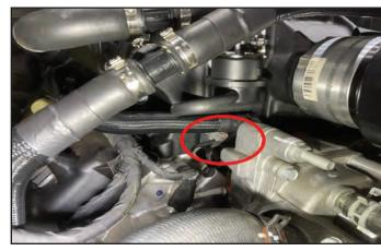
207. Re-install the bracket to the PCM in the orientation shown. Secure the bracket using the (2) factory nuts.
