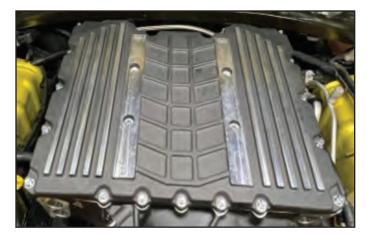
126. Remove (6) internal fasteners securing the CAC's to the base.
