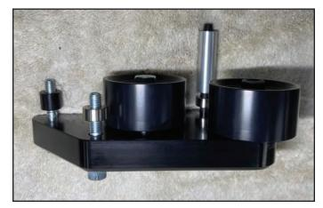
161. You will find an assembly drawing of the FEAD Idler bracket assembly at the back of this manual. There is one for 2009-2010 model years and another for 2011+.
