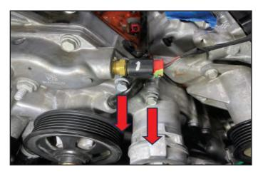
152. Select the following parts: Bracket (PN 65-26-61-025), M8X1.25X110mm long fastener (PN 71-08-12-110), and M8X1.25X40mm long fastener (PN 71-08-12-040). Sub-assemble the fasteners into the bracket as shown in the photo.
