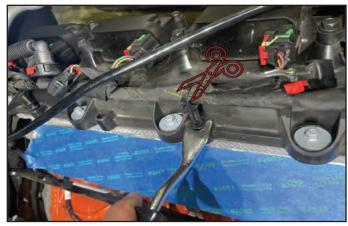
143. Remove the factory brake booster hose from the brake booster.
