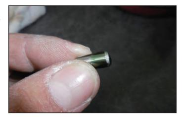
82. Use a hammer and drift-pin or nail-set to tap the crank pins in completely. Ensure that they are in completely, and will not touch the surface of the crank bolt directly when installed.
