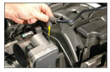
57. Disconnect the PCV vent hose from the air box and the oil fill spout extrusion.
