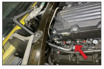
185. Determine the appropriate place to cut the hose (shown at the dashed line) so that will connect to the RH side of the oil separator. Cut the hose (do not throw away the remaining section).
