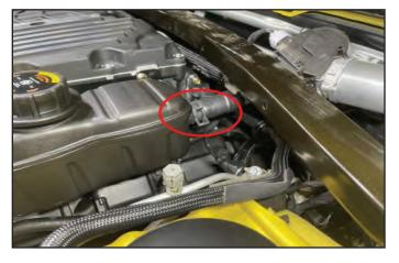
201. Install the factory throttle body using (4) M6X1.0X40mm long fasteners PN 71-06-10-040. Tighten the throttle body fasteners in a criss-cross pattern. Install the throttle body electrical connection and cycle the lock on the connector.
