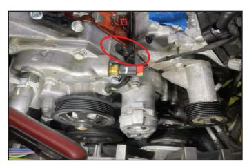
148. Remove the nut holding the factory knock sensor to the stud on the back of the LH cylinder head. Remove the stud holding the back of the heater tube onto the LH cylinder head.
