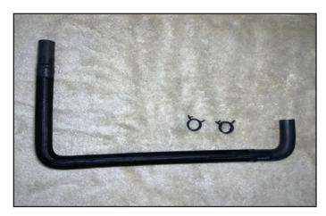
184. Apply Lubriplate to the PCV fitting on the RH side of the supercharger then install the hose from the last step to the PCV and secure it with the constant tension clamp as shown.
