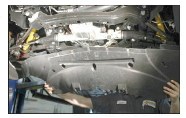
30. Pull up on the two halves of the radiator cover to unsnap them from their mounting holes and set aside for later re-installation.
