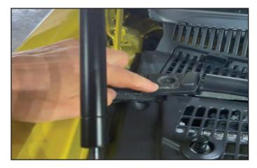
10. Remove the right hand side cowl access panel by lifting up on the tab.
