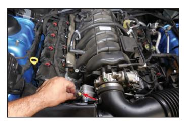
52. Remove the mounting bolt for the air box shown with the green arrow, and the hose clamp on the intake air tube at the yellow arrow location using an 8mm wrench. Remove the intake air tube and air box from the vehicle, set aside for some parts that will be reused later.
