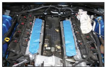
67. Use a 16mm wrench to remove the air box extension support bracket if applicable. Not required on 6.4L vehicles.
