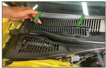
11. Remove the left hand side cowl panel access panel by lifting up on the tab at the arrow.
