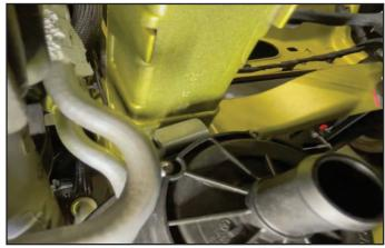
101. Select the hose clamp PN 48-46-10-009 from the kit. Install the clamp around the intercooler pump body and over the mounting bracket as shown. Tighten the clamp to secure the pump to the bracket in the orientation as shown.
