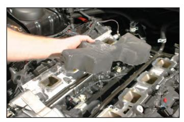
64. Use a vacuum to remove any debris from the heads and adjacent surfaces. Be careful to not allow any debris into the open ports.
