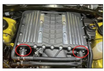
200. Route the opposite end of the hose around the back of the supercharger, over to the fitting on the back of the coolant reservoir. Select a 3/4" constant tension clamp, install it over the hose then install the hose onto the fitting at the back of the reservoir.
