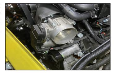
202. Install the new clean air tube onto the throttle body. Install the air box back into the vehicle and re-secure it using the factory bolts. Secure the clean air tube to the throttle body and air box using the provided constant tension clamps.
