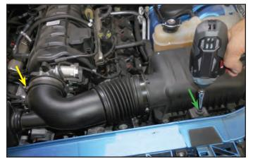
53. Unplug the Electronic Throttle Control (ETC) from the throttle body. Pull back on the white locking tab first before you unplug this connector.
