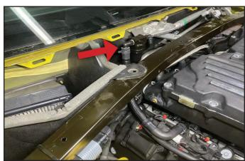
187. Select the hose that was cut in the previous step. Tape back the protective sleeve as shown, then install a 21 mm constant tension clamp to the short hose end. Install a straight hose mender PN 48-46-00-060 onto the short end of the hose. Secure the mender using a 21mm constant tension clamp.
