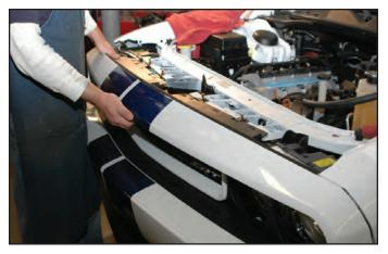
38. Remove the three push pin rivets holding the plastic bumper section to the sub frame. (2 locations shown)
