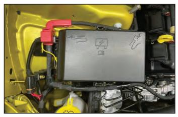
117. Install the I/C pump to LTR hose in the orientation and locations shown. Secure the hose to the tube at the LTR using a 3/4" constant tension clamp.
