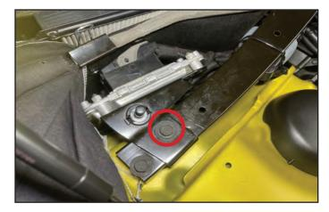
210. Tape up the factory CMCV connector with electrical tape.
