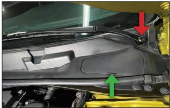
213. Re-install the LH and RH foam rubber trim pieces into each side of the cowl (LH side shown, RH side similar).
