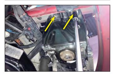
72. Place the two provided dowels in two of the existing crank pulley ring holes.
