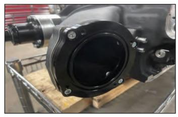
139. Remove the stock throttle body from the factory intake. Harvest the factory throttle body gasket from the intake and install it onto the inlet adaptor on the supercharger.
