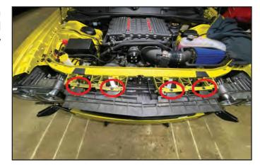
218. Re-install the front fascia, reversing the steps outlined at the beginning of the manual for removal.
