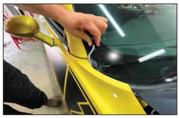
9. Remove the fir tree connector securing the rubber hood isolators on both sides of the cowl.
