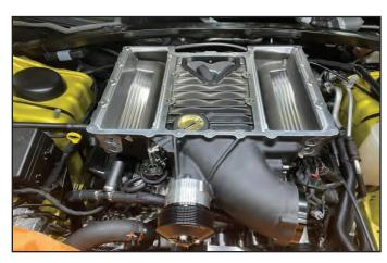
168. Install (10) M6X1.0X40mm long fasteners into the supercharger mounting locations. Hand-start and zero-torque all fasteners in a criss-cross pattern starting from the center out. Pre-torque all 10 fasteners to 53 in-lbs in sequence. Final torque all 10 fasteners to 106 in-lbs in sequence.
