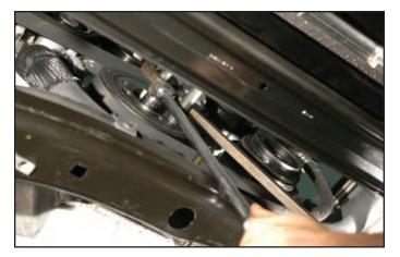
74. Install the crank pin drill guide with the provided bolt and a 22mm wrench. It's convenient to align the two holes for the crank pins in the drill guide horizontally for ease of access. Torque the temporary bolt holding the drill guide to 40 ft-lbs.
