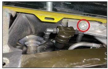
181. Install 3/8" bulk hose (highlighted in green) onto the rear-facing port of the oil fill adaptor. Fully seat the hose over the barb. Route the hose around the back of the supercharger toward the right-hand rear corner of the engine bay.
