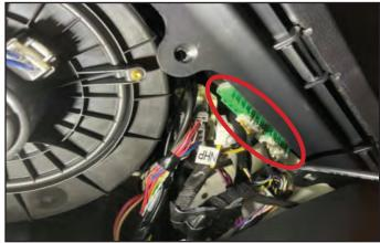
21. If you prefer to leave the security bypass cable (highlighted in green) permanently installed, route the other end under the dash and over to the factory OBDII port in the driver's foot well. Plug the cable into the OBDII port ensuring it is fully seated. Follow the instructions to program the PCM using the hand-held device after the supercharger kit has been installed.
