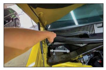
14. Remove the fastener securing the PCM to the vehicle at the red circle.
