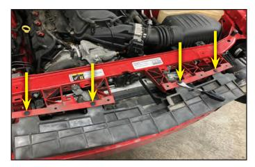
42. Disconnect and remove the ambient air temperature sensor harness from the closeout panel.
