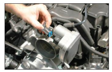
54. Unplug the eight fuel injector connections. You will need to pull out on the red locking tab to disengage it first. Then you can push on the black side button as you pull it out.
