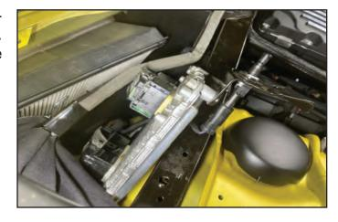
209. Secure the PCM bracket to the cowl using the factory bolt.
