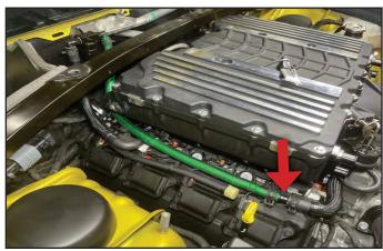
191. Install the CAC hoses to the LOWER charge air cooler ports on the supercharger. Secure the hoses using 3/4" constant tension clamps.
