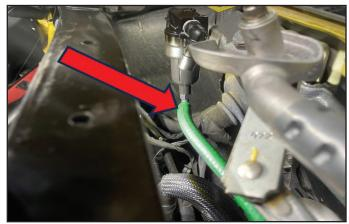
183. Select the hose shown from the kit. Install a 21mm constant tension clamp to the end shown.
