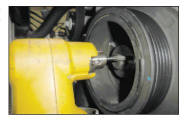
78. When you're finished with the ream bit, blow the holes out again with compressed air watching out for your eyes.
