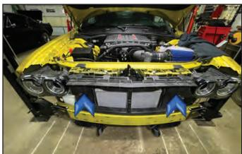
217. Note: ensure the panels do not pinch off the low temp radiator hoses. The panel ends may have to be trimmed to allow clearance.
