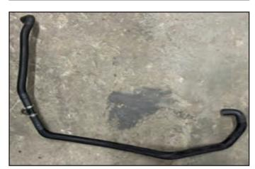
120. Pre-install the hose (highlighted in green) from the last step to the vehicle as shown. The hooked end of the hose routes down between the alternator and the inside of the frame rail, toward the connection point at the RH side of the low temp radiator.
