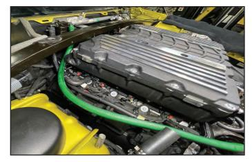
190. Route the hose (highlighted in green) from the oil separator, under the cowl, then along the RH side of the supercharger. Cut the hose to length and attach it to the straight mender (arrow location) on the hose installed in the previous step, securing it with a 21mm constant tension clamp.
