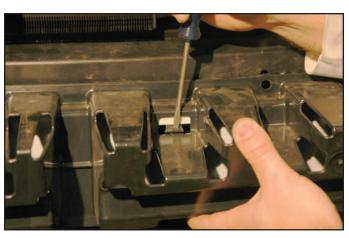
40. Once the clips are released, pull the plastic bumper section free and set aside for installation later.
