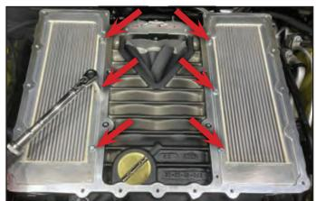
127. Remove (6) turret fasteners from the front securing the turrets to the base. Three fastener locations are shown here.
