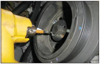
76. Blow out the holes using compressed air. Use safety glasses and be careful of your eyes!
