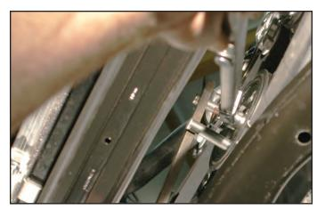
84. Re-install the OEM fan shroud assembly in the vehicle. We found this a little easier from below the vehicle.
