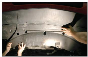
27. Remove the 2 T15 Torx (or 8mm hex) bolts from the front splitter (One per side).
