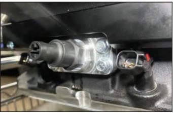
137. If you are installing a boost gauge, there is a spare 1/8" NPT plug on the RH rear corner of the supercharger for this provision.
