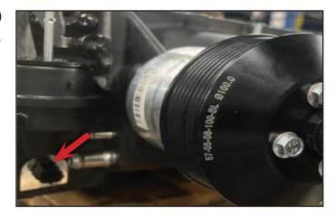
130. Secure the sensor to the intake using an M5 X 0.8 X 10mm long fastener P/N 71-05-08-010. Torque to 70 in-lbs.
