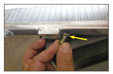
90. The two locations for the carriage bolts are shown here at the arrow locations.
