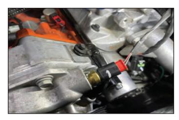
156. Re-install the stud through the heater tube bracket and into the back of the LH cylinder head. Torque the stud 18 ft-lbs.
