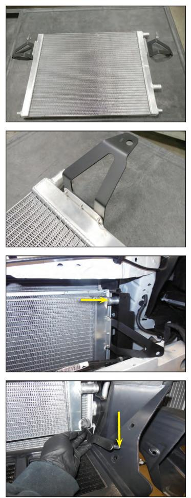
193. Loosely install the two provided nuts on the back side of the bracket just installed.
