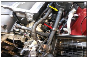
217. Apply a thin layer of Lubriplate grease to the inner rubber of the hose assembly shown. This will be used to connect the upper LTR spigot to the CACs.
