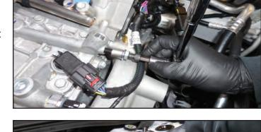
80. Once the Loctite has softened you can tighten the nut with a 9/16" wrench. This will pull the plug from the bore.
