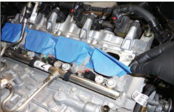
152. Install the provided seal washers shown with a blue arrow on 10 provided M6x35mm flange bolts. Once you have slid the washers on all the way to the heads apply a light coat of Lubriplate grease to their undersides. Finally apply blue Loctite 242 to the ends of these bolts as shown
