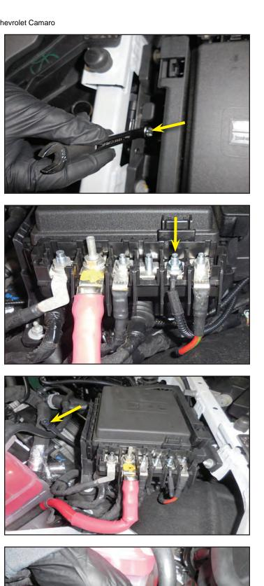
241. Secure the wire connection made in the last step to the hose shown with a cable tie. Trim off the excess cable tie once it has been secured.
