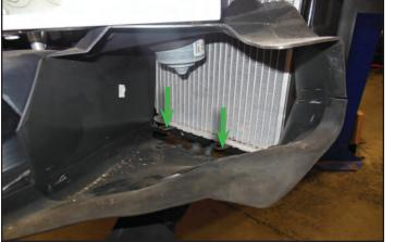
181. Remove the plastic rivet shown with an arrow. The brake air duct should now pivot out of the way.
