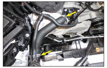
96. Plug both connection points for the hose that was removed in the last step with rags.
