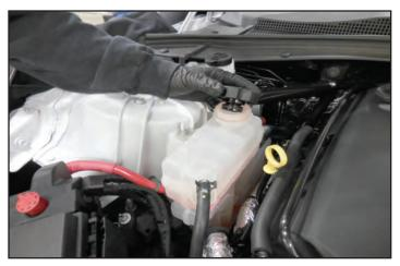
32. Place a clean drain pan under the radiator drain spigot located on the front right side of the vehicle. Loosen the valve shown with an arrow until the fluid begins to drain. Once the fluid has drained completely close the drain valve, and re-install the radiator reservoir cap. This will take about 15-20 minutes.
