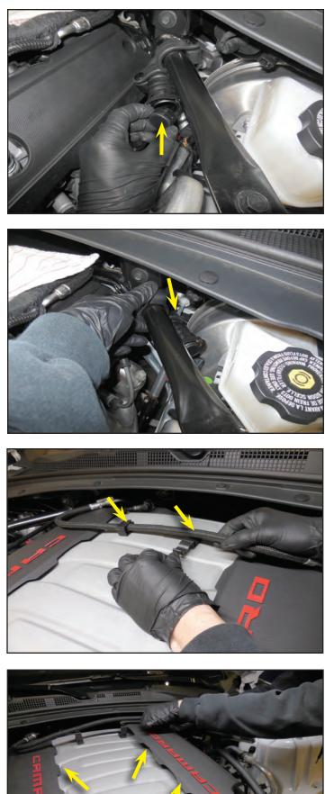
45. Rotate the resonator hose behind the brace.
