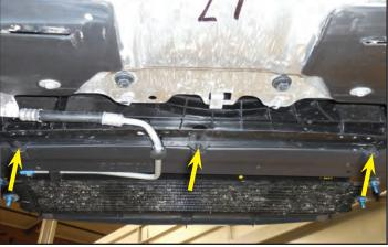
104. Disconnect the transmission cooler line from the clip shown with the yellow arrow.
