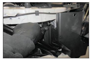
282. Connect the battery and tighten with 10 mm wrench.
