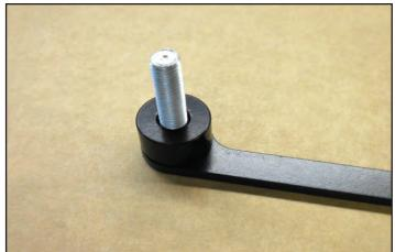
144. Install the coil covers with the supplied lower mount as shown using the provided nuts.
