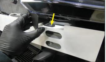
173. Remove the deflector that just had the plastic rivets removed.
