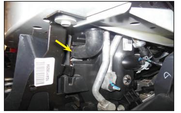
213. Connect the hose assembly end to the intercooler pump discharge using a provided spring clamp. First place the opened clamp over the hose then slip the hose/clamp over the pump spigot. Now re-install the upper radiator supports.
