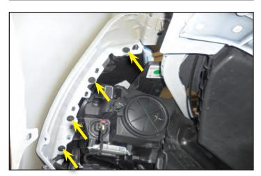
20. Disconnect the electrical plug shown with an arrow that is located in the right fender well.
