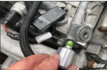
85. Apply a thin bead of the supplied green Loctite 680 to the outside of the supplied PCV relocation fitting in the location shown.
