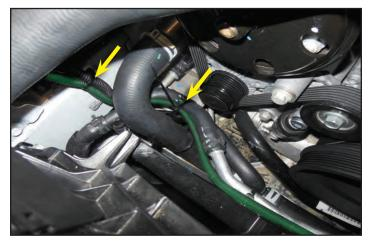
245. Route the power wire for the intercooler pump under the steel tube shown, and cable tie it to that same tube in the two locations shown with arrows.
