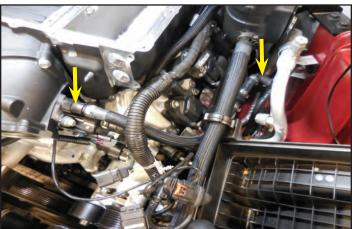
225. Remove the terminal cover on the back of the fuse box. There are two clips on either side of this cover that must be disengaged prior to removal.
