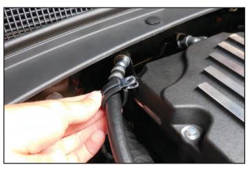
261. Install the last provided M6x20mm bolt in the corner lid location through the Adel clamp and washer that were just installed.
