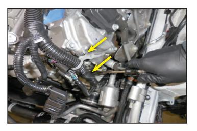
120. Torque the bolts with 15 mm heads to 25 ft-lbs, and the two bolts with 12 mm heads to 18 ft-lbs.
