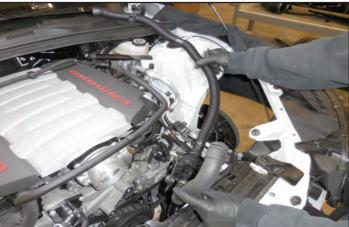
44. Install the provided plug into resonator hose connection shown.
