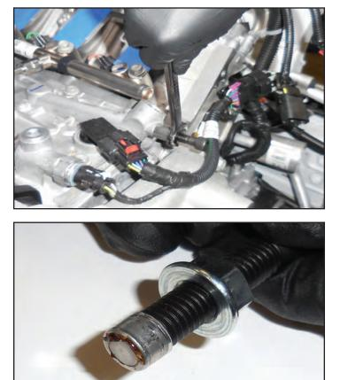
82. Clean the bore area where the plug was with a cotton swab. After the larger particles have been cleaned out use denatured alcohol, or acetone to clean out the bore thoroughly.
