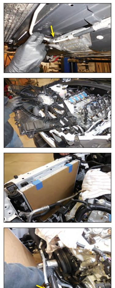
108. You may have to heat the bolt with a heat gun or torch to soften the locking chemicals prior to removal with the impact gun. Save this bolt for a later step.
