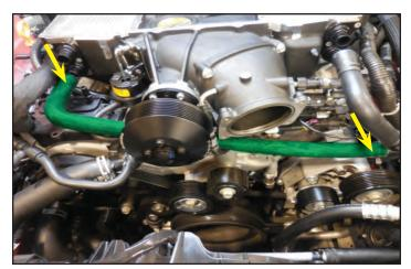
253. Use hose clamp pliers to install the spring clamp at the coolant manifold spigot.
