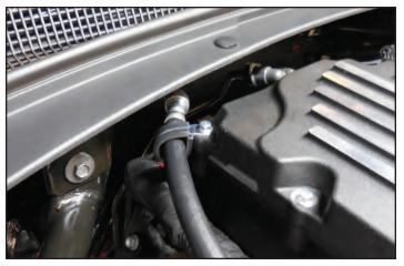
262. Zero torque the fasteners first before applying the final torque. Torque these 23 bolts to 106in-lbs following the order for the lid given at the back of this manual.
