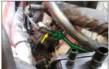
161. Route the longer wire from the last step to the opposite side of the engine routing it under the throttle body adapter as shown with the green dashed line. The shorter wire will run in the opposite direction towards the fuse box. Both of these connections will be plugged in later.
