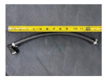
168. Connect the other end of the provided PCV hose from the last step to the 90 degree hose barb shown and firmly secure using the provided Oetiker clamp and provided pliers. The provide pliers are smaller than the ones pictured.
