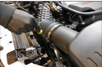
36. Unplug the connection from the MAF sensor by first pulling back on the red release lock located on the underside of the connector.
