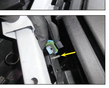
237. Tighten the fuse cover in place with a provided nut.
