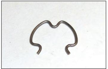
100. Once the spring clip is removed from the hose you can pull the hose out. Carefully clean the port out with a clean towel and plug the port to prevent any debris from entering. Also cap the hose to prevent any leakage. You can now disengage the hardline from the fan shroud.
