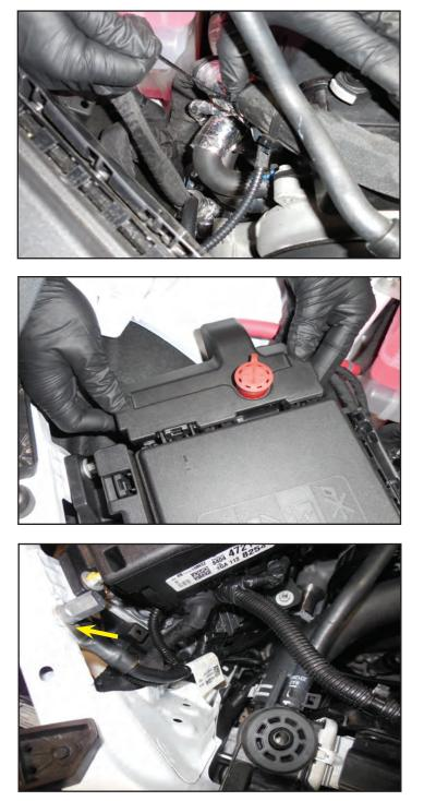
242. Reinstall the terminal cover on the fuse box.
