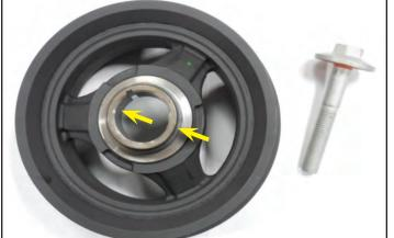
112. Apply motor oil to the crank seal.
