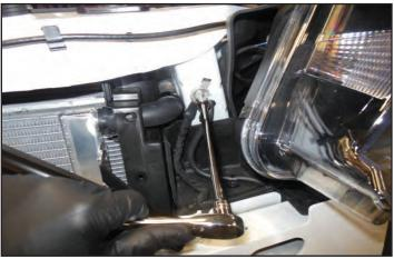
281. Trim the upper plastic rivet shown down by .25" for clearance, and then reinstall the panel shown. Also re-install the left brake duct at this time using the three plastic rivets that were removed.
