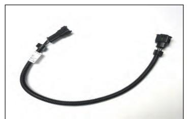
157. Install the MAP sensor wiring extension on the OEM plug.
