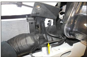
177. Remove the three plastic rivets shown with the arrows. One is hidden behind the pump (shown with a dashed arrow). The rivets shown with the red arrows may be easier to remove from the back side which is shown in the next step.
