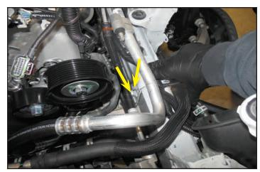
205. Install the provided bracket as seen here using the two OEM bolts that were removed in the previous step. The bracket is normally black but has been highlighted in green for clarity.
