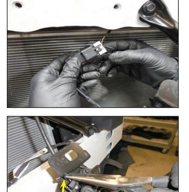
29. Use pliers to compress the plastic fitting holding the cable housing to the latch bracket. This will allow you to push the housing away from the bracket.
