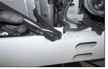
197. Cut the other electrical wire retainer located near the left and right angle brace on the bumper crash bar.
