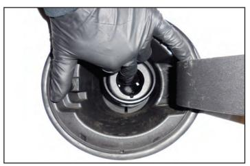
60. Place rags around the fuel line shown at the left side of the engine. Remove the metal locking clip from the fuel line.
