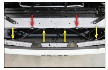
18. Loosen the bolt on the opposite side of the long diagonal brace from the last photo. Use a 15mm closed end rachet wrench if available to loosen 1/4 to 1/2 turn. You do not need to remove this bolt. The passenger side bolt is below the horns at the red arrow location.
