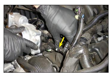
60. Remove the EVAP solenoid electrical connection by pressing the release tab and unplugging.
