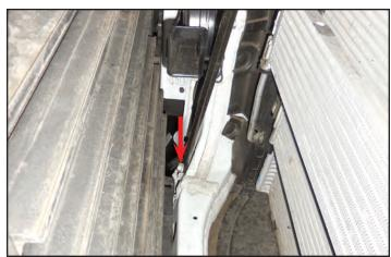
19. Once loosened, pivot the brace inward and down until it touches the back of the shutters. Here you can see the passenger side long diagonal brace moved out of the way. Repeat this process on the driver side long diagonal brace. This will give the necessary room to install the Low Temperature Radiator (LTR) for the intercooler system.
