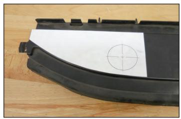
36. Use an electric drill with a hole saw to drill out the 1.75" diameter hole. Debur the hole after drilling.
