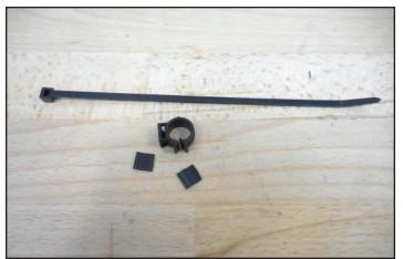
94. Install the cable tie with the clip from the last step around the mesh on the upper radiator hose in the same location the OEM clip was and secure the smaller hose to it.
