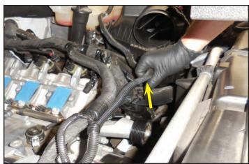
79. Remove the fastener holding the upper radiator hose at the arrow location. Try not to damage this plastic tie because it will be reused.
