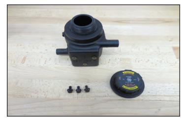
119. Install the cap on the reservoir, and secure in place with the three M6x12mm bolts by hand.
