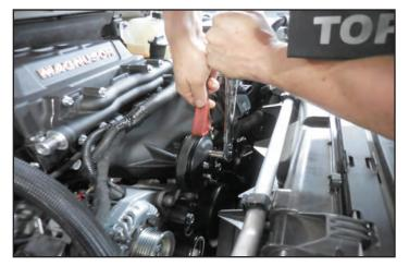
194. Install the belt following the diagram at the back of this manual. Connect a belt tensioner wrench or 1/2" breaker bar at the tensioner and rotate it counter-clockwise. The last pulley to place the belt over should be the smooth pulley that was installed on the right side three steps ago.
