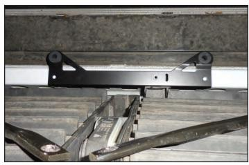
31. Reinstall the OEM center bracket that was removed earlier.
