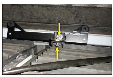
32. Raise the vehicle and remove the plastic cover shown by pinching at three areas, and pulling down. Two of the areas are shown here with pairs of arrows.
