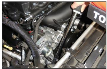
190. Gather the two provided idler pulleys shown along with the two M10x30mm bolts. Apply blue Loctite 242 to the bolts. Ensure that the side with the bearing surface and clip shown below is facing towards the engine when installed.
