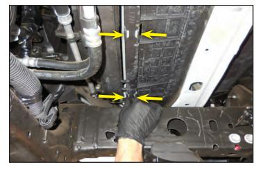
33. Release the tab on the passenger side shown for the cover from the last step.
