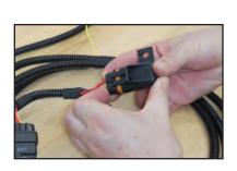
124. Remove the tape from the positive terminal side and remove one inch of the slit loom as shown.
