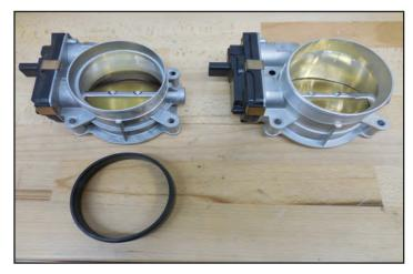
220. For this kit we are using the stock 87mm throttle body. You will place this adaptor over the 87mm throttle body in the orientation shown with the large external chamfer (arrow location) facing up.
