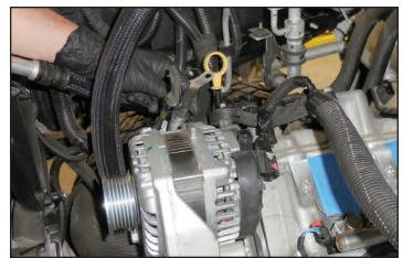
98. Remove the alternator bolt shown at the arrow using a 15mm socket wrench.
