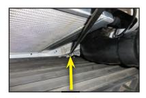
273. Reconnect the two small diagonal braces as shown here. Sandwich the LTR behind the two braces, you may need to pull up on the LTR again to align them.
