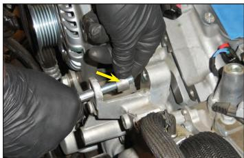
104. Gather the OE alternator bolt shown below along with the bushing that was removed in the last step. Insert the bushing into the provided bracket and tighten it in place with the bolt. See the next step for the bushing depth.
