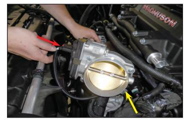
234. Remove the tabs from another cable tie clip shown below. Install the clip on the ETC cable and secure it to the arrow location.
