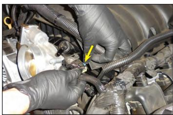
59. Press the release button on the EVAP hose connector and unplug it from the EVAP solenoid.
