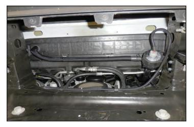
159. Use two cable ties (highlighted in green) to secure the slack of the wire harness that goes to the intercooler pump in the passenger fender well, behind the headlight bucket.
