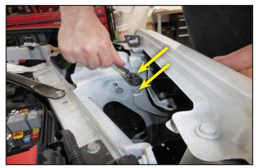
128. Place the intercooler electrical harness bracket in the location from the last step using the two OEM bolts that were just removed.
