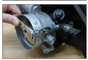
209. Gather the EVAP solenoid that you just removed and the provided M6x25mm bolt shown. Apply blue Loctite 242 to the bolt before installation.
