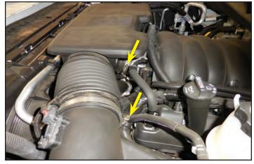
53. Rotate the air intake plenum as shown to reveal the final mounting location.
