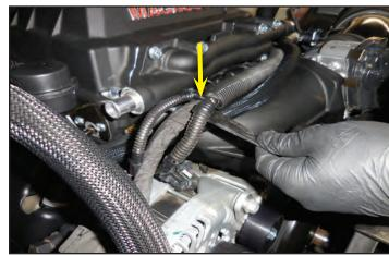
228. Cut 10 inches of 3/4" slit loom and install it at the arrow location.
