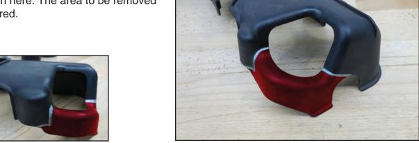
205. Trim the driver's side coil cover at the lines that were made in the last step.
