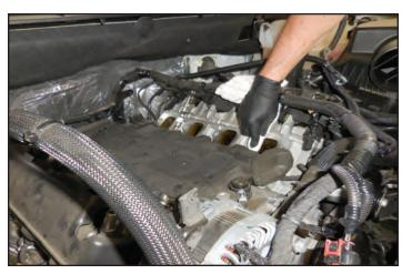
72. Seal the intake ports with tape (Shown here in blue).
