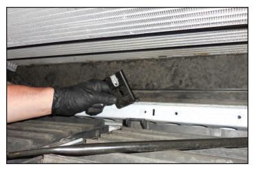
22. Clean the lower cross brace shown here in white with a cleaning product like Simple Green followed by rubbing alcohol to prepare it for the provided lower LTR bracket.
