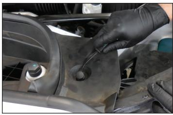
11. Remove the two T15 Torx bolts that hold the hood lever, and remove the lever.
