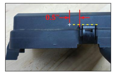
139. Use a center punch to indent the cross location from the last step. Use a 1/8" drill to start the hole location.
