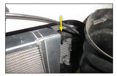
255. Attach the opposite end of the hose from the last step onto the inlet of the supercharger charge air cooler pipe at the arrow location.
