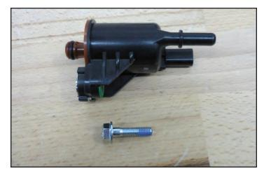
210. Install the EVAP solenoid in the location shown with the arrow using the provided M6x25mm bolt from the last step.
