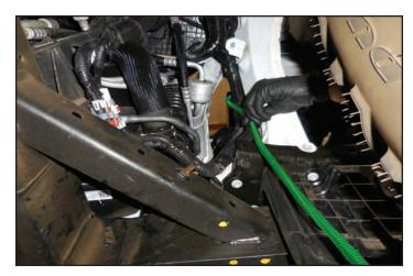
149. Route the end of the cable with the gray connector above the electrical harness shown at the arrow.
