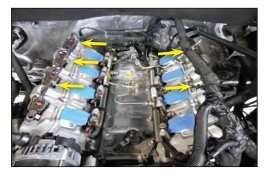
76. Unplug the top connection to all eight coil packs. Four coil packs are shown with arrows. Pull the red locking tab prior to unplugging.
