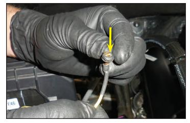
142. Slide the provided grommet from the last step over the yellow trigger wire just above the tape that was added in a previous step at the arrow.
