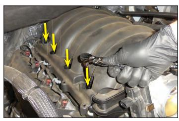
68. Be careful when pulling the manifold forward because the bolts can scratch the cylinder heads. Pull the intake manifold forward a bit to gain access to the wiring harness "tree" anchors that hold the harness to the back of the intake manifold. Use a screwdriver or tree clamp remover to unplug these trees from the OEM intake manifold.
