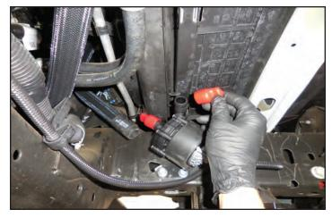
154. Attach the hose from the reservoir at the intercooler pump inlet yellow arrow location and secure with a provided spring clamp. Attach the hose that comes from the lower LTR inlet pipe to the output of the intercooler pump at the red arrow and secure with a provided spring clamp.
