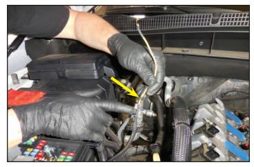
143. Route the yellow trigger wire though the hole that was made in the fuse box cover. Make sure the grommet is fully seated on both sides.
