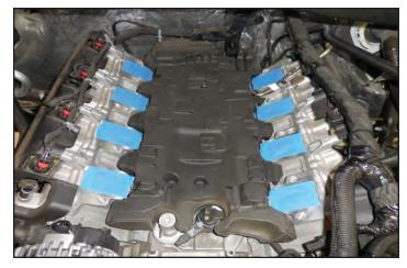
73. Remove the insulation pad from the engine valley. This will not be reused.
