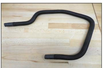
260. Route the hose from the last step as shown here. This hose will go around the air box.
