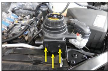
120. Gather the hose assembly shown below. This will be installed on the lower output pipe on the reservoir. Guide the hose (highlighted in green) behind the upper radiator hose at the arrow.
