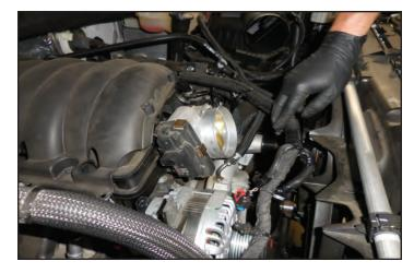
66. Remove the cable tie fasteners from the arrow locations. Repeat this process on the opposite side of the intake manifold.
