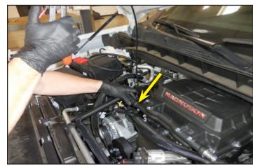
256. Here is a close-up of the inlet pipe hose connection to the supercharger charge air cooler.
