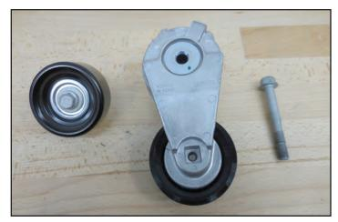
107. Apply blue Loctite 242 to the threads of the pre-installed bolt on the idler.
