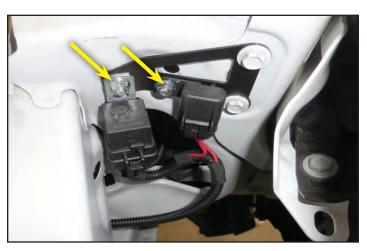
133. Route the red positive wire, and yellow trigger wire under the fuse box.
