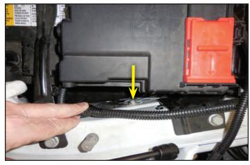
136. Route the ground wire for the intercooler pump harness as shown highlighted in green towards the bolt location from the last step.
