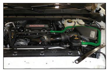
263. Secure the opposite end of the hose to the reservoir with a worm gear clamp. A worm gear clamp is necessary for proper sealing at the reservoir.
