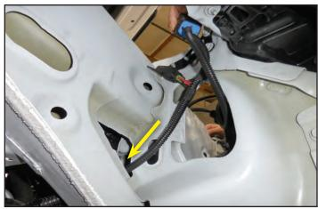
132. Secure the relay and fuse holder to the bracket with the provided serrated flange nuts.
