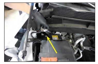
6. Ensure that the engine is cool before proceeding. Remove the radiator cap to help the coolant drain faster in the following steps.
