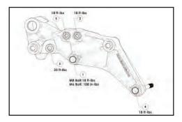
188. Rotate the alternator into the new idler bracket and insert the stock bolt.
