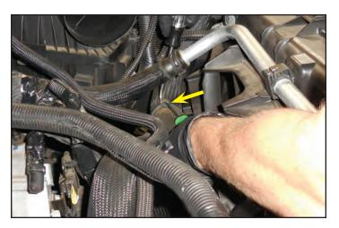
80. Cut the cable tie shown at the arrow. This will be replaced with a new one.
