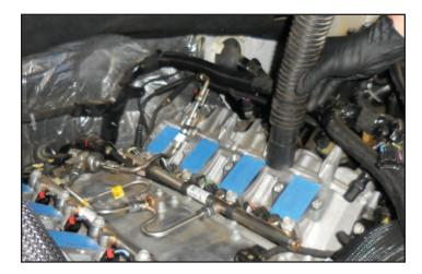
173. Remove the tape from the intake ports and vacuum them out to remove any debris.
