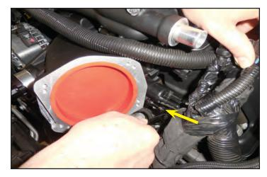
211. Plug in the electrical connection for the EVAP solenoid at the yellow arrow location. Ensure that you have secured the locking tabs on both fittings. The location where you can install a MAP sensor is circled here. No MAP sensor is provided.
