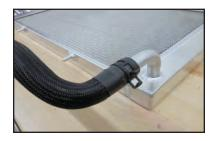
42. Insert the LTR in front of the radiator with the lower inlet pipe facing down and to the passenger side as shown with the arrow. At the same time have someone help you run the hose from the last step through the hole you made in the lower radiator panel earlier.
