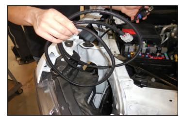
131. Run the other length of wire with the in-line fuse through the triangular hole shown with the arrow. This will be fed under the fuse box.
