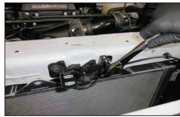
272. Reconnect the two large diagonal braces shown here with a 15mm socket wrench. Torque the two upper bolts to 25 ft-lbs and hand tighten the two lower bolts (one is shown below with the arrow.)
