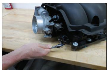
208. Remove the four bolts holding the throttle body to the OEM manifold. You may be using your OEM throttle body depending on how your calibration is being handled. These bolts will not be reused. If you have a 5.3L engine you will need to purchase a throttle body (GM Part# 12678223).
