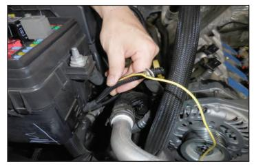
134. Place the red positive wire's eyelet terminal over the main supply nut and secure with a provided serrated flange nut. Once the nut is tight, gently press down on the eyelet until it stops on the eyelet underneath.
