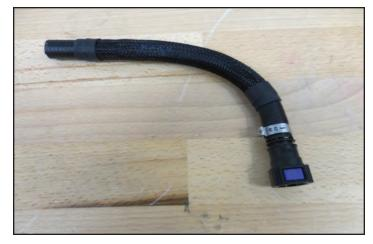
214. Preinstall the provided spring clamp shown below on the side of the hose from the last step without the fitting and secure that end on the supercharger at the arrow location.
