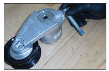
110. Once you have installed the bolt from the last step you will see the boss at the back of the tensioner shown with the arrow.
