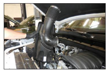
54. Pull the air intake plenum to the passenger side to remove it from the vehicle. This will not be reused.
