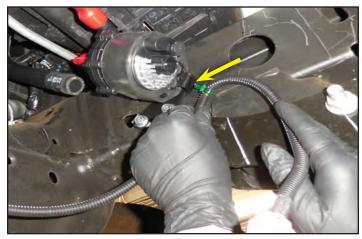
152. Hook the intercooler pump wire loom onto the two OEM connections shown with arrows if they are present. If these hooks are not present use some provided cable ties to secure this cable.
