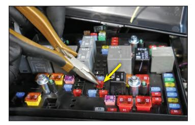
145. Install the "#47 TCM IGN" fuse on the metal terminal at the end of the yellow trigger wire.
