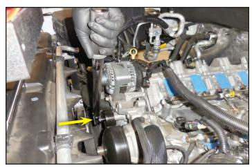
109. Apply blue Loctite 242 to the M10x80mm bolt and install it into the provided tensioner.
