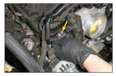
62. Unplug the alternator electrical connection shown with the arrow.
