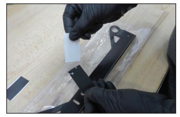
26. Place the double sided adhesive strip in the location shown highlighted in green. Repeat this installation process on the opposite side.
