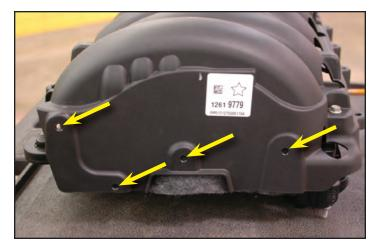
70. Carefully remove the intake manifold from the engine bay. Be careful not to drag the bolts across the sealing surfaces.
