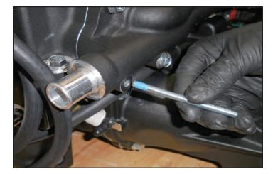
163. Ensure that 18mm of thread is protruding.
