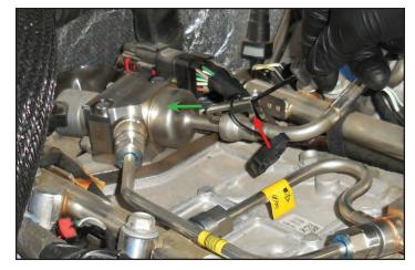
170. Reinstall the securing clip ensuring that it is now oriented to the side as shown with the arrow. This will allow the necessary clearance for the supercharger.
