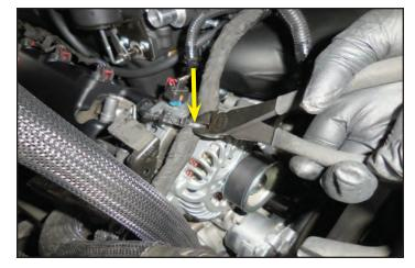
226. Install the power wire back onto the alternator and retighten the nut with a 17mm socket wrench.
