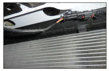
14. Disconnect the electrical connection for the hood release and at the same time remove the anchor holding the connector to the frame.
