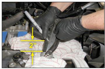
83. Release the clamp at the hose connection and pull the hose off.
