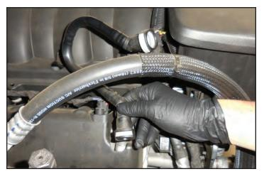
52. Using a 7mm nut driver or a flat blade screwdriver, loosen the clamps at the two arrow locations.
