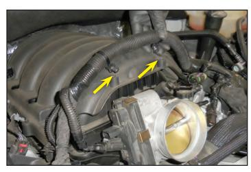
64. Remove the two cable tie fasteners shown with the arrows using a plastic pry bar.
