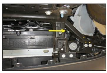
8. Attach a hose at the red arrow and loosen the drain plug at the yellow arrow. Drain the coolant into a clean pan as shown below so it can be reused if the coolant is still in good condition.
