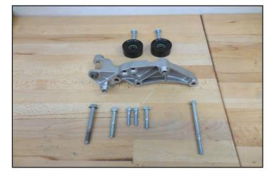
178. Lift the front of the supercharger to place the idler bracket from the last step into position. You will have to align the bracket down in the pocket the alternator used to sit in. Gently lower the supercharger back down and verify that the bracket moves freely.
