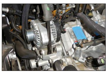
101. Remove the bolt at the water pump. The smaller photo below shows the location better with an arrow.
