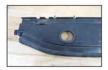
38. Reinstall the cover. Ensure that the tabs are lined up and the clips are locked in place.
