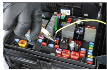
148. Route the end of the cable with the gray connector down from the top of the engine compartment as shown highlighted in green. This view is from under the vehicle on the passenger side with the wheel well cover removed. It is not necessary to remove the wheel well cover.
