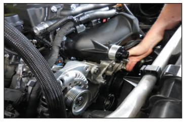
180. Gather the 8 provided M6x35mm bolts and apply blue Loctite 242 to the ends as shown. Gather the provided swivel socket shown below.
