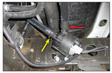
155. Remove the inner tabs from another cable tie with clip as shown below. Attach this clip at the tube shown and lightly secure the cable tie at the arrow location. The cable tie and clip are highlighted in green. Trim the excess cable away.
