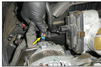
63. Remove the two cable tie fasteners shown with the arrows using a plastic pry bar.
