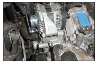
100. Use a prybar to lever the alternator up as shown.
