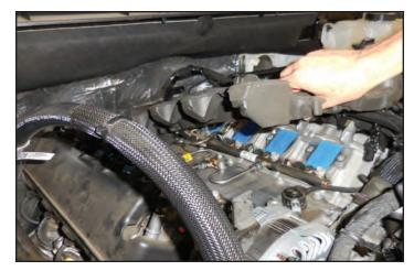
74. Remove the two plastic coil covers on the valve covers.
