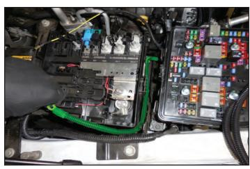
137. Place the ground wire eyelet from the intercooler harness on top of the OEM ground and reinstall the bolt from two steps ago.
