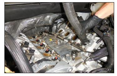
174. Use Simple Green or some other equivalent cleaner to wipe away any left over adhesive or debris. Apply some Tri-Flow or equivalent lubricant to a clean rag and wipe down the sealing surfaces.
