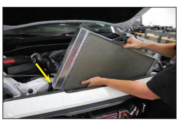
43. Here you can see the LTR hose installed through the radiator panel hole.
