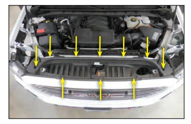
10. Remove the inner portion of the rivet first and then extract the outer portion.
