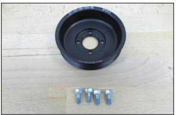
193. Use a strap wrench to hold the supercharger pulley in place while you torque it to 108 in-lbs using a 10mm socket wrench.
