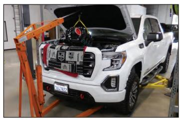
176. Ensure that the bolt holes on the supercharger line up with those on the heads. Make sure the electrical harness lays over the top of the supercharger inlet as shown. (Alternatively you can route the electrical harness under the supercharger for a cleaner look, but this will create more tension on these wires) Verify that the superchargers is fully seated on the heads and not hung up on anything.
