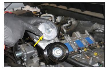
111. Line up the boss from the tensioner with the hole shown here at the red arrow in the photo below. The yellow arrow shows the location for the M10x80mm bolt. This is located below the alternator as shown in the photo to the right.
