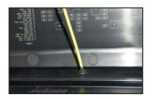
144. Remove the 10Amp fuse labeled as "#47 TCM IGN" at the location shown with the arrow.
