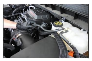
261. Install the hose from the last step at the supercharger charge air cooler outlet pipe with a provided hose clamp at the arrow location.
