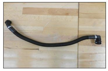
246. Install the hose assembly from the last step at the two arrow locations on the passenger valve cover and the air inlet duct. Ensure that the connections engage fully with a click. Gently pull on the connections to verify they are locked.
