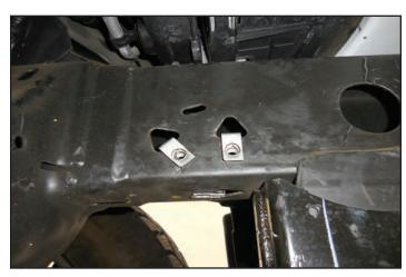
48. Mount the bracket with the two bolts as shown.
