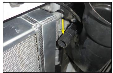
254. Attach the hose to the outlet pipe of the LTR at the arrow location with a provided spring clamp.
