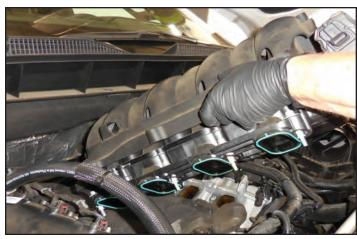
71. Clean the sealing surfaces on the heads using a cleaner like Simple Green.
