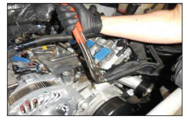
93. Gather the provided cable tie and clip shown. Remove the two tabs inside the clip.
