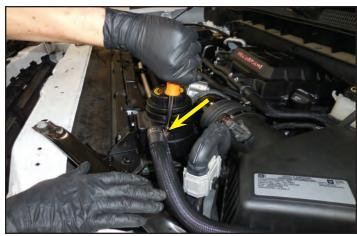
264. Gather the two clamps shown below. They will be used to connect the hose from the last step to a wiring harness behind the air box at the arrow locations.
