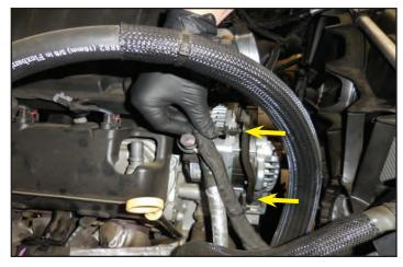
65. Pull the electrical wiring away from the throttle body to give room for intake manifold removal clearance.
