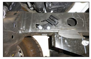
49. Install the pump in the rubber insulator with the orientation shown with the pump bolt location close to the rubber boss at the arrow.
