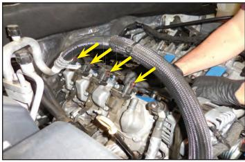
77. Unplug the spark plug wires for the back two coils on both sides of the engine. Mark the two rear coils on each side to ensure that they are installed in the original locations later. Remove the two bolts holding each of the two rear coil packs on both sides of the engine using a 10mm wrench.
