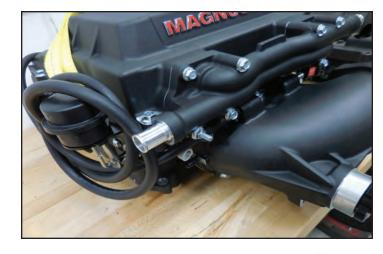
165. Remove the 8 intake manifold gaskets at the bottom of the intake manifold by first pulling at the tabs shown at the arrow locations. These will be installed on the supercharger housing. Replace any damaged gaskets with GM part# 12626354. Wipe the gaskets with a clean dry shop towel.
