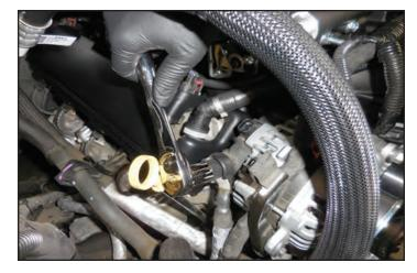
227. Unwrap the tape at the electrical harness junction shown.
