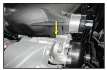
186. Gather the provided M8x40mm bolts shown below and apply blue Loctite 242 to the ends. Install these two bolts at the locations shown with arrows below the supercharger input shaft. You may need to loosen the other 3 slightly to get these to align.
