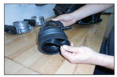
219. The rubber adaptor will be needed for the stock 87mm throttle body shown on the left. If you are running the 95mm LT5 throttle body shown on the right, you will not need the adapter.
