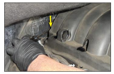
69. This image shows the location of the four tree connectors on the back of the intake manifold.
