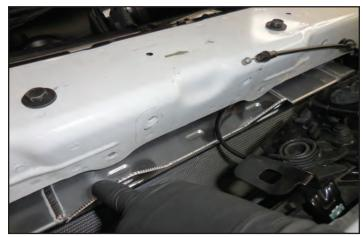
269. Reconnect the cable to the hood latch.
