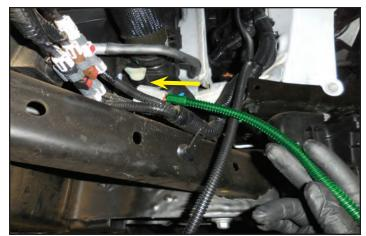
150. Route the gray connector over to the intercooler pump. Look at the next step to see how to attach a cable tie to the wire loom.
