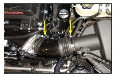
239. Consult the instructions for the supplemental device that connects to the MAF sensor. Do not connect the MAF sensor directly to the OEM connection.
