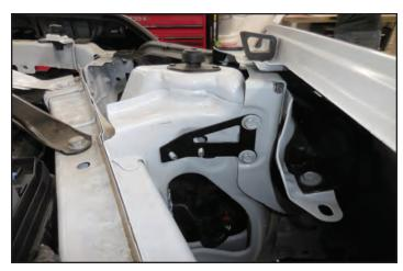
129. Run the gray plug from the intercooler pump harness through the opening shown with an arrow.
