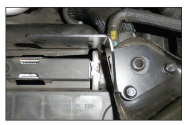
117. Torque the two M6x25mm bolts to 108in-lbs.
