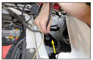
130. Continue to feed the gray plug and associated wiring through the hole in the last step until you have it near the headlight as shown.
