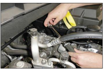
185. Ensure that the idler bracket sits flush with front of the supercharger at the arrow location.
