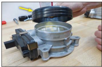
221. Here is the adaptor in its final location with the large chamfer facing up.
