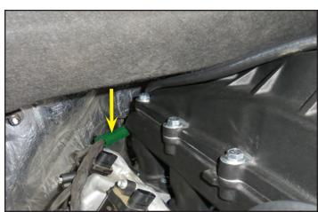
201. Plug in the electrical connections for all the coil packs on both sides.
