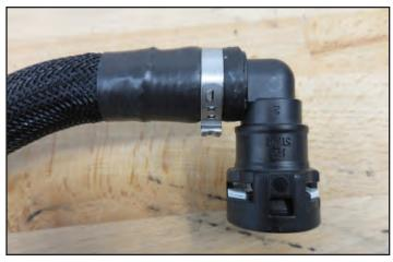
244. Secure the OEM 45 degree fitting on the opposite side as shown with another Oetiker clamp.
