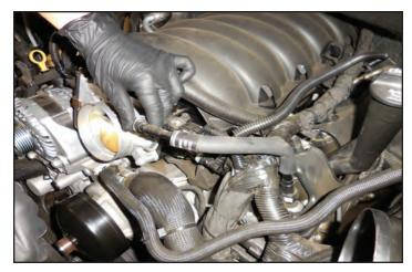
58. Release the blue locking tab, shown at the yellow arrow, on the MAP sensor electrical connection and unplug it.
