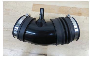
238. Install the air inlet duct between the throttle body and the airbox lid. Secure in place with the two hose clamps. Install first on the air box lid and then lower the lid/duct assembly down, sliding the duct onto the throttle body.
