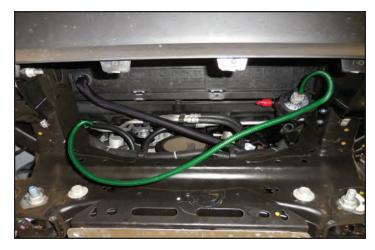
151. Ensure that there is enough slack to connect the cable from the previous step to the intercooler pump as you attach a provided cable tie with a tree connector on it (highlighted in green) at the location shown with the arrow here. This will provide a stress relief at the cable connection.
