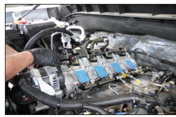
75. Remove the cable ties that are on the electrical harnesses. Several of these cable ties are shown below.
