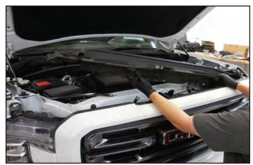
13. Locate the electrical connector for the hood latch shown that is on the underside of the cross support for the radiator.
