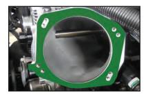
223. This photo shows the 95mm LT5 throttle body installed, but the stock 87mm throttle body will be used for this kit. Ensure that you apply blue Loctite 242 to the ends of the provided M6x40mm bolts as shown in the photo below.
