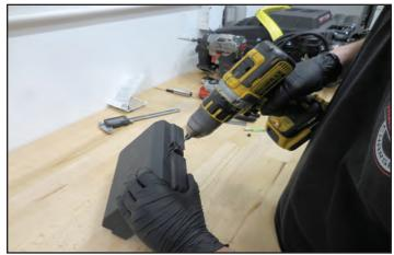
140. Use a step drill to open the hole up to 1/4" in diameter.
