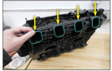
166. Install the 8 gaskets from the last step into the bottom of the supercharger as shown here. Ensure that the tab lines up with the notch in the top edge at the locations shown with yellow arrows.
