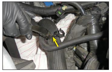
81. Pull the mesh away from the end of the hose connection. This will allow room for the hose to be cut. Also wrap the connection location with rags as shown to catch any coolant.
