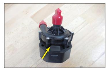
50. Install the rubber insulator on the bracket as shown. Ensure that it is fully engaged in the bracket.
