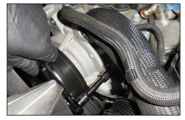
102. Use the provided bolt shown below to press out the bushing at the arrow.
