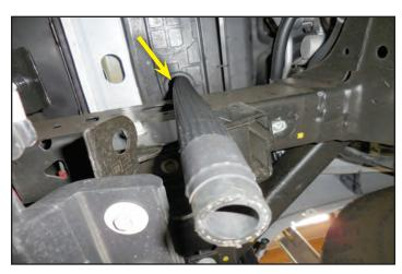
44. Line up the LTR using the marks that you made earlier with the holes in the bracket. This will allow you to line up the pins with the holes in the bracket. Verify the pins have aligned in the grommets by feel or with an inspection mirror.
