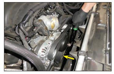
57. Remove the driver side PCV hose at the valve cover.
