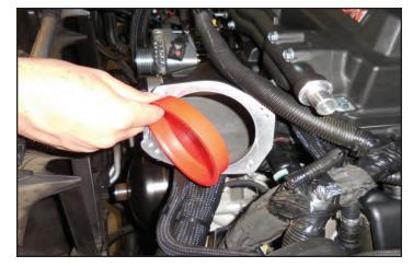
218. Remove the rubber adaptor from the end of the provided inlet duct.
