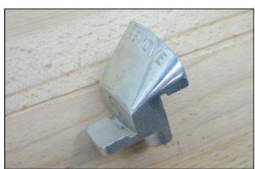
56. If using the tool shown in the last step you can rotate the crank with a 1/2 breaker bar and socket to allow the belt to ride up the ramp and derail itself.
