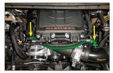
247. Secure the electrical harness to the PCV hose with a cable tie at the arrow location.
