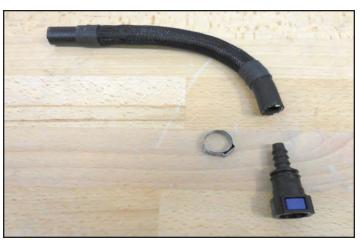
213. Slide the Oetiker clamp on the hose followed by the fitting. Use Oetiker clamp pliers to crimp the end of the clamp as shown.
