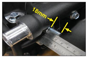
164. Install the provided M6 serrated flange nut on the stud and torque it to 108in-lbs.
