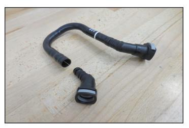
241. Gather the hose assembly, fittings and Oetiker clamps shown. The fitting on the left was removed earlier from the OEM PCV hose. The other items are provided.
