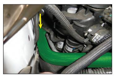
253. After the hose passes through the rubber shield it will be seen through the front like this.
