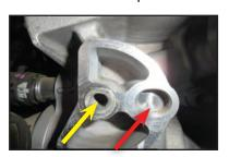
112. **Torque the tensioner to 25ft-lbs**. Make sure the boss stays properly aligned and tensioner is sitting flat before torquing.
