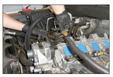
97. Remove the alternator positive cable terminal.
