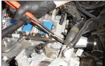
90. Reinstall the hose with the tabs for the clamp facing to the rear.
