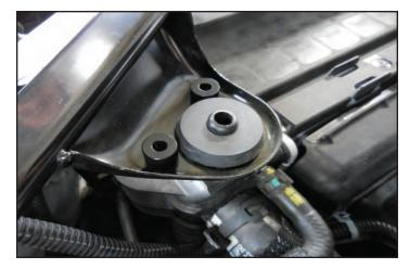
115. Place the bracket on top of the spacers, and install the two M6x25mm bolts from two steps ago through the top and secure them with the M6 serrated flange nuts from below. Use a 10mm socket wrench on top and a 10mm open end wrench on the bottom.
