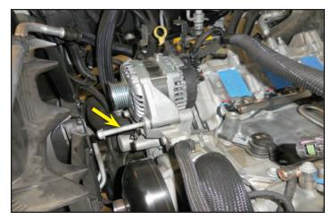
99. Loosen but do not remove the alternator mounting bolt on the opposite side with a 15mm socket wrench.
