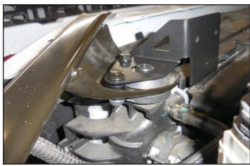
116. Ensure that the bracket is lined up with the radiator as shown.
