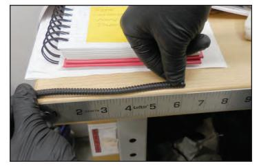
126. Peel back the yellow trigger wire through the OEM slit loom until it reaches the next tape junction. Cover the yellow wire with the wire loom from the last step and tape it in place at both ends. Continue the tape roughly 1" along the yellow wire.
