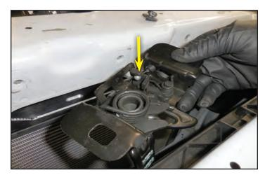
270. Plug in the electrical connector for the hood latch shown that is on the underside of the cross support for the radiator.
