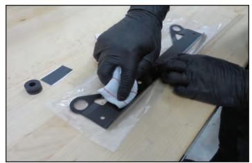
25. Peel the white cover off the double sided adhesive strip.
