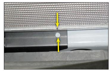
45. Temporarily install the OEM bolts loosely to maintain the LTR position while performing other operations. You will need to pull up on the LTR to align these bolts. The LTR is not designed to rest on the lower bracket. Double check on the grommet alignment.
