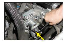
189. Torque the two alternator bolts shown in the last step with arrows to 25 ft-lbs.
