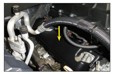
203. Route the vacuum line for the supercharger bypass behind the wiring for the coils as shown at the arrow.
