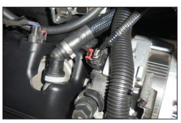
233. Gather the provided electronic throttle control (ETC) cable extension shown below. Route the cable end under the supercharger inlet at the yellow arrow. Plug it into the throttle body and engage the lock.
