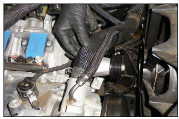
92. Rotate the clamp for the smaller hose so that the tabs face to the rear as you did with the other clamp.
