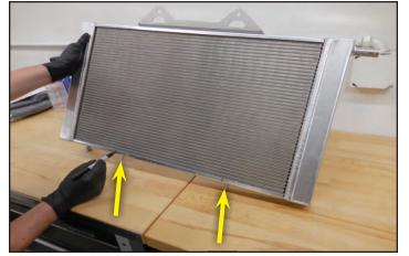
41. Install the hose assembly from the last step at the lower LTR inlet pipe and secure with the clamp from the last step.
