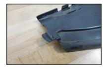
35. Use the template provided at the back of this manual to determine the location for the 1.75" diameter hole. Line up the template as shown here on the smooth underside of the passenger side. Use a center punch to transfer the hole location.
