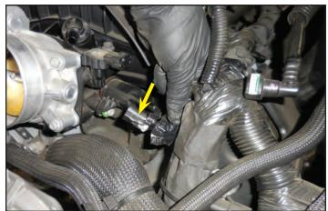
61. Disconnect the ETC connector from the throttle body. Depress the locking tab and pull the connector free.
