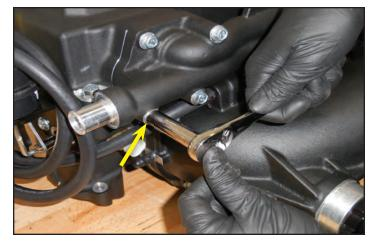
162. Apply some provided blue Loctite 242 to the stud from two steps ago as shown and install it at the location where the bolt was removed in the last step. It should thread in and bottom out by hand.
