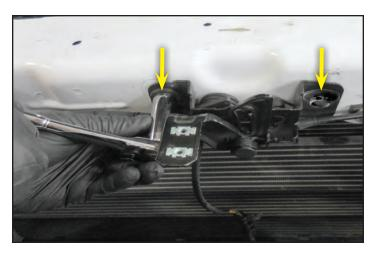
16. Disconnect the release cable from the hood latch.
