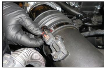
240. Gather the OEM PCV hose shown and carefully remove the fitting shown. Ensure that you do not cut into the barbed fitting when cutting through the plastic hose.
