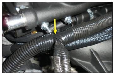
230. Install the provided cable tie with the M6 thread connection at the arrow location. Make sure the tie wrap does not pinch the wires at the junction.
