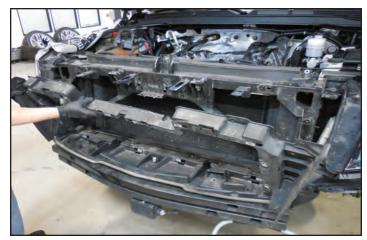
87. Remove the inner shroud shown. You will have to fold the plastic over at the lower passenger side corner to clear a metal support. You will be drilling holes in the passenger side of this shroud in the following steps.
