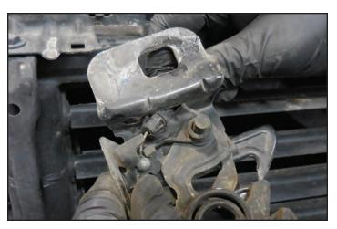
32. Use a 10mm wrench to remove 14 fasteners from perimeter of the louver assembly.
