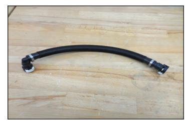
230. Install the hose from the last step between the driver's side valve cover and the inlet air tube. Ensure that you press the two white locking buttons. Pull at each connection to make sure locks are engaged.
