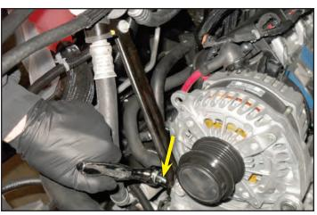
136. Pry alternator up to rotate it out of the way. This is done to gain clearance for the supercharger install.
