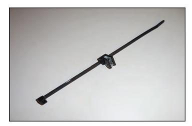
149. Remove the clip from the cable tie that was shown in the last photo and install it at the arrow location on the fan shroud.
