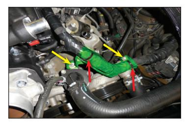
168. Remove the tape that wraps around the plastic ramp. Under this wrap is another cable tie that will need to be cut. After that the ramp shown below will be removed. This will not be reused.
