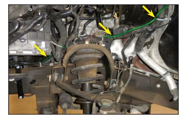
122. Plug in the electrical connection at the arrow location on the coolant pump. Adjust routing if necessary to gain slack at the connector.
