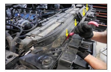
On both sides near the headlights you can see the backsides of the remaining 4 rivets (2 per side). You may have to cut these to remove them. Replacement rivets are provided for these locations. The front shroud will be removed in the next two steps to allow access to the other side of the rivet.
