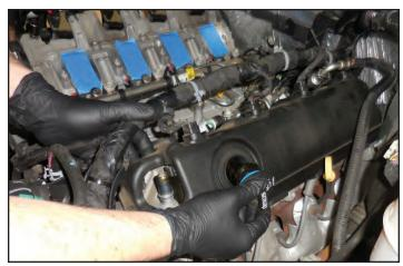
62. Remove the plastic coil cover and reinstall the oil filler cap. Remove the coil cover on the passenger side as well.
