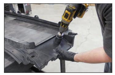
90. Install the two provided rubber grommets. Also cut the edge for hose clearance in the two arrow locations. Round the corners to eliminate any sharp edges.
