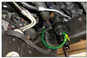
123. Route the intercooler pump ground wire (highlighted in green) above the brake booster housing. Remove the factory nut at the grounding location shown with the arrow using a 10mm socket wrench and place the eyelet from the coolant pump ground wire on the stud. Reinstall the nut to secure the two ground wires.
