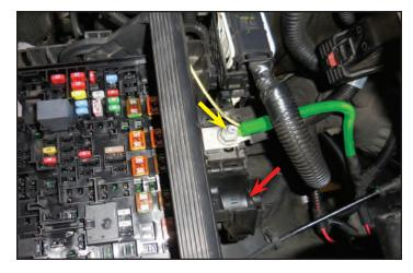
126. Create a notch at the green highlighted location shown with the arrow using side cutters and a file. This is where the yellow trigger wire will be located.
