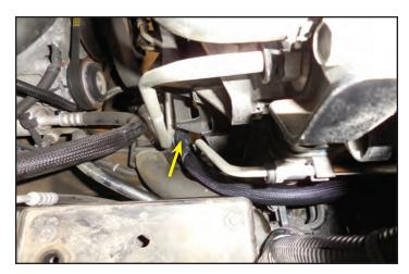
113. Continue to feed the hose from the last step (highlighted in green) over to the coolant pump and secure at the pump output with a provided spring clamp at the arrow location.
