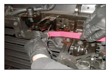
29. Mark the location of two hood latch fasteners to allow proper alignment during reinstall.
