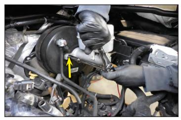
99. Replace the nuts incorporating the reservoir assembly. Torque to 25 ft-lbs. Verify your torque wrench settings.
