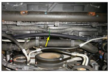
115. Install the provided 29" mesh over the provided 3/4" hose that is 27" long as shown.
