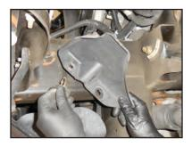
102. Remove the 6 mounting bolts for the rock guard, and remove the guard. Use a 15mm socket for the two bolts with red arrows, and a 10mm socket for the other four at the yellow arrows.
