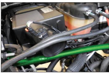
216. Slide the upper LTR hose onto the barb and secure in place with the pre-installed clamp at the arrow location.
