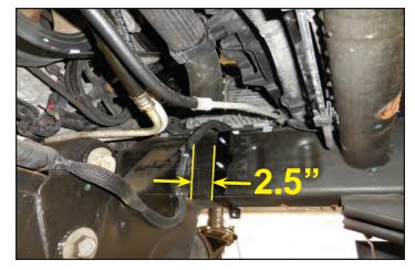
105. This image shows the opposite side of the frame rail from the last step. Apply Loctite 242 to the provided M6x20mm bolts and use them to attach the flat bracket from two steps to the bracket from the last step. Torque to 120 in-lbs.
