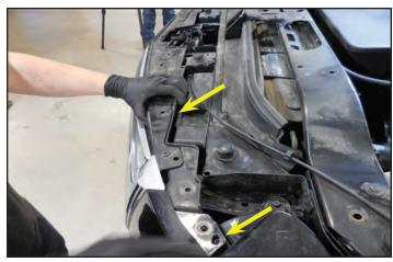
19. Remove the electrical connection for the front wiring harness. Unlock the rotating connector and pivot 90° to disengage.
