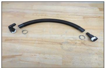
229. Pre-install the two hose clamps, followed by the two fittings. Next use Oetiker clamp pliers to secure the two clamps as shown.
