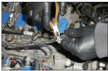
155. Ilf you have a 6.2L engine you will remove the four bolts holding the throttle body in place. These bolts will not be reused. If you have a 5.3L engine you will need to purchase a throttle body (GM Part# 12678223).
