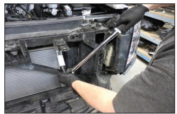
97. Hand tighten the supplied coolant reservoir onto the provided bracket with the three M6x12mm bolts using a 10mm socket wrench.
