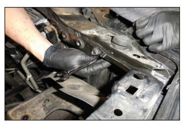
72. Remove the bolt for the window washer fluid tank near the lid and the one in the tray shown below. This will allow you to move the tank in order the access a radiator cross brace bolt using a 10mm socket wrench.
