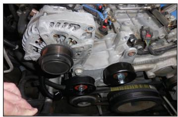
145. Loosen the factory spring clamp at the yellow arrow and rotate the hose clockwise as seen from the top (red arrow) from this connection then secure in place with the clamp. This will allow more clearance away from the belt line.
