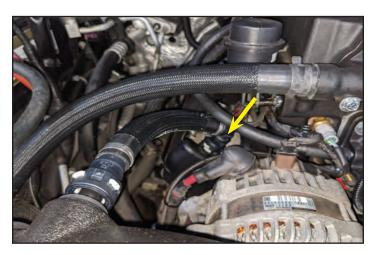
228. Gather the provided polyester mesh, hose clamps, fittings and 5/8" diameter hose. Cut the hose to 17 inch long. Install the provided 17 inch mesh over the hose.
