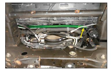
114. Install a provided cable tie (highlighted in green) at the arrow location around the wiring harness. Ensure that this is snug to avoid restriction on the hose. Trim the end off the cable tie.
