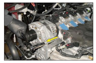
134. Loosen the other alternator support bolt shown. Do not fully remove the bolt.
