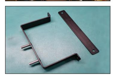
104. Install the bent bracket from the last step on the left inner frame rail with the studs towards the top. Orient the bracket 2.5" from the cross support as shown in the image.
