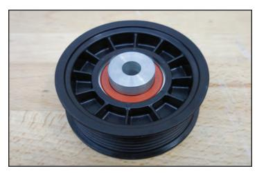
140. Apply Loctite 242 to the supplied bolt as shown below. Install the pulley with the spacer at the backside in the arrow location shown and torque to 25 ft-lbs.
