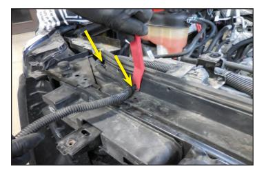
79. Pry the third harness anchor from the back side of the panel shown in the last step. Secure the electrical harness out of the way near the coolant reservoir as shown in the image below.
