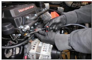
199. Plug the ETC wire extension from the last step into the throttle body and secure with the locking mechanism.
