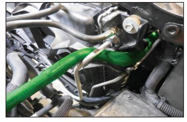
215. Route the hose from the last step under the air box tube as shown highlighted in green.
