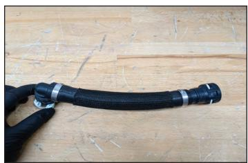
227. Install the 90° fitting of the hose assembly from the last step onto the passenger side valve cover and press the white locking button. Connect the straight fitting from the hose assembly in the last step onto the inlet air tube where shown and press the white locking button. Pull at each connection to make sure the locks are engaged.
