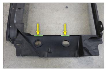
91. Reinstall the shroud and secure it with the plastic rivets.
