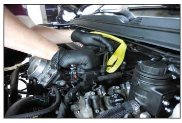
175. Apply Loctite 242 to the 4 lid bolts from the last step. Reinstall the bolts in their original location and torque them to 18ft-lbs.
