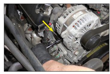
43. Here is the bracket removed in the last step. This bracket and the bolt will not be reused.
