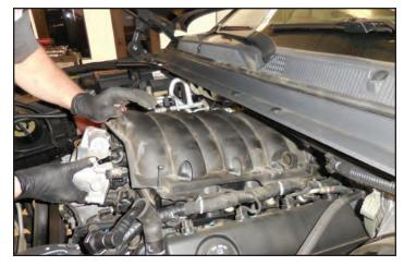
57. Carefully wipe down the sealing surface around the intake ports with Simple Green or equivalent cleaner. Make sure to not allow any debris to enter the ports.
