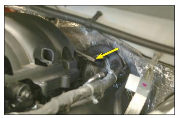
55. This image shows the location of the four tree connectors on the back of the intake manifold.
