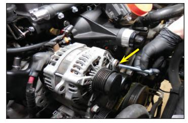
189. Torque the two alternator bolts shown with arrows to 25 ft-lbs.
