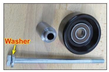
142. Insert the bearing in the spacer as shown.
