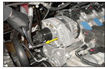
135. If you have the bracket located next to the alternator remove it. This bracket will be reattached later.
