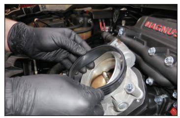
223. Install the intake tube between the airbox and the throttle body. Passenger side barb should point straight backwards.
