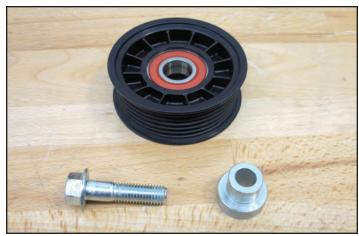
139. Insert the spacer into the bearing as shown.
