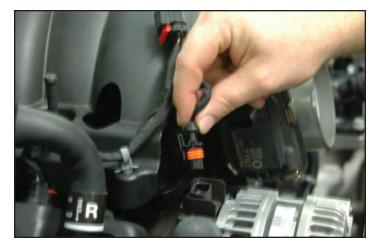
46. Pull the four "tree" tab wire loom mounting anchors from the holes in the right, and left side of the intake manifold.
