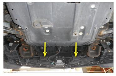
17. Carefully pull out on the side lower fender connection to ensure it is free. The plastic piece that was loosened in step 14 may come completely off.
