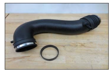
222. If you are using the stock 6.2L throttle body you will need to install the adapter shown. There is a lip on the inside diameter that faces out. The lip is also tapered on the outside.
