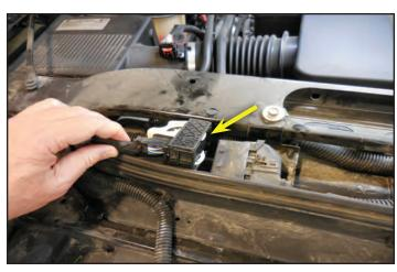
20. Use a plastic pry bar to remove cable ties shown with arrows.
