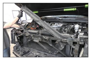
88. Cut out the supplied template at the back of this manual that corresponds to your vehicle for marking the two hole locations in the shroud that was just removed.
