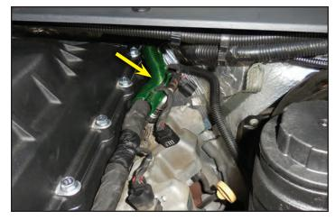
177. Reinstall the two rear coil packs on each side in their original locations. Make sure to plug in the spark plug wire at the bottom and the electrical connection at the top. Secure each coil pack with the two OEM bolts.
