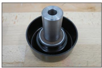
143. Apply Loctite 242 to the supplied bolt as shown below. Make sure the washer sits beneath the head of the bolt before tightening. Install the pulley with the spacer at the backside in the arrow location shown and torque to 25 ft-lbs.
