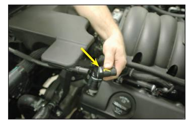
38. Loosen the clamp at the air box securing the air plenum in position using an 8mm nut driver.
