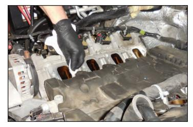
58. Apply tape to the ports to prevent any debris from entering the engine.
