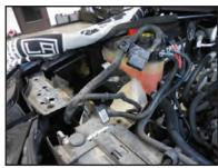
80. Push the hood release cable upward and pull it out of the retaining clip shown.
