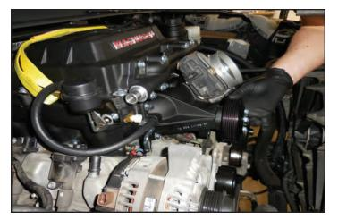
174. Remove the four supercharger lid bolts that are holding the two metal brackets that are securing the lift strap using a 12mm socket wrench. The 4 bolts will be reinstalled in the next step. Save the strap and brackets in case you ever need to remove the supercharger.
