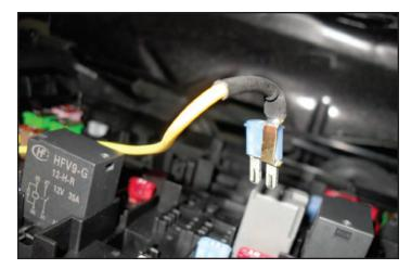
130. Replace the fuse in slot number 74 (labeled: ECM IGN) with the fuse tap installed on one leg. Press the yellow wire down into the notch you created earlier at the red arrow.
