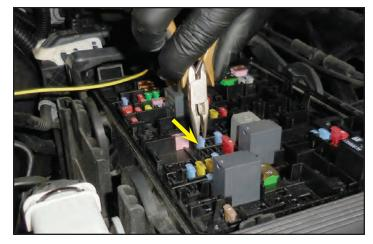
129. Connect the fuse tap end of the yellow wire from the intercooler wiring harness to one leg of the fuse just removed. It will be a tight fit.
