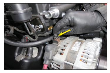
198. Plug in the provided electronic throttle control (ETC) extension wire and secure with the locking mechanism.
