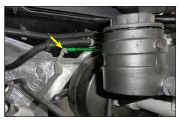
124. Remove the fuse box cover by pressing the two tabs (One shown here with an arrow) and pulling up.
