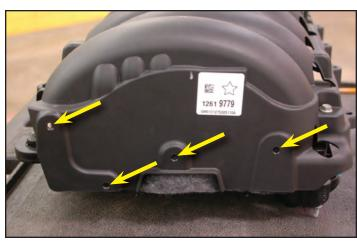
56. Pull the OEM intake manifold out of the vehicle and set aside. Parts will be used from this assembly. Gaskets, and throttle body will be reused.
