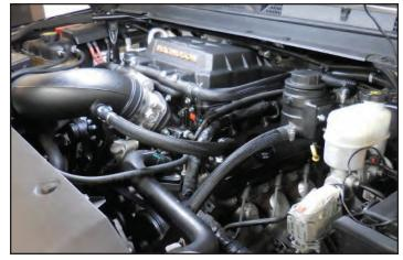
237. After the initial test drive gradually work the vehicle to wide open throttle runs, listen for any engine detonation (pinging). If engine detonation is present let up on the throttle immediately. Most detonation is caused by low octane gasoline still in the tank. Affix the Premium Fuel Only decal on the inside of the fuel fill door.
