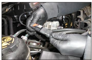
207. Remove the cable tie fastener from the arrow location and cut it free from the wiring.
