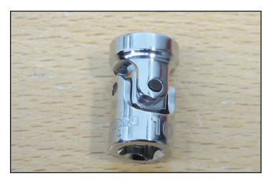
172. Use socket from the last step with a 1/4" drive long extension to tighten the 8 bolts that were just installed. Start out by spinning these bolts in place by hand without a wrench. Follow the torque order given at the back of this manual and gradually work your way up to the final torque of 120 in-lbs.
