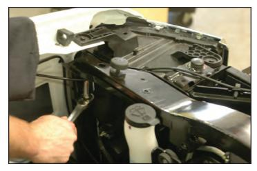
74. Remove the cross-frame support brace center bolt using a 13mm wrench.
