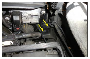
118. Gather the bracket shown below and install it at the two threaded studs and tighten in place with the original nuts.
