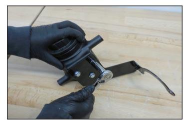
98. Remove the two nuts holding the master cylinder to the brake booster canister using a 15mm socket. One location is shown with an arrow in this image. The other nut is located on the opposite side.
