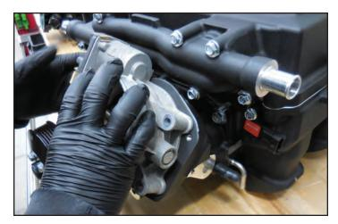
160. Install the four M6x40mm bolts with Loctite 242 on the throttle body and torque them in two stages with the final torque of 130 in-lbs.
