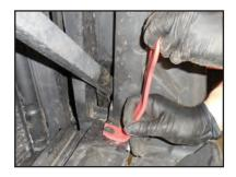
82. Remove the plastic rivet in the center of the panel shown with the arrow in the image to the right. Also remove the two corner rivets (one location shown with the arrow in the image
