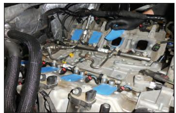
165. Wipe down the intake port outer sealing surfaces with a rag coated with Tri-flow or equivalent lubricant. Pull the coil harnesses to the sides to make clearance for supercharger installation. Ensure that there are no tools or other items left in the valley area before you install the supercharger.
