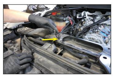
76. Pull the cross-frame support brace from the vehicle and set aside for re-installation in a later step.
