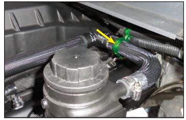
221. Gather the intake tube assembly and adapter shown. (Note: Adapter may be preinstalled in tube and will need to be removed as shown)
