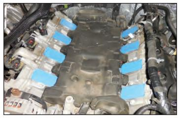
59. Remove the valley cover foam insulation from the vehicle. This cover will not be reused.
