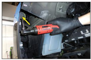
15. This picture shows the interior wheel well removed completely. There are three bolts holding the plastic retaining clip to the upper fender well mounting bracket. This clip locks the lower fascia connection in position. Remove these three bolts using a 7mm wrench to allow the lower section to be pulled free.
