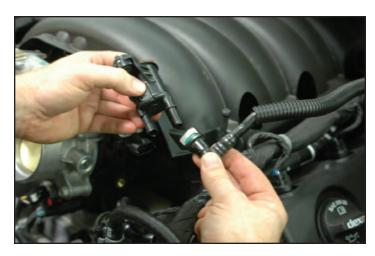
52. Remove the PCV hose from the valley cover on the left side below the throttle body. Disconnect it at the two locations shown. This hose will not be reused.
