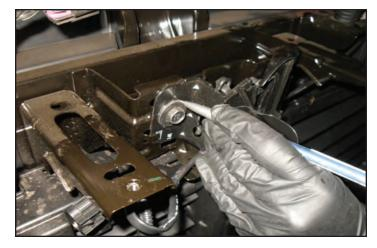
30. Use a 13mm wrench to remove the two hood latch fasteners marked in last step.
