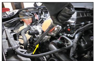
195. Use a strap wrench to hold the supercharger pulley in place while you torque it to 108 in-lbs using a 10mm socket wrench.
