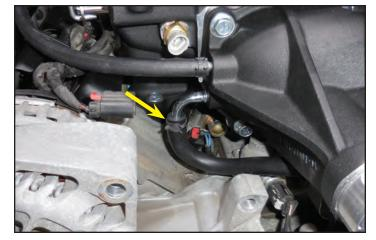
185. Plug in the MAP sensor connection and engage the locking tab shown with the arrow.
