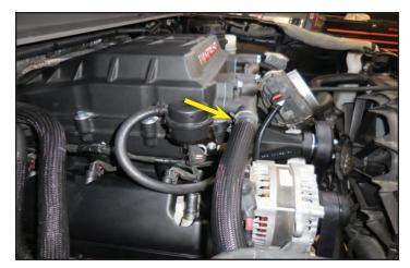
218. Lightly install another cable tie with a C-clip over the hose from the last step and clip it to the MAF/IAT breakout harness as shown highlighted in green. The cable tie should be snug on the hose so it does not restrict coolant flow.
