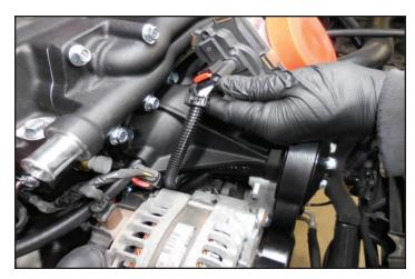
200. Tuck the excess cable under the supercharger drive cover in the arrow location. Ensure that this wire does not get into the belt path.
