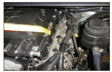
170. Gather the M6x35mm bolts and apply Loctite 242 to them as shown below. Install the driver's side front bolt first. Use a magnetic telescoping pick up tool to install the 8 supercharger mounting bolts as shown here.
