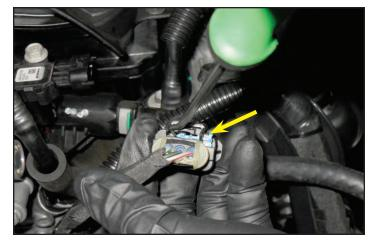
49. Use a 10mm socket wrench to remove the EVAP Solenoid from the intake manifold. This is located just behind the throttle body on the left side, below the MAP Sensor.
