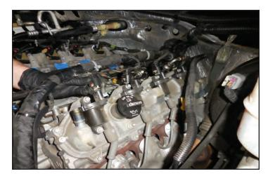
64. Unplug the spark plug wires for the back two coils on both sides. Mark the two rear coils on each side to ensure that they are installed in the original locations later. Remove the two bolts holding each of the two rear coil pack in using a 10mm wrench.
