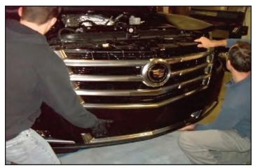
23. Disconnect the wiring from the sonar unit. Use a 7mm and 10mm wrench to remove the four bracket fasteners holding the sonar in place. If you have a 2016-17 model refer to the next step.
