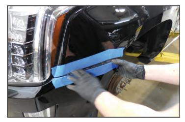
18. Lever up on the top of the fascia to release the four clips on either side of the hood release to allow the front top section to be pulled out just a bit.
