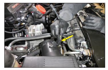
206. Connect the male plug from the MAF/IAT breakout harness to the vehicles female electrical connection and engage the locking mechanism.
