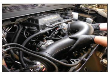
224. Tighten the two hose clamps at both sides of the intake air tube using a 7mm nut driver.
