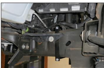
107. Install the coolant pump with the two provided Adel clamps and two M8 nuts at the yellow arrow locations. Ensure that the pump output barb is facing the direction of the green arrow. Ensure that the lower Adel clamp is about 1/2 inch from the bottom as shown. Be careful not to over tighten the M8 nuts, this can cause the Adel clamps to bend.
