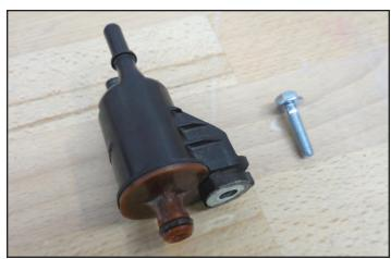
187. Install the EVAP solenoid in the location shown and secure it with the M6x25mm bolt at the yellow arrow. Plug in the electrical connection at the red arrow and the hose connection at the blue arrow.
