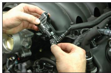
51. With the EVAP solenoid free, you can now easily disconnect the EVAP tube from the solenoid by pressing the gray release tab and pulling free. Save the EVAP solenoid. The fastener will not be reused.
