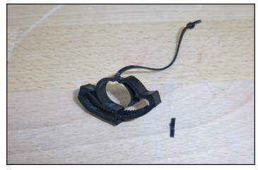
153. Install the fuel line safety clip rotated to the side as shown here to allow more clearance for the supercharger.
