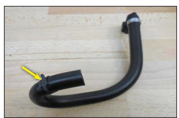
183. Install the connector from the hose assembly in the last step onto the PCV valve. You should hear a click to indicate the connector is locked. Pull up to make sure the lock is engaged.
