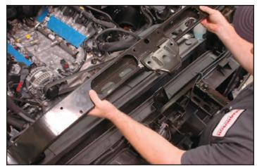
77. The arrow locations here show the three threaded holes from one side of the support brace that was removed in the last step.
