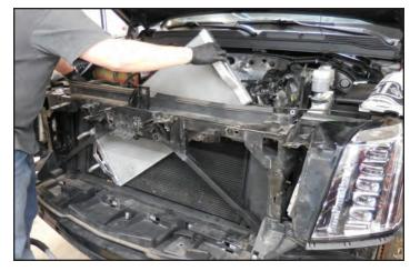
93. The LTR should now be resting on the bottom tray forward of the radiator. Center the unit and use the mounting bracket holes to align and place the mounting brackets on the "A-Frame" in front of the radiator.
