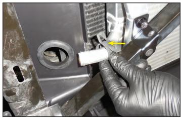
111. Slide the hose from two steps ago through the grommet and over the lower LTR hose barb and secure with the clamp as shown. The short elbow end connects to the LTR shown here.
