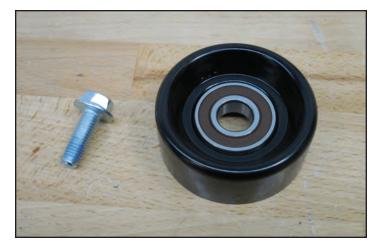
194. Install the pulley from the last step into the idler bracket from two steps ago and torque it to 25 ft-lbs using a 15mm socket wrench.
