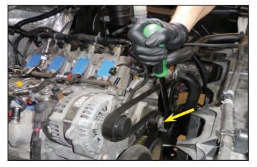
133. Remove the alternator mounting bolt shown using a 15mm socket wrench. This bolt will not get reused.
