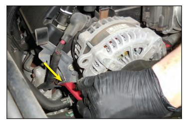
42. Remove the bolt securing the bracket in location shown using a 13mm socket wrench.
