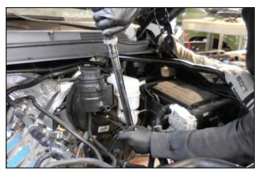
100. On the driver's side outer frame rail remove the bolt holding the plastic cover shown at the arrow using a 13mm socket wrench.
