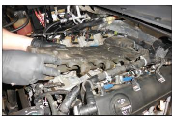
60. Remove the PCV hose from the valve cover.
