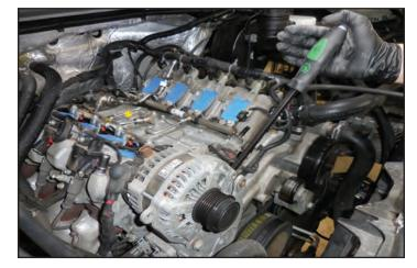
137. Remove the bolt shown with an arrow using a 15mm socket wrench. This will be replaced with a longer bolt to install an idler.
