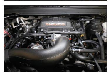
236. Test drive vehicle for the first few miles under normal driving conditions. Do not perform any wide open throttle runs. Listen for any noises, vibrations, engine misfire or anything that does not seem normal. The supercharger does have a slight whining noise under boost conditions, which is normal. Check & bleed the charge air cooler reservoir as needed.
