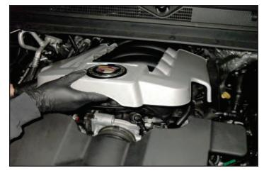
37. Depress the gray locking tab to release the PCV vent hose coming from the valve cover at the air plenum on both sides of the engine. These two hoses will not be reused.
