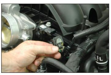
48. Use a pick tool to move the blue lock tab over from the inside if you can't get it to disengage with your finger from the outside.
