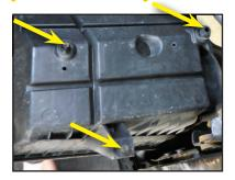
70. Next to the airbox location you will need to remove the two push pins shown with arrows.
