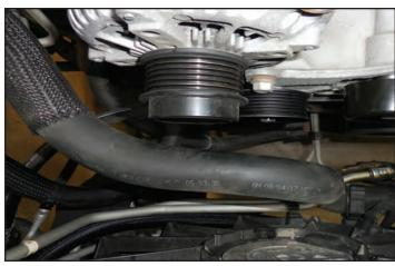
147. Wrap the radiator hose with the provided mesh as shown with the arrow.
