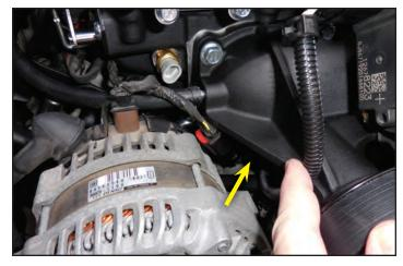
201. Cut the inner tabs out of the inside of the provided hose clip for the cable tie as shown in the photo below. Install the hose clip (highlighted in green) as shown in the image to the right with a cable tie (highlighted in red).
