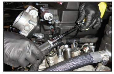
173. Spin the supercharger pulley by hand after torquing it in place to ensure nothing is binding.
