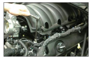
54. Be careful when pulling the manifold forward because the bolts can scratch the cylinder heads. Pull the intake manifold forward a bit to gain access to the wiring harness "tree" anchors that hold the harness to the back of the intake manifold. Use a screwdriver or tree clamp remover to unplug these trees from the OEM intake manifold.
