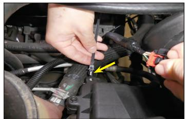
209. Route the factory wiring harness from the MAF sensor in the orientation shown highlighted in green. Secure in place with the two cable ties shown with arrows.
