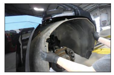
14. In the fender well (on each side of the vehicle facing up), use a 7mm socket wrench to remove the bolt from the fascia to fender.
