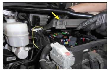
125. Flip the cover open for the positive lead at the back of the fuse center (red arrow location). Remove the nut of the positive lead (yellow arrow location) using a 13mm socket wrench. Replace the nut incorporating the eyelet terminal on the red wire from the intercooler wiring harness.
