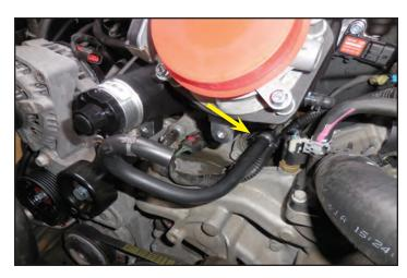
184. Install the other end of the hose from the last step on the 90° hose barb shown and secure with the spring clamp. The hose barb at this location might also be straight.
