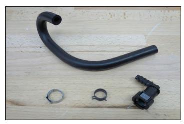
180. Insert the 90° fitting into the hose end and orient as shown.
