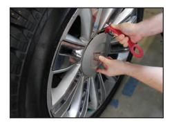
10. Use a 7mm wrench to remove the four bolts (there may only be two bolts for the 2016-17 model as shown here) at the front of the inside plastic wheel well to fascia connection on each side of the vehicle.
