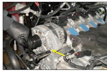
87. Loosen the other alternator support bolt shown.
