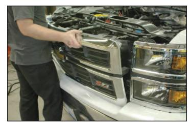
170. Replace the four bolts holding the top of the fascia/grille to the sub frame and the four bolts on the underside of the grille using a 10mm wrench.
