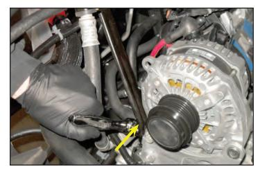
89. Pry the alternator up to rotate it out of the way.
