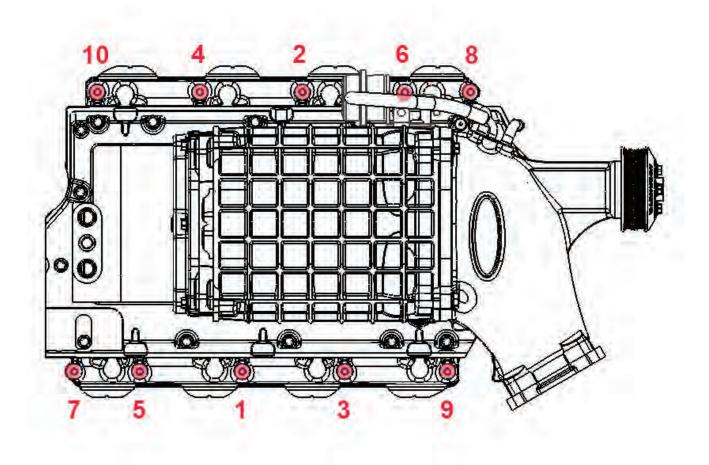
Supercharger Torque Order Diagram
