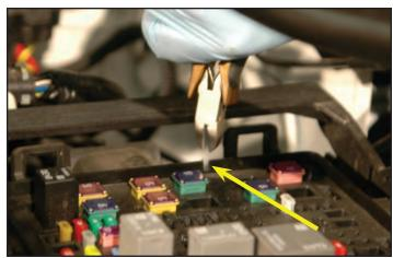
133. Remove the fuse number 3A (labeled: MISC IGN) from the slot in the fuse center. The fuse number may not be the same on your vehicle, but you should be able to find the fuse labeled MISC IGN.
