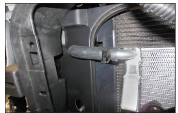
117. Gather the provided cable tie with clip attached. Remove the clip shown in the next step.
