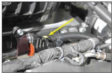
147. Connect the factory MAP sensor plug to the connector on the MAP sensor.
