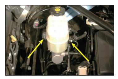
68. Replace the nuts incorporating the reservoir assembly. Torque to 25 ft-lbs. Verify your torque wrench settings.
