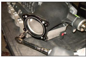
95. Install the OEM throttle body on the supercharger inlet using a 10mm wrench and torque to 106 in-lbs using the supplied 40mm long M6 fasteners.
