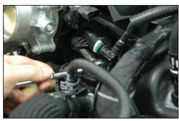
16. With the EVAP Solenoid free you can now remove the electrical connection by pressing the release tab and unplugging.
