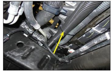
125. Install the end of the "Pump to Lower LTR" hose to the output side of the intercooler pump and secure in place with a provided worm gear clamp.
