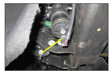
130. Secure the pump harness to the existing harness using the provided cable ties.
