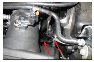
153. Push the wire loom mounting "tree" back into the hole on the back side flange of the air box.
