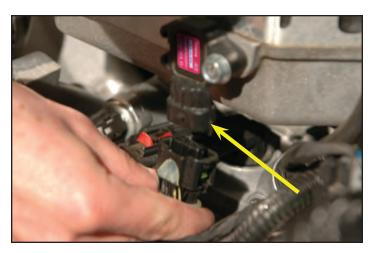
148. Connect the throttle body plug to the throttle body. Connect the alternator wire plug to the receptacle on the alternator. Some tape removal on the harness may be needed to allow the connection between throttle body, and alternator.
