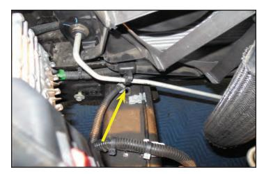
72. This step applies only to 2014-15 trucks. Use a provided zip tie to anchor the harness to the existing black brake hard line, which runs parallel to the frame rail.
