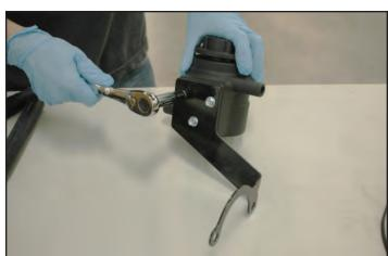
67. Remove the two nuts holding the master cylinder to the brake booster canister using a 15mm socket.
