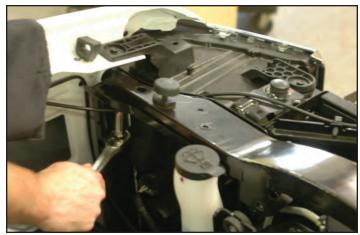
47. Remove the cross-frame support brace center bolt using a 13mm wrench.
