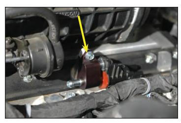
144. Connect the extended EVAP solenoid plug to the EVAP sensor. Secure the extension harness to the coil pack harness with a few of the provided zip-ties.
