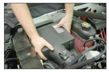
150. Route the MAF/IAT breakout harness behind the alternator. Make sure the harness will not get pinched by the alternator. Use a tie wrap to secure the harness to the factory heater hose as shown by the red arrow to the left.
