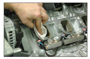
106. Clean the OEM gaskets removed from the intake manifold earlier, and install them in the grooves on the bottom of the supercharger intake manifold (one of eight shown here at the yellow arrow location). If you find any damaged gaskets you will need to replace them with GM replacement parts. The tab will line up with the slot on the outside edge.
