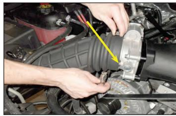
163. Tighten the hose clamps on both sides.
