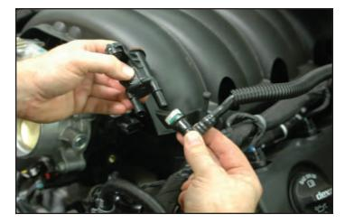
18. Remove the PCV hose from the valley cover on the left side below the throttle body.
