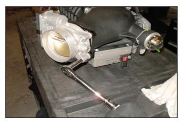
96. You should have the 3 parts shown to the right. (A) IAT sensor, (B) crush washer and (C) MAF/IAT breakout. To complete the installation of the sensor you will need a 19mm (or ¾") deep socket and a torque wrench capable of 175in-lbs (~15ft-lbs).
