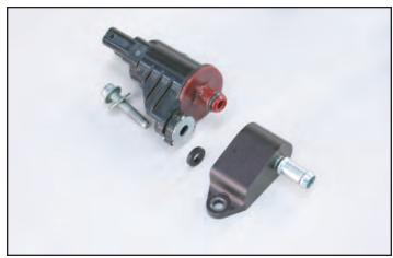
143. Mount the EVAP solenoid mounting bracket to the left side boss on the supercharger lid using the provided 16mm long bolt and secure in place with a 10mm wrench. Torque to 106 in-lbs.
