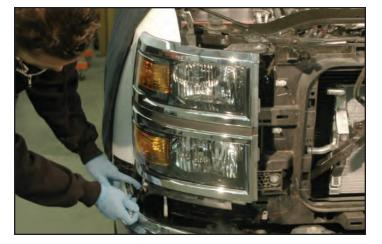
169. Replace the fascia/grille in position and push on the center of each side grille opening to reconnect the two snap clips, and the bottom guiding slots.
