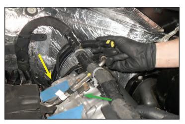
104. Remove the tape or rags covering the intake ports on the heads. Be careful to not allow any debris to fall into the exposed ports.
