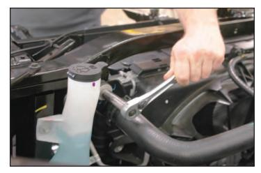
42. Remove the two upper-forward, diagonal fender-brace bars using a 10mm wrench.
