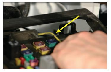
137. Replace the cover on the fuse center engaging the snaps. The lid should NOT be crimping down on the yellow wire.
