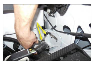
128. Place the relay on the stud closest to the firewall and secure with a supplied 6mm nut, using a 10mm socket. Use the remaining supplied 6mm nut to secure the fuse holder to the bracket. Make sure to route the wires to the fuse holder as shown, so that they do not rub on the sheet metal below.
