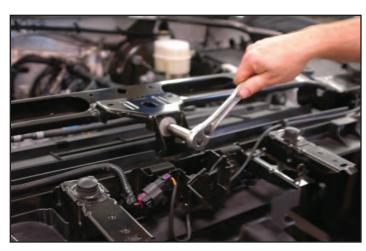
48. For 2017 or newer Sierra/Silverado. The bolt for the window washer reservoir may need to be removed to allow clearance for removing the cross-frame support brace.
