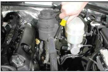
79. Route the other end of the hose from the last step forward and down to connect to the intercooler pump inlet hose barb using a provided wide band spring clamp.
