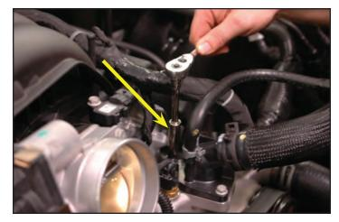
22. This does not apply to the 2017 or newer Sierra/Silverado. Use a 10 mm wrench to remove the bolt from the lower mounting bracket anchoring the wire harness.
