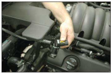
7. Loosen the clamp at the air box securing the air plenum in position.
