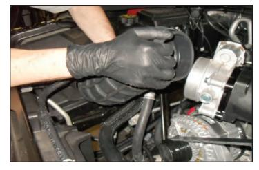
162. Install rubber duct onto throttle body side, and install hose clamp around connection. Make sure duct tabs line up with throttle body indicated with arrow.
