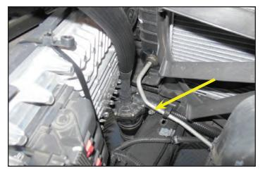
126. Install the provided fuse in the charge air cooler pump wiring harness fuse holder, and replace the cap.
