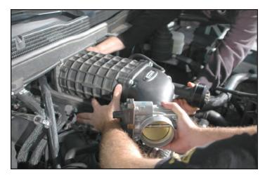
108. Apply blue Loctite 242 to the ten provided 75mm long supercharger mounting bolts. Install supercharger mounting bolts and torque in position to 106 in-lbs using a 10mm wrench. Follow the torque order given at the back of the book. At this point also reinstall the bolt holding the fuel injection line to the left side of the engine that was removed earlier.
