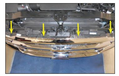
38. Pull straight out on the fascia/grille to disconnect the two remaining snap clips at the center of each side, and the bottom guiding slots. Set the fascia/grille aside carefully for later reinstall.
