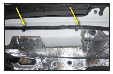
102. Remove the factory EVAP hose from behind the left side cylinder. Squeeze the connector clip to release the clip and pull free.
