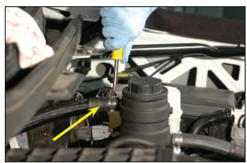
115. Route the hose from the right hand side of the charge air cooler forward, down, and route it through the upper hole made in the plastic near the radiator as shown with the yellow arrow.
