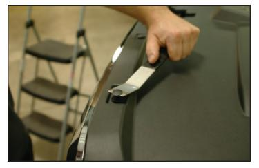
33. This does not apply to the 2017 or newer Sierra/Silverado. Remove the front wheel well fender trim from both sides by removing the 6 bolts located around the perimeter.
