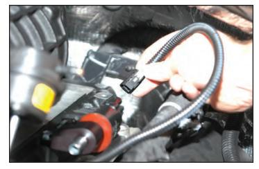
145. Connect the provided 10" x 3/8" PCV hose between the EVAP solenoid and the supercharger inlet hose barb. No clamps are required. If necessary adjust the hose length to prevent rubbing on supercharger bolt head.
