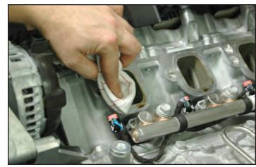
31. Use tape or clean shop towels to cover over your intake ports. It's important to keep these ports clean and avoid any debris falling into the exposed openings.
