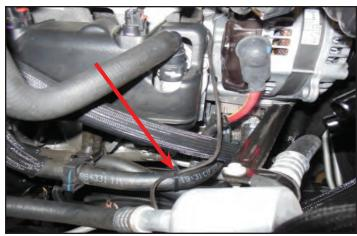
151. Continue to pass the MAF/IAT breakout harness to the right underneath the AC line. Secure the MAF/IAT breakout harness with another tie wrap to the factory MAF harness as shown by the red arrow to the right. \*Note: The green arrow is a reference to the tie wrap installed in the previous step.
