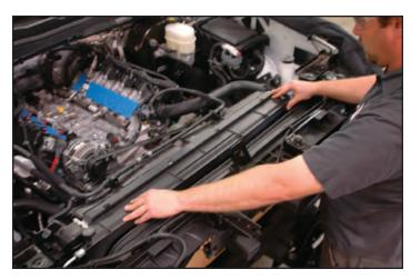
64. Replace the upper radiator cross-frame brace and secure with the OEM mounting bolts.
