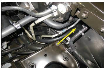
123. Connect the hose from the last step to the lower LTR barb and secure in place with a provided wide band spring clamp.
