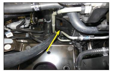
122. Route the end of the "Pump to Lower LTR" with the 90° bend through the hole made in the plastic cover earlier (shown with an arrow).
