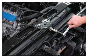
65. Replace the upper radiator mounting bolts and vibration dampers.
