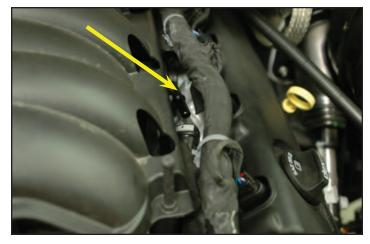
21. Use a 10 mm wrench to remove the nut holding the wire harness to the base of the bracket in front of the left side valve cover.
