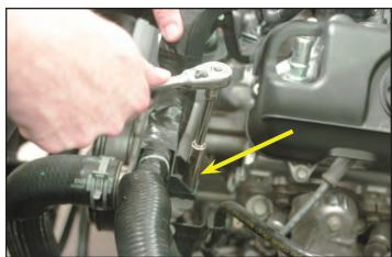
23. Remove the three harness "tree" clamps from the left side of the intake manifold.
