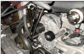
113. Install the provided accessory drive belt using the drive belt routing diagram. A larger diagram is included at the back of this book.
