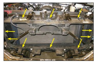
54. Here you can see the three lower locations after the rivets have been removed.
