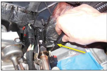
103. Connect the gray end of the new provided EVAP hose shown to the location where the factory EVAP hose was just removed (shown with a yellow arrow). Remove the bolt holding the fuel injection line in place (shown with a green arrow) to allow clearance while the supercharger is being installed. This bolt will be reinstalled after the supercharger is mounted.
