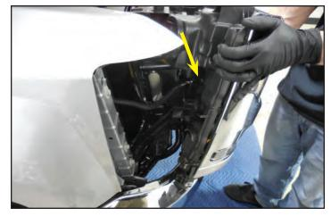
41. Remove the two upper radiator mounting bolts using a 13mm socket.
