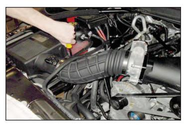
164. Connect the free end of the PCV hose from the left hand side front valve cover hose barb onto the lower hose barb of the air tube (Indicated with a blue arrow). Connect the provided 90° PCV hose between the hose barb on the right hand side front of the valve cover and the remaining upper hose barb of the air tube as shown.
