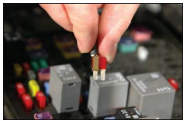
135. Replace the fuse in slot number 3A (labeled: MISC IGN) with the fuse tap installed on one leg.
