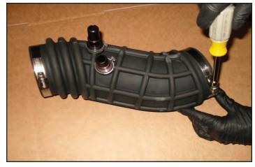
161. Install the rubber duct from previous step on the air box. Apply Lubriplate grease to the side near the throttle body to help it slide better.
