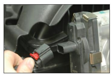
12. Disconnect the alternator control sensor plug from the alternator.
