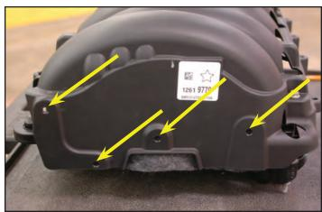
27. Pull the OEM intake manifold out of the vehicle and set aside. Parts will be used from this assembly. Gaskets, and throttle body will be reused.
