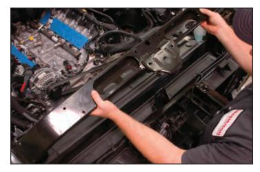
50. Pull up on the upper radiator shroud to unsnap it from the retaining slots, set aside for later re-install.
