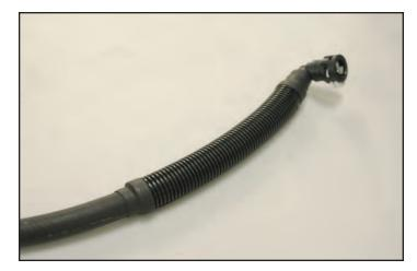
158. Connect the 90° hose barb on the uncovered side of the PCV hose to the left hand side front of the valve cover hose barb. Route the hose under the supercharger inlet toward the right hand side of the vehicle. The split loom covered section of the hose should be on the right hand side above the alternator.
