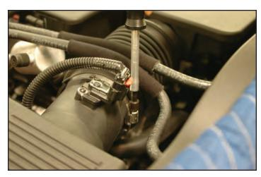
8. Remove the air intake plenum from the vehicle. This will not be reused.
