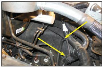
131. Remove the fuse center cover by pressing the release tabs and lifting up.
