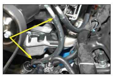
156. Push the two provided zip-tie "tree" connectors into the two bolt holes in the front of the supercharger intake manifold. The flat part of the connector should be pointing up.
