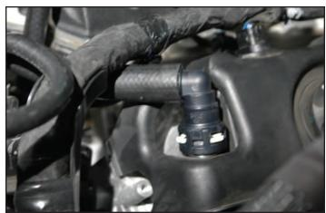
159. Anchor the PCV hose to the front of the supercharger intake manifold using the installed zip-tie tree mounts.
