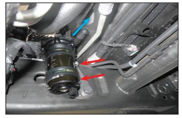
77. Refer to the expanded diagram at the end of the instruction manual to prepare your intercooler system plumbing hoses for install. When measuring the mesh sleeve make sure it is in a relaxed state.
