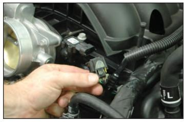
15. Use a 10mm wrench to remove the EVAP Solenoid from the intake manifold. This is located just behind the throttle body on the left side, below the MAP Sensor.
