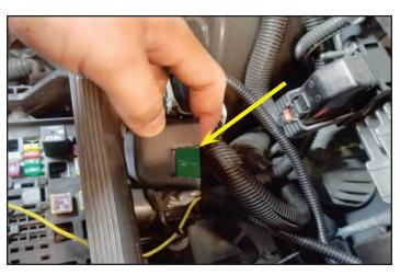
140. Connect the black ground wire eyelet terminal to the existing grounding bolt at the firewall on the left hand side, just above and inside the brake booster canister.
