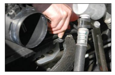
154. Clean up your wiring adding zip-ties as needed to secure the wiring.
