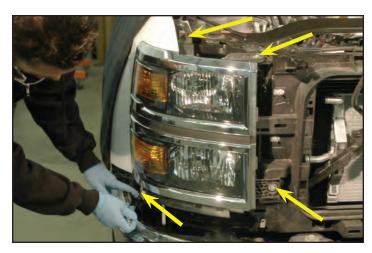
40. This does not apply to the 2017 or newer Sierra/Silverado. Lift up carefully on the headlight to separate it from the frame and disconnect the wiring harness plug (shown at the yellow arrow location) by pressing the release tab and pull it free. Set the headlight aside in a safe spot to be reinstalled in a later step. Repeat the removal process on the left side headlight..
