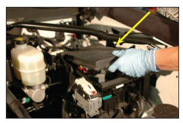
132. Cut a small slot in the back lip of the fuse center tray as shown.
