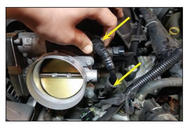
20. Rotate the hose approximately 180° to gain access to the release tab on the left side valve cover, depress the tab and pull the hose free from the vehicle. Set aside for later usage.
