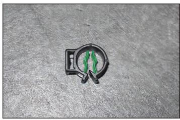
119. Here you can see the two tabs on the left that have been removed from the clamp on the right. Reinstall this clip onto the cable tie.
