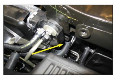
116. Connect the hose from the last step that came from the right side of the charge air cooler to the upper LTR barb and secure with a wide band spring clamp. Secure the hose along its path with a few provided zip-ties.
