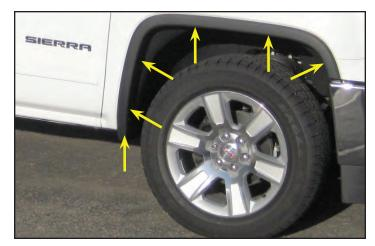
34. This does not apply to the 2017 or newer Sierra/Silverado. In the fender well, use a 7mm wrench to remove the two bolts (on each side of the vehicle) at the front skirt holding the fascia/grille bottom panel to the sub-frame.
