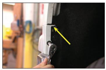
35. This does not apply to the 2017 or newer Sierra/Silverado. Carefully pull out on this fascia bottom panel to unsnap it from its location
