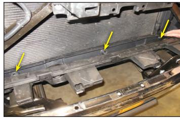
55. Once the rivets have been removed you will have to pull the sides of the panel inward to release them from their locations as you pull upward. Be careful not to damage any radiator fins while you remove this panel.
