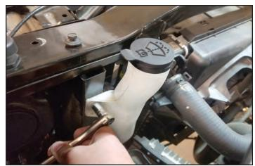
49. Pull the cross-frame support brace from the vehicle and set aside for re-install in a later step.
