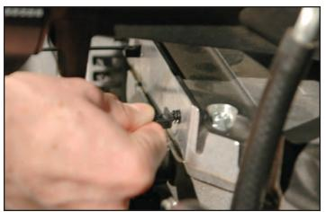
157. Slide the provided 8" section of split loom over the PCV hose and anchor in place at each end using two 1" pieces of the provided heat shrink as shown. The opposite side of this hose will be connected in the next step.
