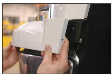
36. This photo shows the hidden locations for the six clip retainers (shown with yellow arrows) for the fascia bottom panel from the last step. Have an assistant hold the panel while you pry at these six locations to remove the panel. The red arrow locations show the four lower mounting areas for the grille that will be referred to in the next step. (Red arrow locations are not on the 2017 or newer Sierra/Silverado).
