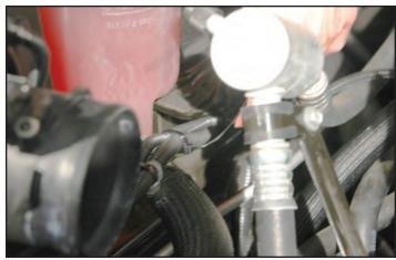
155. Connect the provided PCV hose with the blue colored quick connect locking pin between the existing valley cover hose barb on the left side and forward supercharger inlet hose barb.
