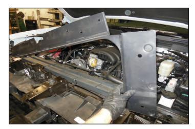
57. Cut out the provided template for your vehicle and install it in the location shown on the panel just removed. There is a specific template for the Sierra or Silverado. Use this template to mark the location for the two holes, and cut the holes out using a rotary tool or knife.
