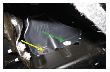
70. This step applies only to 2014-15 trucks. Use a 15mm socket to remove the right hand
