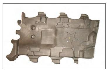
84. Install trimmed insulator from last step into manifold valley.
