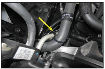
121. Slide the long straight section of the "Pump to Lower LTR" hose through the space shown with the arrow. This will be routed to the output of the pump.
