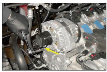
88. This does not apply to the 2017 or newer Sierra/Silverado. Remove the bracket located next to the alternator it will be re-attached later.
