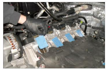
105. Wipe intake port sealing surfaces clean with lacquer thinner, alcohol, or some other non-petroleum based solvent.
