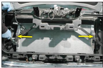
63. Replace the upper radiator shroud by snapping into place.
