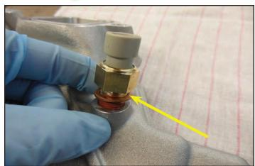
99. Once the sensor is snug to the crush washer use a 19mm (or ¾") deep socket attached to your torque wrench and torque to 175in-lbs (~15ft-lbs).
