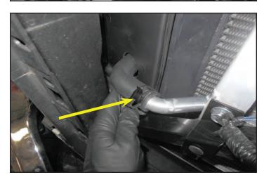
124. This view is from under the vehicle looking to the left front. Run the opposite end of the "Pump to Lower LTR" hose behind the lower portion of the radiator as shown and secure in place with provide cable ties as shown with the arrow.
