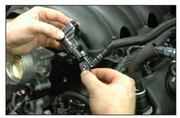
17. With the EVAP Solenoid free, you can now easily disconnect the EVAP tube from the Solenoid by pressing the gray release tab and pulling free. Save the EVAP Solenoid, and its fastener, for a later step.
