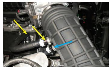
165. If you disconnected the reservoir overflow hoses earlier, reconnect using the OEM clamps. Ensure that you remove any plugs that you may have installed on these hoses.
