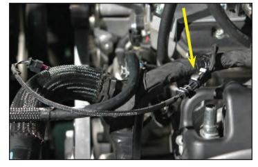
142. Mount the OEM EVAP solenoid to the provided mounting bracket using the factory mounting bolt and provided spacer using a 10mm wrench as shown. The washer may not be on original bolt. Add blue Loctite 242 to bolt before installing. The black spacer should sit between the solenoid and bracket.
