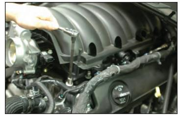
25. Pull the intake manifold forward a bit to gain access to the wiring harness "tree" anchors that hold the harness to the back of the intake manifold. Use a screwdriver or tree clamp remover to unplug these trees from the OEM intake manifold.
