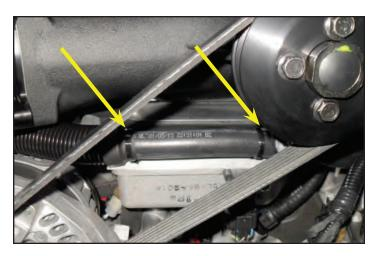
160. Gather the rubber duct shown. Loosen hose clamps to prepare for install. The left side clamp will be taken off completely to install over throttle body.
