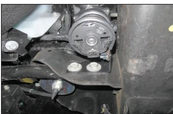
75. This step applies only to 2016 and newer trucks. Install the provided intercooler pump bracket shown on the left side inner frame rail using the provided bolt (shown with a yellow arrow) in the OEM threaded hole. The metal tab will line up with the hole shown with the green arrow to maintain proper alignment.
