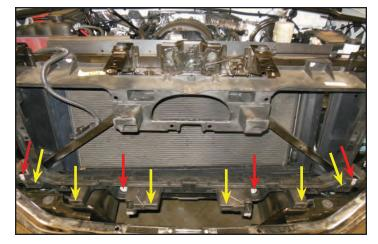
37. Remove the four bolts (shown with arrows) holding the top of the fascia/grille to the sub frame using a 10mm wrench. Also remove the four bolts from the lower portion of the grille that were mentioned in the last step.
