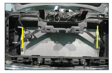
62. Attach the mounting brackets to the LTR mounting flange using the supplied bolts and a 12mm wrench. Do not tighten until you have aligned the LTR to be level, cross checking against the existing horizontal lines of the radiator. Secure in place when you've got proper alignment.
