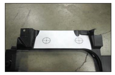
58. Install the two provided grommets at the hole locations. Now re-install the panel back into its original location using the OEM push rivets.
