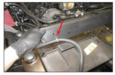
53. Remove the plastic push rivets from the plastic panel that is located around the radiator. This is the same shroud that retainer clips were removed from in the last two steps. There are 3 push rivets on top, 2 on each side, and 3 on the bottom. All the rivet heads are hidden from view in this photo. The top and bottom rivets are located on the back sides of this panel.
