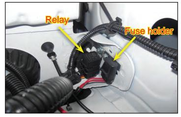
129. Route the plug from the wiring harness down to the inside of the fuse center, along the existing wiring harness and plug into the intercooler pump connector.
