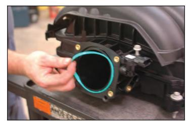
94. Install the throttle body adaptor plate, and torque to 106 in-lbs. Install the throttle body gasket removed earlier in the groove of the supercharger inlet. If the throttle body adaptor provided has a gasket you will not need to use the old one.
