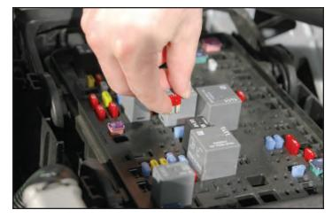
134. Connect the fuse tap end of the yellow wire from the intercooler wiring harness to one leg of the fuse just removed.
