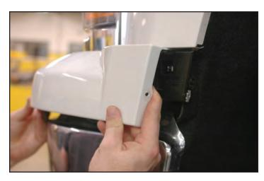
172. In the fender wells, use a 7mm wrench to replace the two bolts (on each side of the vehicle) at the front skirt holding the fascia/grille bottom panel to the sub-frame.
