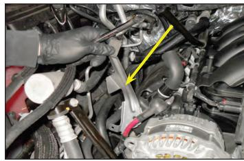
11. Disconnect the ETC connector from the throttle body. Depress the locking tab and pull the connector free.
