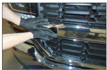
39. This does not apply to the 2017 or newer Sierra/Silverado. Use a 10mm wrench to remove the four headlight mounting bolts on the right side of the vehicle. (This is a photo of a Silverado headlight. The Sierra has the same mounting locations.)
