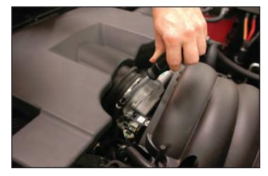
6. Depress the gray locking tab to release the PCV vent hose coming from the valve cover at the air plenum on both sides of the engine. Remove these two hoses for later reinstallation.
