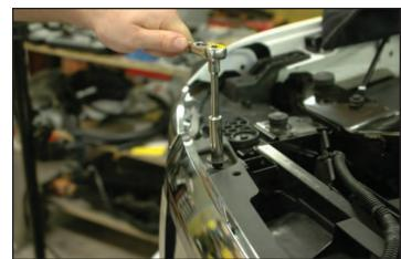
171. Carefully push in on the fascia bottom panels to snap the retaining clips into position.
