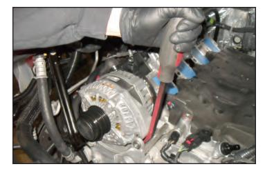
90. Alternator shown rotated out of the way.
