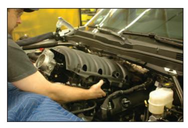
28. Carefully remove the valley cover foam insulating blanket from the vehicle. This will be reused after trimming in a later step.
