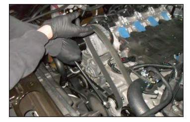
86. Remove the left alternator mounting bolt shown using a 15mm wrench.
