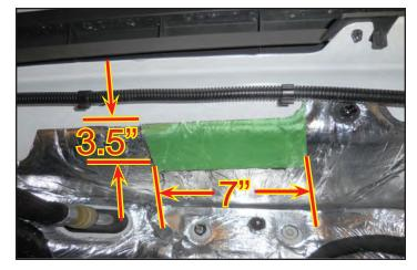
101. Here is a photo of the insulation after it has been modified. Also at this time you may find it helpful to temporarily detach the two clips holding the wiring harness at the locations shown with the arrows here to provide more clearance for the supercharger installation. You can replace these two clips once the supercharger is installed.
