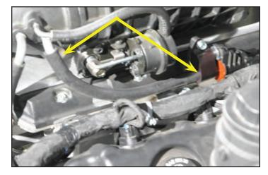
146. Connect the opposite end of the supplied EVAP hose, that was connected to the rear of the left hand side head where the factory hose was removed earlier, to the EVAP solenoid where shown with the arrow. The yellow locking clip end goes to the solenoid, and the gray locking clip end goes behind the cylinder head. Ensure that both "click" into locking position.
