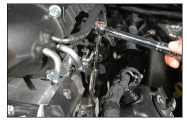
109. Plug the IAT end of the MAF/IAT breakout harness into the sensor.
