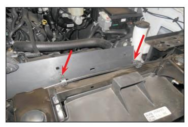
52. Remove the retainer holding the wiring harness shown with an arrow.
