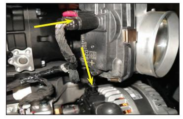
149. Replace the factory air box by pressing into position until the unit snaps in place.
