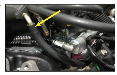
102. Remove the OEM brake booster check valve from the end of the hose on the OEM intake manifold.
