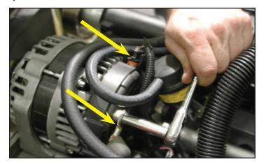
109. Attach the supplied nose cover support bracket to the tensioner bracket assembly using the provided 12mm bolts. Press up firmly under the nose cover and torque to 18-20 ft-lbs, verify your torque wrench settings.
