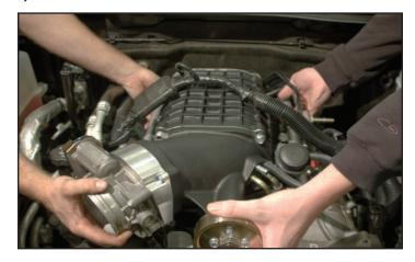
85. Use a 10mm wrench to anchor the new intake to the heads with the ten provided M6x65mm bolts. Tighten using a center-out, criss-cross pattern and torque to 106 in-lbs. Verify your torque wrench settings.
