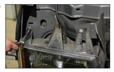
163. Snap the grille back into place using the seven OEM snap connections in the appropriate receiving slots.
