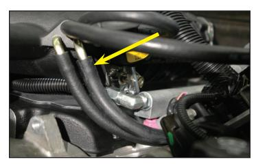
106. Connect the provided fuel line extension to the OEM fuel line hose. Connect the end of the extension to the driver side fuel rail manifold as shown.
