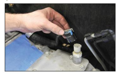
38. Use a 1-1/16" wrench to remove the Oil Pressure Sensor from the valley cover.
