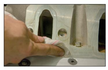
83. Spray a mist of silicone lubricant or mild soapy water on the port surfaces to facilitate the supercharger install.
