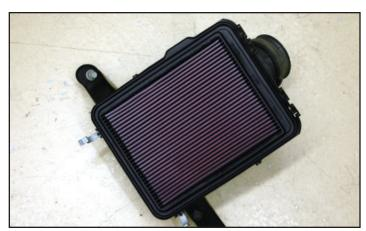
158. Install the air box back in its original location with the stock hardware. Tighten down using a 13mm wrench.
