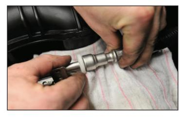
25. Use a 10mm wrench to remove the alternator power connector cable.
