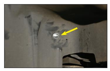
142. Drill a second ¼" hole in the provided intercooler reservoir mounting bracket as shown.
