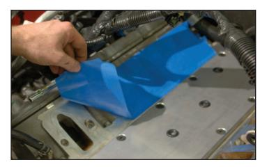
82. Wipe the surfaces clean using a non-petroleum based solvent (alcohol-lacquer thinner, etc).
