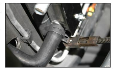
148. Cut the hose to fit so that it connects to the discharge barb of the intercooler pump and secure with a provided spring clamp. Slide a section of the provided split loom over the hose to protect it from chaffing at the pass through hole as shown.
