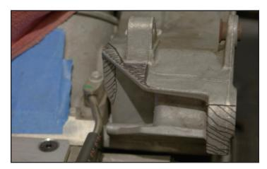
52. You can start your cuts with a reciprocating saw or cutting wheel, and finish off with a grinding wheel. These pictures show the two areas of concern. Take note that the pulley mounting boss needs cutting both on the inside edge and into the bottom curve. Test fit with the new Tensioner Mounting Bracket.
