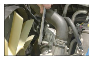
60. Here are the new belt tensioner and supercharger nose support bracket assemblies.
