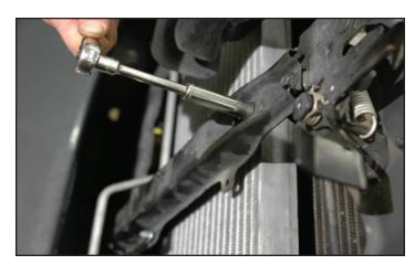
134. Remove the factory air box using a 13mm wrench on the two hold-down bolts and pull free.
