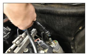
21. Rotate the PCV hose 90° clockwise and pull up on the intake manifold PCV connector to remove the line from the Intake Manifold.
