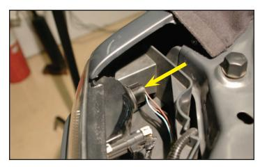
166. These are the intercooler pump wiring components.
