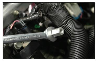
95. Install the provided EVAP Solenoid mounting bracket on the spacer just installed using the provided 10mm bolt as shown.
