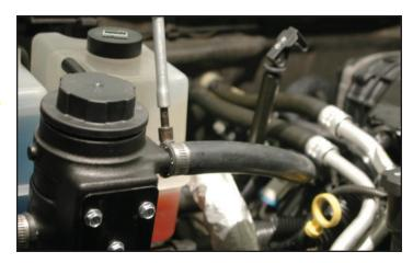
154. Cut 1-1/2" of the short leg of the other provided 4" x 36" x 3/4" 90° elbow hose. Attach the modified short leg to the driver side hose barb exiting the lid behind the supercharger. Route the hose toward the passenger side fender parallel to the just installed hose then down toward the intercooler pump.
