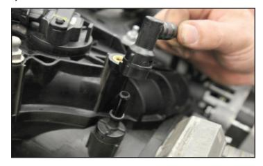
18. Use a small screwdriver to depress the locking clip of the EVAP Solenoid mounting bracket and pull the EVAP Solenoid up off the bracket.
