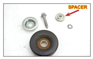
62. Mount the new tensioner bracket using the three 15mm and one 13mm bolt (on the bottom bracket hole). The removed idler pulley goes back in the original location without the spacer. Torque the bolts to 40 ft-lbs. Verify your torque wrench settings.
