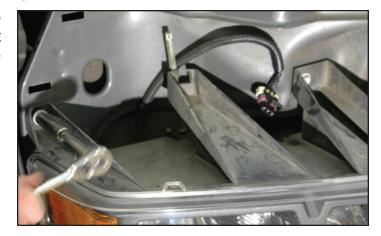
137. Using a 1-1/2" hole saw, cut a hole through the foam and fascia framework at the passenger side adjacent to the headlight. Align the bottom with the existing AC line push clamp, about 1-1/2" from the mount as shown.
