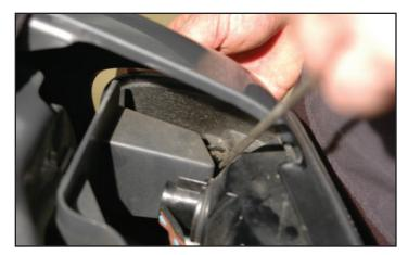
124. Remove the grill section from the vehicle. There are seven metal pinch clips that press into slots of the mounting frame. Carefully lever these clips out using a long screwdriver. Be careful of what you use for a fulcrum. This picture shows you a close up of the pinch clips.
