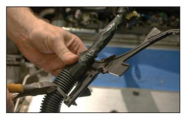
64. Temporarily disconnect the clip anchoring the wiring harness to the passenger side wheel well, just in front of the coolant reservoir.
