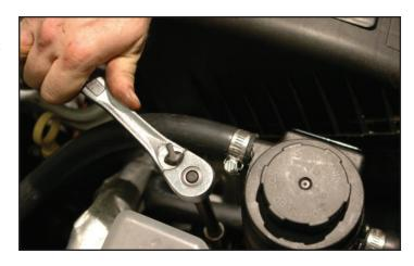
159. Connect the MAF plug back on the air box.
