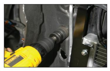
139. Remove the forward push pin rivet above the vertical flap bend of the passenger side wheel well. This is near where the wheel well begins to turn toward the forward face as indicated in this picture.
