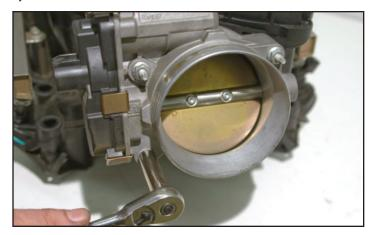
73. Remove the two studs from the OEM intake manifold using a #5 internal Torx socket.
