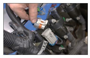
66. Disconnect all eight plug wires from the coil packs.
