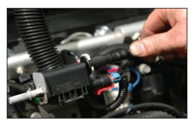
99. Cut a section of the provided 3/8" hose to 12-1/2" in length. Attach one end to the forward pointing EVAP Solenoid barb using a provided worm gear clamp and route the other end to the hose barb adjacent to the Bypass Actuator hose as shown.
