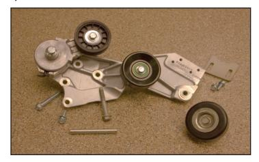
61. Pry off the retaining clip and remove the spacer from the OEM Idler Pulley that was removed from the alternator mount earlier.
