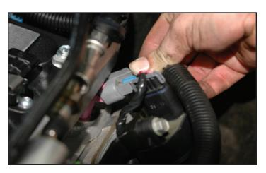
92. Re-connect the main harness clip on the passenger side wheel well, just in front of the coolant reservoir.
