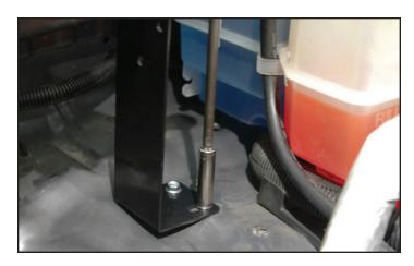
146. Attach the intercooler reservoir to the mounting bracket with the provided 10mm bolts, tighten securely.
