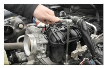
32. Carefully remove the OEM intake manifold from the engine and set aside. Some parts will be removed later for installation on the new supercharger assembly.
