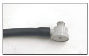
104. Plug the brake booster check valve into the grommet of the brake booster.
