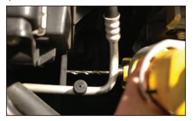
173. Open up the holes on the intercooler pump harness fuse holder and relay with the ½" bit.
