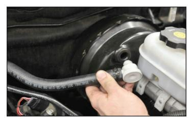
23. Pull up on the rear of the fuel line safety clip and remove the clip.
