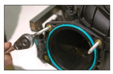
74. Place a bead of the provided Lubriplate lubricant in the groove of the new supercharger inlet and press the provided O-ring into place.
