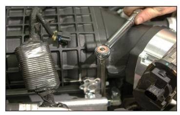
86. Remove the plastic loom covers from the coil pack harness using a small screwdriver to release the locking tabs of the four hold down clips.
