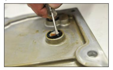
42. Press the removed O-rings into the same location grooves of the supplied valley cover.
