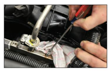
11. Disconnect the throttle body control plug.
