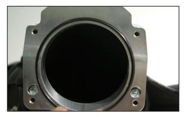
75. Install the two studs removed from the OEM intake into the top mounting holes of the new supercharger inlet. Tighten with a #5 internal Torx.
