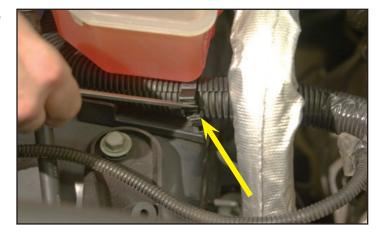
65. Disconnect the main coil pack connection from both of the coil packs.
