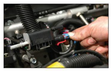
98. Connect the rear EVAP Solenoid tube to the EVAP Solenoid.
