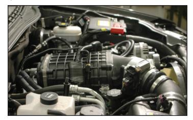
189. Test drive the vehicle for the first few miles under normal driving conditions. Do not perform any wide open throttle runs. Listen for any noises, vibrations, engine misfiring, detonation (pinging) or anything that does not seem normal. The supercharger does have a slight whining noise under boost conditions. This is normal.
