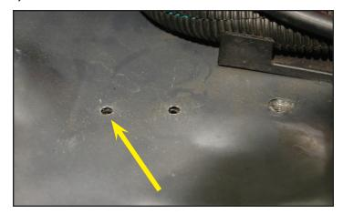
145. Using the provided 10mm bolts and nuts, secure the reservoir mounting bracket to the wheel well as shown. Tighten securely.
