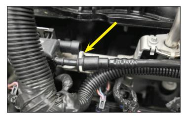
17. Disconnect the EVAP Solenoid hose from the top of the OEM intake manifold.
