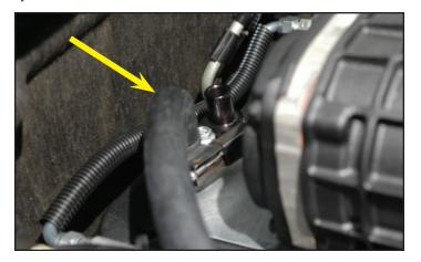
153. Route the hose over the wire loom, under the AC condenser lines and over to the intercooler reservoir. Cut to fit, and secure to the reservoir inlet barb using a provided WORM GEAR clamp. IMPORTANT: Clamps on the reservoir must be WORM GEAR!
