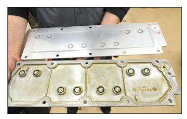
43. If you had to remove the valley cover gasket from the OEM valley cover, reinstall on the valley at this time. Use a 5mm Allen socket to install the provided eleven countersunk Allen bolts and torque to 18 ft-lbs. Verify your torque wrench settings. Press the supplied O-rings into the top surface of the new valley cover, a small dab of Black RTV silicone will hold the O-rings in place.
