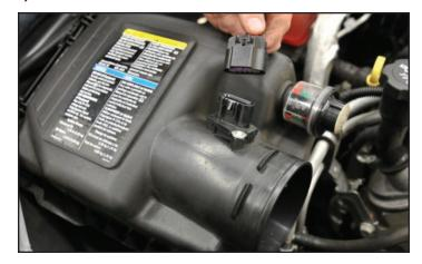
14. Disconnect the injector plugs from the eight injectors by pulling out on the release clip and pulling the injectors free.
