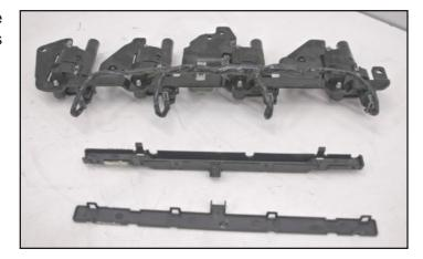
89. Replace the modified coil packs back in position and secure using the original hardware. Torque the bolts down to 106 in-lbs. Verify your torque wrench settings.
