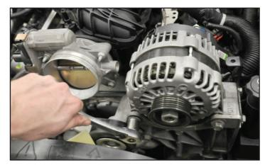
29. Remove the bolt holding the wire harness to the top of the OEM intake manifold, using a 10mm wrench.
