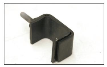
133. Holding the vertical brace in stock position, using the vacated wire loom hole as a reference, press the lower heat exchanger bracket over the heat exchanger bottom surface, stud facing forward. Replace the original bolts in their proper location and mount the vertical brace back between the upper and lower cross frame members. Incorporate the lower mounting bracket in the vacated hole and tighten securely with the provided nut. Verify all five bolts/nuts are secure.
