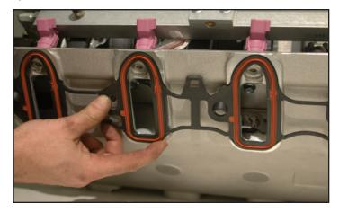
81. Verify that your valley cover area is clean and remove the tape or rags you have used to cover the intake ports of the heads.
