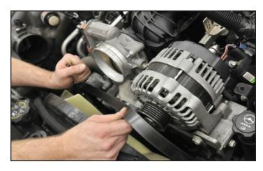
28. Use a 15mm socket to remove the alternator mounting bolts and remove the alternator from the vehicle, set aside for later install.
