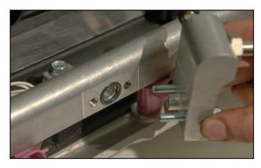
79. Torque the mounting bolts to 106 in-lbs using a 10mm wrench. Verify your torque wrench settings.
