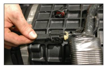
115. Route the other end of the provided harness behind the supercharger and connect to the MAP sensor.
