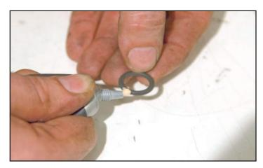
78. Mount the fuel manifold to the fuel rail using the provided hardware ensuring that the O-ring stays seated.
