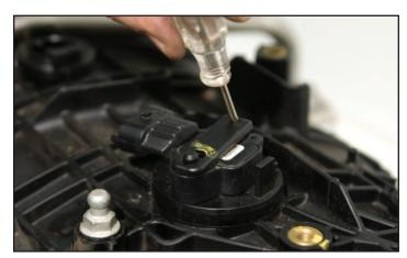
70. Place a bead of the provided Lubriplate lubricant on the MAP Sensor O-ring.
