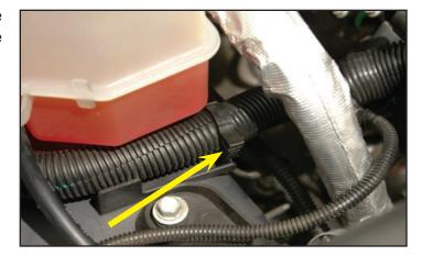
93. Use a knife or dykes to remove the wiring harness clip on the driver side of the engine that used to hold the wiring harness to the coil pack mounting stud.
