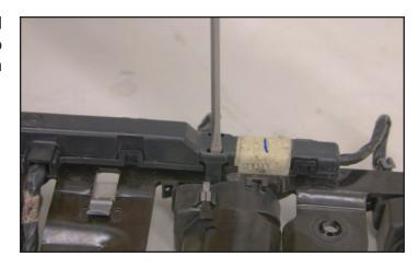
87. Split the covers from the bases again using a small screwdriver on the ten locking tabs. Remove the covers completely, these will not be reused.
