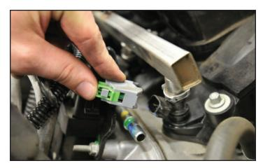
15. Disconnect the control plug from the EVAP Solenoid.
