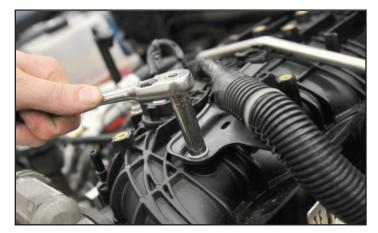
30. Pull the wiring harness off the mounting studs of the coil packs on both sides of the engine.
