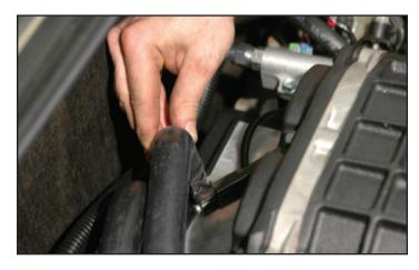
155. Using the remaining 4" x 18" x ¾" 90° elbow hose, cut the short end of the hose to center the hose as it passes through the framework as it mounts to the upper heat exchanger hose barb. Secure the hose with a provided spring clamp on the heat exchanger hose barb, and cover the hose as it passes through the fascia framework with a section of the provided split loom to protect it from chaffing.
