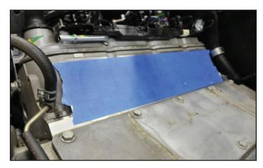
35. It will be necessary to drain some coolant from the system because the steam vent pipe will be replaced. Loosen the two bolts that secure the thermostat assembly with a 10mm wrench. Catch the coolant in a clean drain pan for reuse. Re-tighten the thermostat bolts after draining is complete, torque the bolts to 106 in-lbs. Verify your torque wrench settings.
