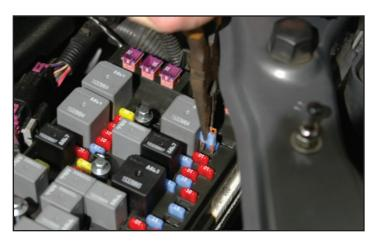
171. Insert the provided 15A fuse in the intercooler pump harness fuse holder and replace the cap.
