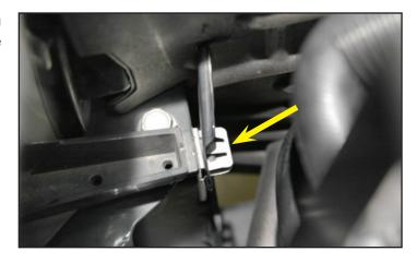
164. Pull up on the small tab of the four upper locking clips to secure the grille.
