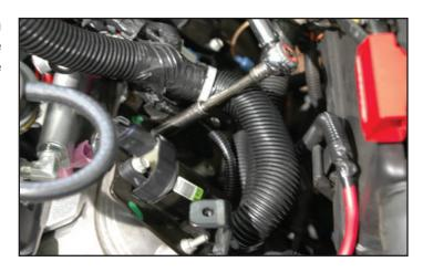
90. Re-connect the male coil pack connectors, and plug wires to the coils.
