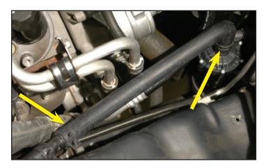
151. Put a section of the provided split loom over the hose just installed to protect it from chaffing against the air box and adjacent AC condenser lines. Use provided zip ties to anchor to adjacent lines as shown.
