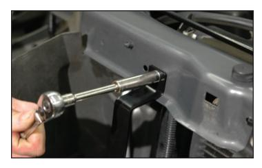
131. Remove the wire loom clip on the vertical brace removed earlier. This hole will be used to attach the lower heat exchanger mounting bracket.
