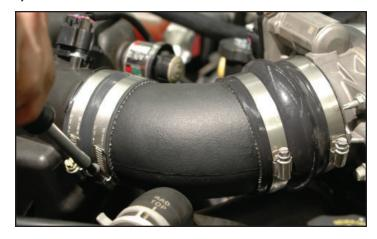
161. Connect the provided 3/8" hose to the passenger side PCV barb pointing forward below the oil fill spout on the valve cover. Route the hose up to the air tube barb, cut to fit and press onto the barb, no clamps are necessary.
