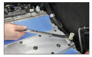
46. **IMPORTANT!** If your vehicle comes with this stud-nut mount by your valley cover, cut the stud off flush with the top of the nut, or replace the stud with a bolt. See close up in next step.
