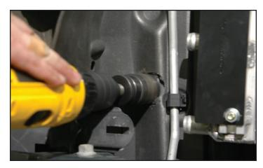
138. Drill a second hole above the first one, centered on the existing depression. Clean up your edges with a rat-tail file or grinding wheels.
