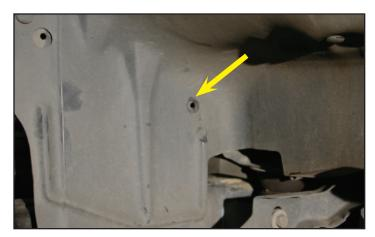
140. Assemble the intercooler pump mounting bracket in this sequence: Provided bolt through Adel clamp with pump inserted, Adel clamp leg pointing back, on the opposite side of the discharge barb. Next is the provided spacer, followed by a provided washer. Press this assembly through the hole just vacated by the push pin into the wheel well with the pump inlet pointing up and the discharge barb pointing forward as shown.
