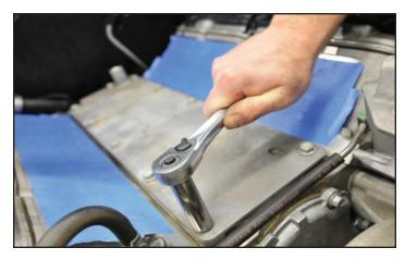
40. Remove the OEM valley cover. The valley cover gasket will be reused. Sometimes the gasket will stick to the OEM valley cover, if so, carefully remove, inspect and clean for reinstallation.
