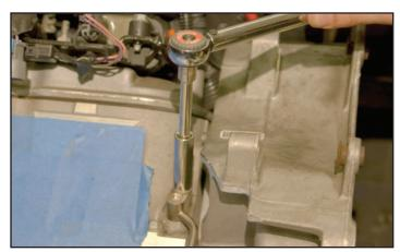
59. Remove the OEM belt tensioner assembly using a 15mm wrench.
