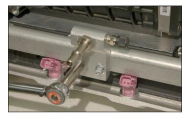
80. Snap the provided intake manifold gaskets into place on the supercharger tub.
