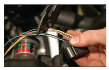
of the MAF split loom back to the junction at the main wiring harness. Route these wires over to meet the two white wires from the IAT sensor on the driver side. Using the provided crimp connectors, join the wires together. It does not matter which wire goes to which.
