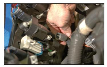
67. Unbolt the coil packs to the valve covers using a deep 10mm wrench on the five (each side) mounting bolts/studs.
