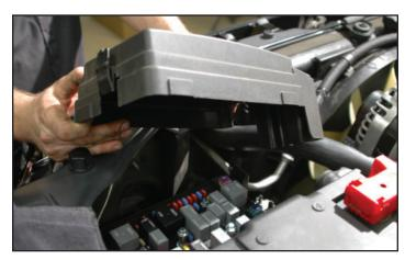
168. Remove the 15A "IGN" fuse. This fuse is in the forward bank, second fuse from the fender. Verify the fuse by name, you want a fuse that is active only when the engine is running.
