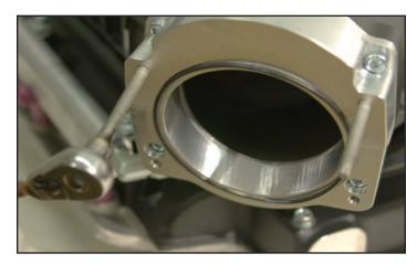
76. Ensure that the Throttle Body gasket is in place and using the original hardware, mount the OEM Throttle Body to the new supercharger inlet. Use a 10mm wrench to torque the bolts and nuts to 106 in-lbs. Verify your torque wrench settings.
