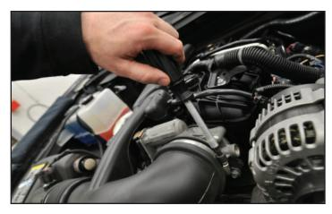
8. Use a flathead screwdriver or 8mm nut driver to remove the air tube clamps from the air box.
