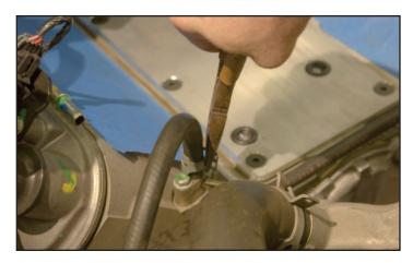
56. Use a 10mm socket wrench to remove the two coolant vent pipe bolts.
