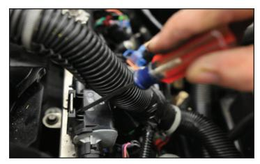
19. Pull the blue tab on the MAP sensor plug sideways to release the lock, then push down on the black tab and pull the connector off the MAP Sensor.
