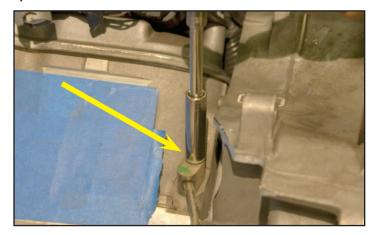
57. Remove the OEM vent pipe assembly. Make sure that the O-rings did not stick to the cylinder heads, if so, remove them.
