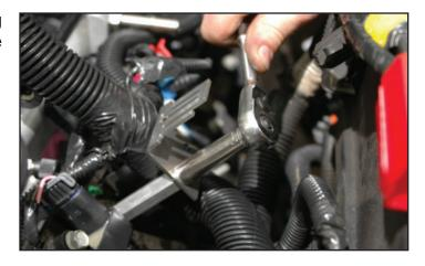
96. Install the EVAP Solenoid with the electrical connection pointing to the rear onto the just installed mounting bracket.
