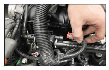
16. Disconnect the rear EVAP Solenoid hose by depressing the release clip and pulling the line free.
