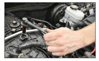
22. Remove the brake booster check valve by pulling it out of the mounting grommet.
