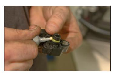
71. Use a 4mm Allen wrench to remove the MAP Sensor hold down clip behind the supercharger on the driver side. Press the lubricated MAP Sensor into the mounting hole and replace the mounting clip, tighten the clip using a 4mm Allen wrench.
