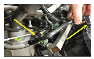
13. Unplug the Mass Air Flow sensor from the air box.
