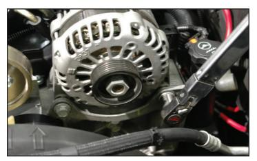
108. Connect the alternator control and hot lead wire to the alternator using the stock components.
