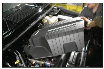
8. Using a flat blade screwdriver or an 8mm nut driver, loosen the two large hose clamps holding the air cleaner duct assembly.
