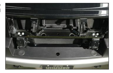
98. Here is the heat exchanger and its mounting components.
