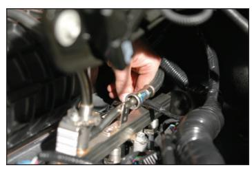
64. Attach the EVAP sensor back on the fuel rail.
