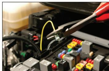
123. Remove the 10Amp HVAC IGN fuse. Check with the fuse map to verify location.
