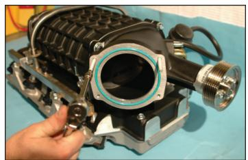
51. Install the stock throttle body removed in step 46 onto the new Supercharger housing using a 10mm socket wrench. Torque the throttle body nuts and bolts to 106 in-lbs. Verify your torque wrench settings.
