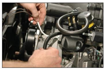
72. Locate Mass Air Flow (MAF) sensor on the airbox. Pull the split loom off a bit to expose the wires. Cut the two tan wires approximately 2" from the MAF connector.
