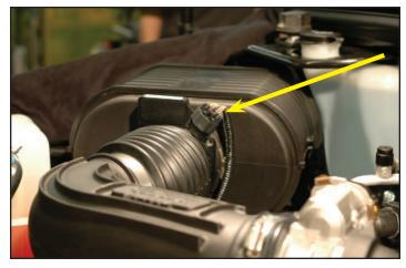
133. Cut a section of 3/8" hose provided to 8" in length. Push one end on the 90° barb installed in step 130 which is now located on the bottom of the installed air tube.
