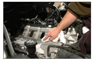
29. Cover the intake ports with tape or clean rags to keep dirt and objects from entering the engine. (Remember be clean.)
