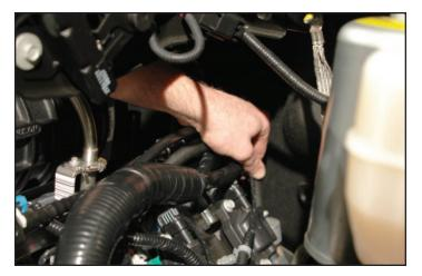
78. Route this hose forward between the coil brackets and injectors. Plug the remaining end into the front supercharger barb as shown.
