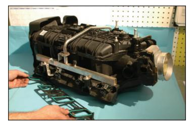
38. Install the intake manifold gaskets just removed onto the new supercharger manifold. Ensure that the gaskets are fully seated into the reliefs in the manifold.
