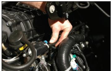
69. Locate the two IAT white wires on the driver side of the engine between the fuel rail and the Supercharger. Using the supplied white wires and shrink connectors provided, strip ½" off all ends, and crimp these wires together extending their reach.
