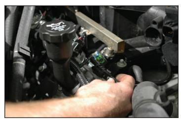
12. Disconnect the electrical connector on the throttle body.
