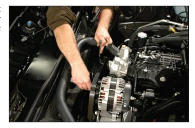
22. Using a 15mm socket wrench or standard wrench remove the two bolts holding the factory belt tensioner to the bracket and remove the tensioner. (Put tensioner and bolts aside for later use.)
