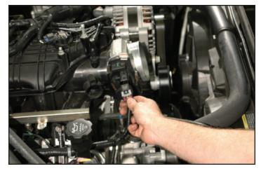
13. Using a 10mm socket wrench remove the three bolts and one nut holding the plastic wire harness retainer to the intake manifold.
