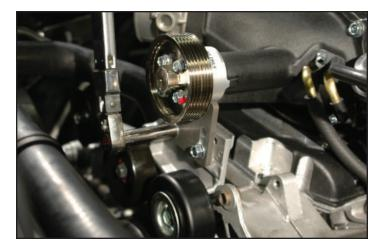
82. Remount alternator using OE hardware, torque bolts to 40 ft-lbs. Verify your torque wrench settings.
