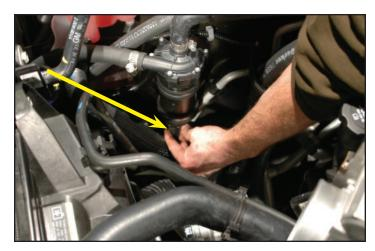
120. Remove the fuse center cover by pressing on the front lock tab and unsnap from the rear.
