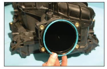
49. Install the O-ring just removed onto the new Supercharger housing as shown.
