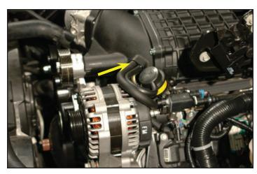
84. Re-attach the alternator battery (+) cable to the alternator post using a 10mm socket or box wrench, cover with post sock.
