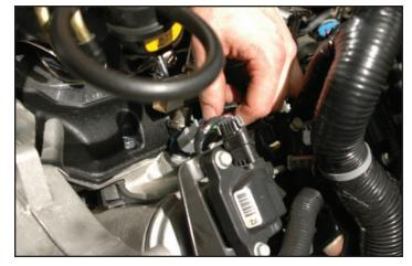
61. You will need a bit more wire for the alternator voltage sensor plug. Pull the main wiring harness split loom off the mounting stud at the front driver side valve cover. Remove about 4" of the main wiring split loom tape (1-1/2" in diameter) and pull the alternator plug wires out of the split loom about 4".
