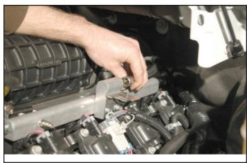
59. Replace the stainless steel safety clip that was removed in step 20. Bend the single, short tab on the EVAP bracket slightly. This will create a tight fit with the EVAP solenoid.
