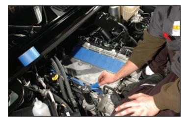
30. Remove idler pulley using a 15mm socket wrench.
