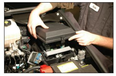
121. Route the remaining wire loom with the red and yellow wires of the intercooler relay behind the brake booster, along side the engine side edge of the fuse center, in and up at the middle of the fuse center box bottom edge, into the fuse center itself.
