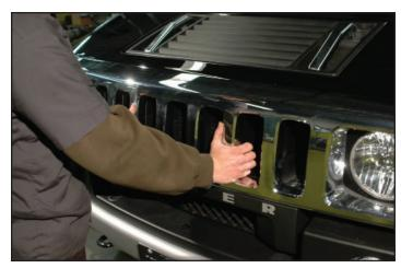
152. Replace the four (two each side) nuts at the outside of each turn signal securing the grille to the hood.
