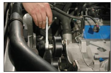
31. Use a soft hammer to disassemble the idler pulley. The parts on the right side will not be re-used; the parts on the left are required in a later step.
