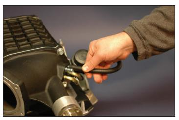
136. Carefully pull the other end of the hose off of the bypass actuator hose barb. Ensure that the brass fitting at the tip of the barb remains on the bypass actuator hose barb tube as shown.
