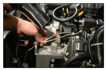
71. Cut a piece of the ¼" split loom provided to cover these wires plus about 12". Tuck the wires inside leaving the ends exposed through the side of the split loom and route the split loom under the Supercharger nose toward the passenger side of the vehicle.
