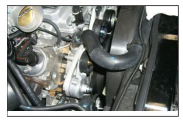
34. Replace the Idler pulley removed in step 30 onto the new bracket support assembly. See step 31 for parts required.
