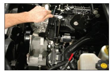
26. Carefully remove the intake manifold assembly and set aside.
