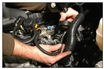
63. Route the MAP sensor wires between the fuel line and fuel rail, then plug into the Map sensor at the driver side rear of the Supercharger manifold lid.
