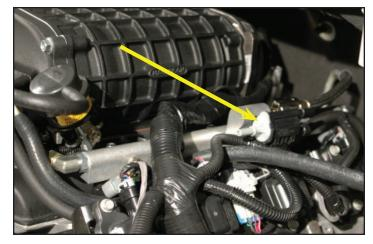
65. Plug the EVAP sensor wires back on the EVAP sensor. **NOTE: The plug should be toward the firewall.**
