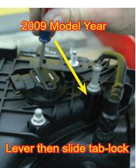
40. The clip can now be removed, now carefully lift the sensor out. (Make sure that the MAP sensor seal does not get damaged, as it will be reused.)
