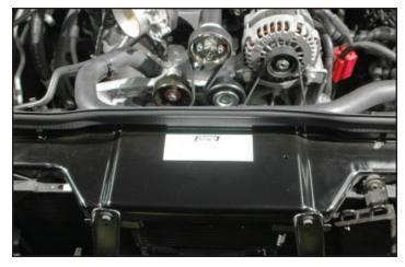
89. Attach the reservoir mounting bracket to the reservoir with the three supplied bolts. Mount the reservoir to the middle-passenger-side fuel rail mounting post using the provided bolt and 1/2" spacer below the mounting bracket, and torque back to 106 in-lbs. Verify your torque wrench settings!
