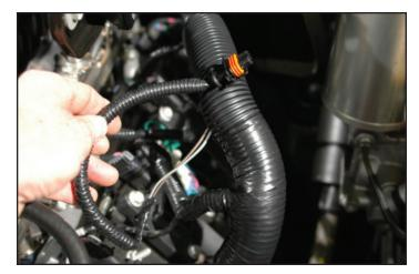
62. Cover the Alternator plug wires with the provided ¼" split loom and re-tape the new and existing split loom.
