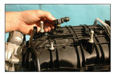
41. For 2009+ MAP sensor skip to step #42. If you have the 99-08 style MAP sensor you will need to install the provided bushing. YOU MUST install the bushing with sealant to prevent a vacuum leak. We recommend black silicone RTV or green Loctite 680. Be sure to wipe off any excess sealant inside the bushing. Allow sealant to cure before starting engine.
