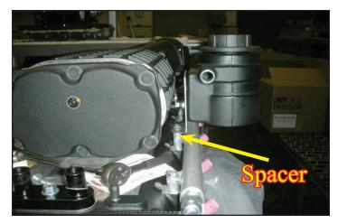
90. On the front end of the passenger-side wheel well in the engine compartment: Drill two ¼" holes. Using the existing hole for the plastic wiring loom clamp as a guide (removed in this photo), go forward 1-1/4" then down 2". Drill your first hole here. Go down from that hole an additional 2-1/4" and drill your second hole.
