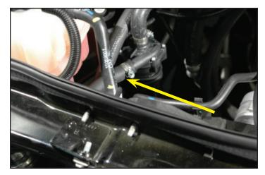
110. The other end of the 90" hose installed in step 106 is routed to the supercharger inlet barb located on the driver side, rear of the supercharger manifold. Tighten the #10 clamp firmly.
