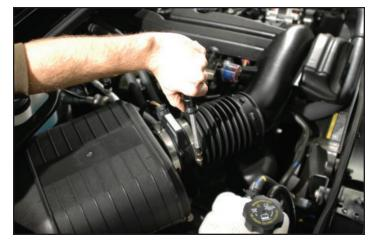
Pull the PCV valve cover hose on the passenger side of the vehicle free from the airduct assembly.
