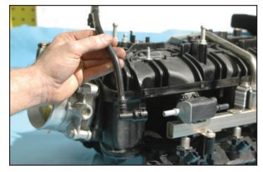
45. Remove the EVAP sensor from the fuel rail by depressing the release tab and lift the sensor free.
