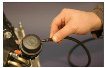
139. Route the hose back along the supercharger to the rear of the supercharger on the passenger side. Remove the existing cap from the hose barb as shown.
