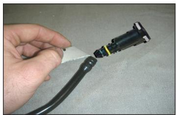
67. Cut a section of the supplied 3/8" hose to 11" in length. Install the factory fittings removed in the previous step onto the ends.
