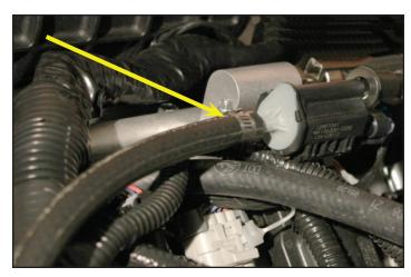
80. If not done in step 65, plug in the electrical connection to the EVAP Solenoid.
