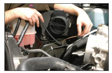
74. Using the new Intake Air Temp (IAT) wires you just extended and crimp/shrink connectors supplied, connect the extended wires to the tan wires you separated that run through the harness to the vehicles computer. The ends of the wires to the MAF plug will be abandoned. Strip about ¼" of insulation from the ends of the tan wires to the computer and the extended white wires. Crimp the connectors on.
