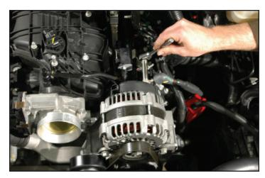
24. With a 15mm socket wrench remove the two bolts holding the alternator to the alternator bracket. Remove the alternator.
