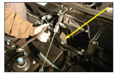
113. Replace the plastic push pin rivet holding the deflector in position.
