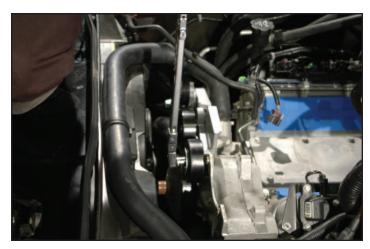
36. Carefully cut out & remove cable guide/mount that was mounted on top of intake.
