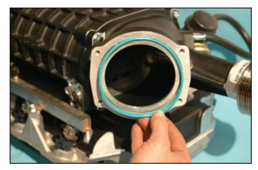
50. Install the two throttle body mounting studs removed in step 47 onto the Supercharger housing as shown using an E5 inverted Torx socket.
