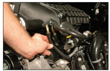
79. Cut a piece of the provided 3/8" hose to 16-1/2" in length. Attach and clamp one end to the front barb on the EVAP Solenoid.
