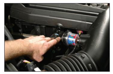
10. Remove the duct assembly by lifting it out.
