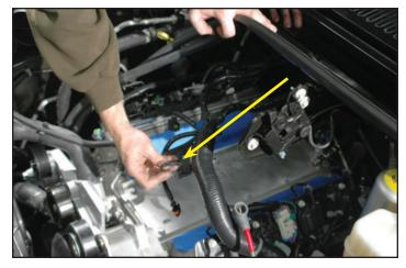
37. Remove the OEM intake manifold gaskets from the base of the stock intake manifold.
