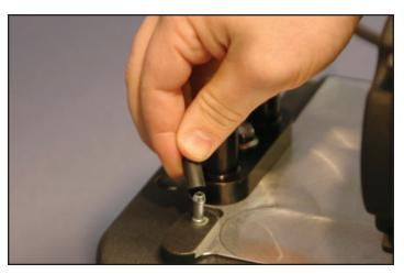
140. Plug the remaining end of the new bypass actuator hose onto the hose barb you just exposed.
