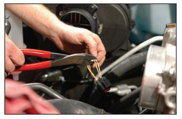
73. Remove the tape to the junction at the wire harness, and pull the two tan wires from this flex loom back to the next junction in the wire harness.
