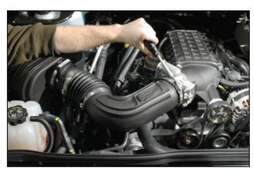
132. Plug in the MAF sensor at the air box.
