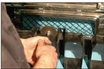
147. You need to place a piece of tape on the inside of the cells to be cut to create a visible line to follow. Use a straight edge slid between the top and bottom cuts you just made and draw a line as shown. Now take the cutting wheel (or hack saw blade, Dremmel etc.) and connect the top and bottom cuts to remove the pieces.
