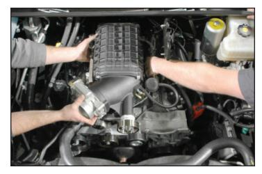
54. Start all ten fasteners by hand to ensure proper lineup. Torque all ten fasteners in a criss-cross pattern to 106 in-lbs.
