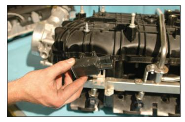
46. Use a 10mm socket wrench to remove the stock throttle body from the stock intake manifold.
