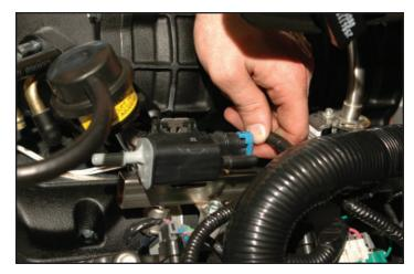
66. Carefully cut the fittings off of the EVAP hose removed in step #18. Be careful to not damage the fittings.
