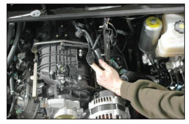
17. Unplug the EVAP solenoid electrical connection.
