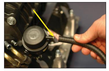
137. Press the supplied barb cap onto the hose barb of the supercharger inlet where you removed the bypass hose.
