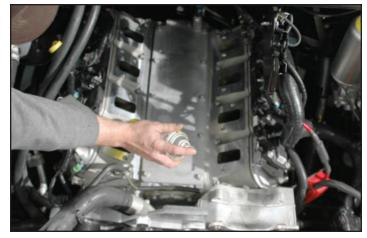
53. Using an assistant, carefully lower your new Supercharger manifold assembly into place.
