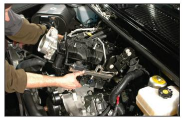
27. Using a vacuum cleaner, remove any dirt or debris from the intake port area. Be careful not to get any dirt in the intake ports.
