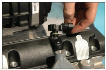
43. Using a 4mm Allen wrench, install the MAP sensor retaining clip with the provided 6mm button head screw as shown.
