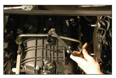
20. Release the fuel line safety clip, and with the fuel line disconnect tool (included in kit), remove the fuel lines from the fuel rail. Be careful, the system may still be under pressure. Use shop rag under the connections to catch any fuel spills. Dispose of shop rags appropriately. Stay away from sparks and flames (Remember fuel is highly flammable).
