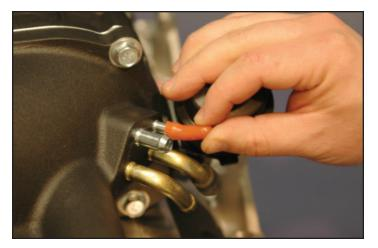
138. Install the new provided bypass hose onto the bypass actuator vacuum hose barb where the hose was removed.
