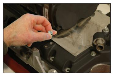
42. Apply a bead of the supplied Lubriplate lubricant to the MAP sensor seal and press the MAP sensor into the provided hole in the supercharger manifold as shown.
