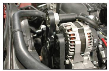
87. Press the supplied sliding idler pulley down to its tightest position and torque to 40 ft-lbs. Using the 15mm tensioner or breaker bar, release the tensioner and remove the retaining pin placing tension on the drive belt. Drive belt is a Gates #K061098.
