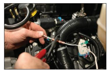
70. Use a heat gun or hair dryer set on high, shrink the insulation on the connectors so that it contracts around the wires completely. You MUST shrink the insulation, as crimping the connectors alone is NOT enough to secure them.
