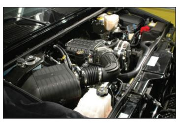
156. Test drive vehicle for the first few miles under normal driving conditions. Do not perform any wide open throttle runs. Listen for any noises, vibrations, engine misfire or anything that does not seem normal. The supercharger does have a slight whining noise under boost conditions, which is normal. Check & bleed intercooler reservoir as needed.
