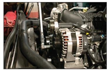
83. Connect the remaining end of the front EVAP Solenoid hose attached in step 79 onto the inlet barb of the supercharger as shown.
