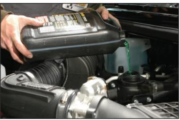
155. Start the vehicle for five seconds and shut off. Once again, check for fuel leaks, fansupercharger belt alignment, radiator, and intercooler reservoir. Top off as necessary
