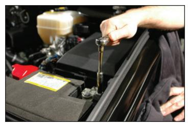
7. Remove the plastic sight shield by lifting from the front and pulling free from the engine, this will not be reused.
