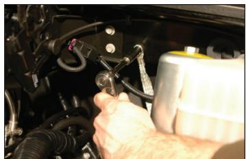
115. Align the two plastic connection boxes of the intercooler relay as shown. Use a ¼" drill to create two enjoined mounting holes.
