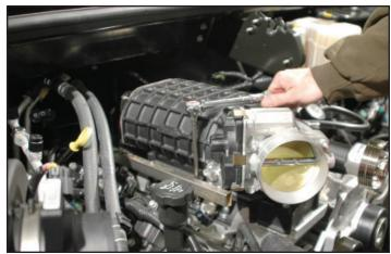
55. Assemble the EVAP solenoid bracket and bolts onto the fuel manifold.
