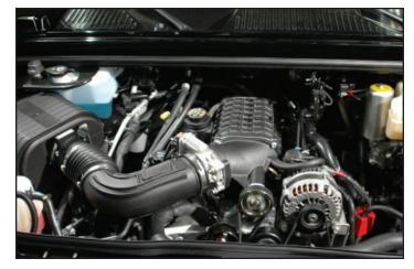
157. After the initial test drive gradually work the vehicle to wide open throttle runs, listen for any engine detonation (pinging). If engine detonation is present let up on the throttle immediately. Most detonation causes are low octane gasoline still in the tank. Affix the Premium Fuel Only decal on the inside of the fuel fill door.
