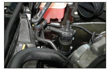
93. Replace the wire loom clamp and re-attach the wire loom.
