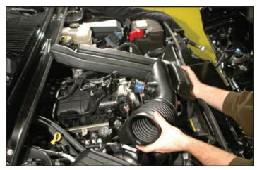
11. Rotate the rigid PCV hose just disconnected toward the driver side of the vehicle (appx. 90°) to expose the retaining clip release tab. Press the tab clockwise (as seen from the front of the vehicle) to release. Pull the hose from the passenger side valve cover barb, this hose will not be reused.
