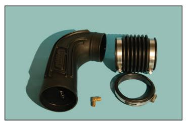
130. Use some Teflon sealer or Teflon tape to coat/wrap the threads of the brass 90° fitting. Install the fitting in the air tube threaded hole with the barb pointing at approximately 2:00 from a bottom view, as shown in this picture.
