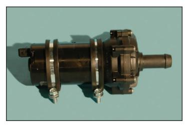
92. Push the bolts of the Adel clamps through the fender well and finger the nuts on. Make sure the pump discharge barb is just above the hose from the water pump to the radiator overflow reservoir. Tighten the bolts.
