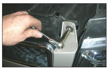
154. Carefully replace the front fascia and using a 10mm socket wrench, replace the six bolts that secure the front fascia to the radiator support.
