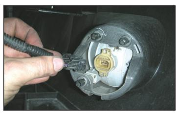
126. With the wheel well loose, pull back on the wheel well, giving you access to the fog lamps. Disconnect the electrical connector from the lamp. Repeat on the other side of the vehicle.
