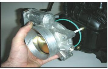
56. Using a 10mm socket wrench, remove the stock throttle body from the OEM intake manifold. Next, using a #5 internal Torx, remove the two mounting studs from the stock manifold.
