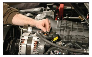
96. Plug in the Electric-Voltage sensor wire into the Alternator connector as shown.
