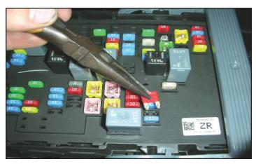
110. Remove the 10amp mini-fuse in the fuse box that labeled HVAC-IGN. **NOTE:** Fuse location may vary, verify by fuse name!
