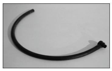
82. Cut a section of the provided 11/32" brake hose to 26" in length. Install the stock check valve on one end, and plug the check valve into the brake booster.
