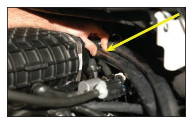
148. Cut 1" of the short end of the 4 x 60x ¾" 90° molded hose supplied and connect the short end to the remaining supercharger barb (it should be the one closest to the driver side of the vehicle) and secure it with a #10 clamp provided.
