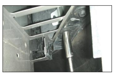
127. After unplugging the fog lamps, remove the two bolts with a 10mm socket wrench that secure the fascia to its support frame. Also remove the two bolts that secure the lower front fascia to its support brackets.
