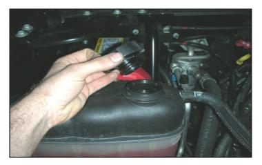
11. With a cool engine remove the radiator cap. (Be careful not to remove the cap if the engine is still hot.)
