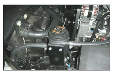
160. Refill radiator and intercooler system with vehicle manufacturer recommended coolant mixture. Let run for 5-10 minutes. Bleed system at reservoir. Check system periodically for fluid level.
