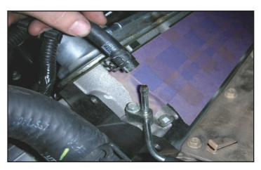
34. Remove the coolant hose from the vent pipe.
