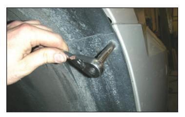
125. Using a 7mm socket wrench and a flat blade screwdriver, remove the two bolts and the two plastic pushpins that secure the inner wheel well to the front fascia.
