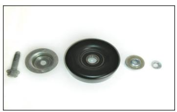
70. Using a soft hammer, knock the factory bolt loose from the idler pulley. The bolt retainer and stand-off (pictured here on the right side of the pulley), will not be re-used. Note: The bolt, dust cover and idler will mount to new tensioner bracket.
