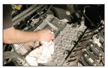
39. Clean off the receiving end of the heads using a suitable non petroleum based solvent (alcohol, acetone, etc) to remove any residue.
