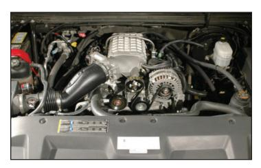
161. Start the vehicle for 5 seconds and shut off, once again check for fuel leaks and fansupercharger belt alignment. Check radiator and intercooler reservoir.
