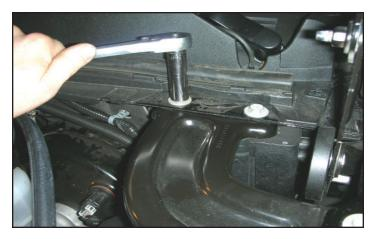
120. Re-install the fender to the firewall brace.
