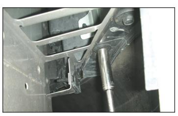
155. Replace the two bolts to secure the fascia to its support frame using a 10mm socket wrench. Also replace the two bolts that secure the lower front fascia to its support brackets.
