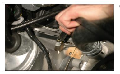
64. Install the supplied steam vent hose and secure using the OEM hose clamp.
