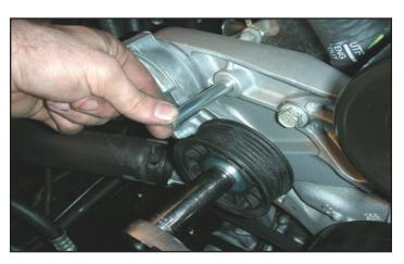
97. Use a 15mm socket wrench to lever the tensioner all the way down, then insert the pin provided into existing hole on the tensioner bracket to hold the tensioner in the compressed position.
