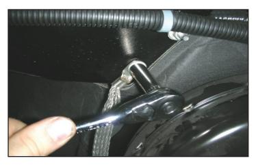
117. With a 10mm socket wrench, remove the nut securing the ground cable to the firewall.
