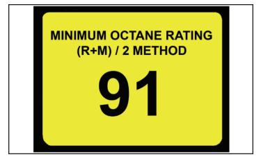
Your system requires the use of minimum 91 Octane gasoline fuel. This system is not compatible with E85 fuel.
