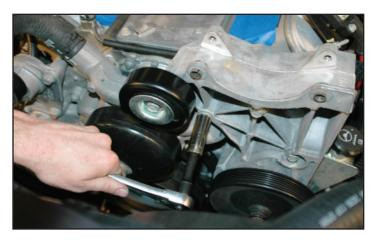
47. To make installation of the supercharger manifold easier, remove the alternator/power steering bracket from the engine block. Using a 15mm socket wrench, remove the four bolts on the front side and the one bolt on the lower driver-side.
