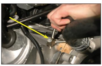
63. Install the supplied vent pipe using the stock hardware, torque to 106 in-lbs. **Note: Verify your torque wrench settings.**
