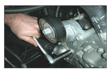
42. With a 15mm socket wrench, remove the three bolts that hold the tensioner to the water pump and remove the tensioner. Notes: The tensioner won't be re-used, but one long stock bolt, and the short stock bolt will be re-used. \*Some 08-and up tensioners only have the two long bolts. We will still use one of those and will supply a new bolt to take the place of the short stock bolt that wasn't installed originally.
