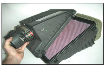
102. Re-install the air box lid and then install the air box assembly back into the vehicle.
