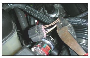
65. Locate the MAF electrical plug, pull back the flex loom about 12", and cut the tan wire and the tan w/black stripe wire about 2" from the MAF connector.
