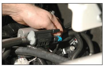
90. Plug in the electrical connection to the EVAP Solenoid.
