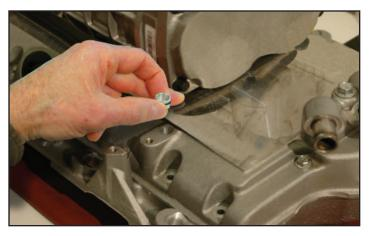
49. For 2009+ MAP sensor, skip ahead three steps. If you have the 99-08 style MAP sensor you will need to install the provided bushing. YOU MUST install the bushing with sealant to prevent a vacuum leak. We recommend black silicone RTV or green Loctite 680. Be sure to wipe off any excess sealant inside the bushing. Allow sealant to cure before starting engine.
