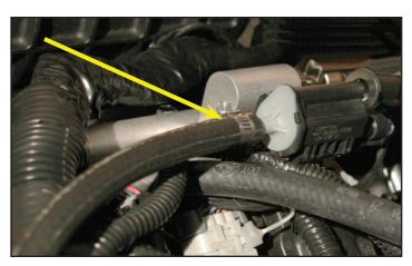
89. Cut a piece of the provided 3/8" hose to 16-1/2". Attach and clamp one end to the front barb on the EVAP solenoid.
