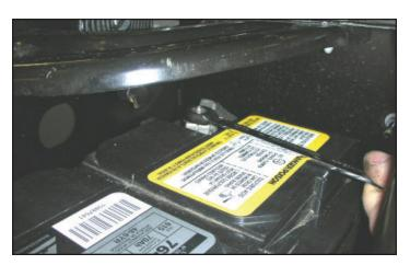
159. Re-connect the battery with a 10mm socket wrench.
