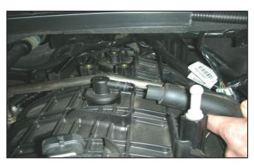
24. Next, remove the PCV hose from the top of the intake. Also, remove the other end of the hose from the rear of the valve cover. This will not be re-used. NOTE: On 2009 and up model year vehicles, this connector has changed. To remove, first the clip connector on the valve cover needs to be released and disconnected. Then rotate the entire assembly clockwise 90° (looking down on the intake manifold) then pull up as the twist lock is released.
