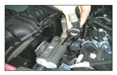
22. Remove the EVAP line from the solenoid by pressing in the gray retainer clip and pulling the line off of the solenoid. Repeat procedure for removing the other end of this line. Your vehicle may not have the test port (the green cap) shown in this picture.
