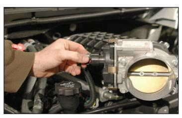
79. Plug the electrical connector for the ETC back into the throttle body.
