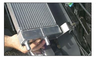
141. Install the heat exchanger onto the studs of the rubber mounts and secure it with the nuts supplied and a 10mm socket wrench.
