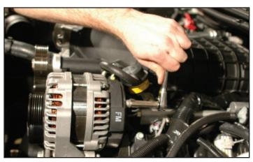
94. Ensuring that the battery is still disconnected, connect the battery positive (+) cable you routed six steps ago to the back of the alternator and secure the nut with a 10mm socket wrench.
