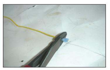
113. With the relay mounted, take the yellow trigger wire from the relay, strip about 1/4" of the insulation from the end and crimp it onto the supplied spade connector.
