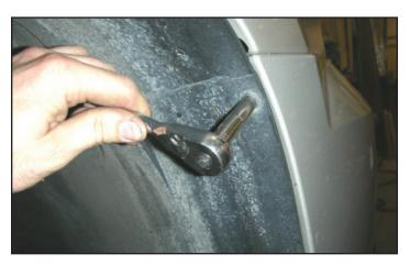
157. Using a 7mm socket wrench, replace the two bolts and the two plastic pushpins that secure the inner wheel well to the front fascia.
