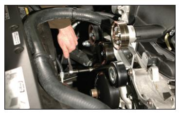
72. Install the tensioner assembly into the vehicle as shown.
