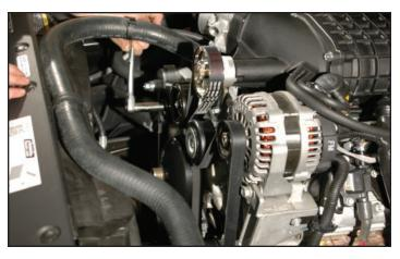
98. Using the belt routing diagram as a guide install the new belt provided. Slide the idler pulley down and torque to 40 ft-lbs using a 15mm socket wrench. Verify your torque wrench settings. Finally remove the pin and release the tensioner. Make sure the belt contacts all pulleys correctly.
