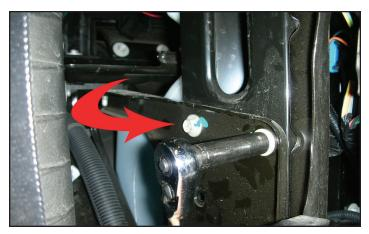
130. Using a 10mm socket wrench, remove the bolt shown, this is behind the drivers' side headlight, and is bolted to the radiator support.
