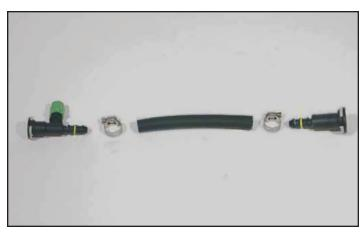
86. Cut a section of the 3/8"hose to 11" in length. Install the factory fittings removed in the previous step onto the ends.
