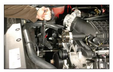
73. Torque all the bolts to 40 ft-lbs with a 15mm socket wrench. Verify your torque wrench settings.
