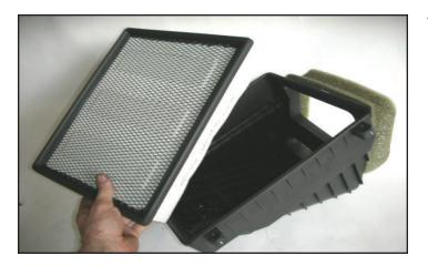
100. Remove the stock air filter from the air box.
