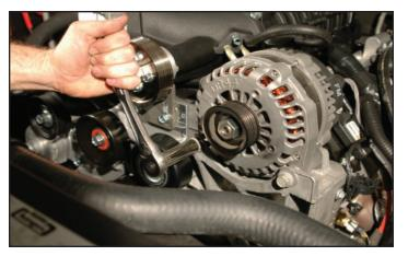
92. Next, re-install the alternator using the factory hardware.
