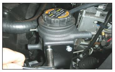
124. Mount the intercooler reservoir tank to the bracket using the three M6 X 12mm bolts. Tighten the bolts using a 10mm socket wrench.
