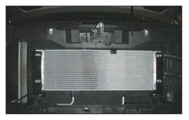
144. Here is the heat exchanger mounted. Note: The hose barbs are on the driver side.
