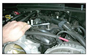
16. Remove the wiring harness bracket from the intake manifold by removing the nut with a 10mm socket wrench.
