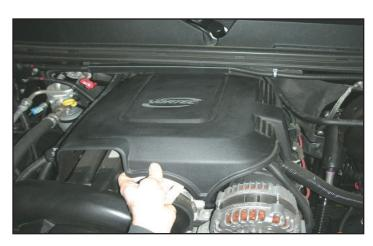
6. Remove the plastic engine cover by lifting up at the front and pulling the cover forward. This cover will not be re-used.
