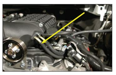
84. Cut a section of the provided 3/8" hose to 25" in length. Plug one end into the PCV barb at the back of the driver-side valve cover. Route the other end under the coil bracket and plug into the hose barb on the supercharger as shown.
