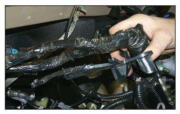
76. Remove the wiring harness from the original bracket.
