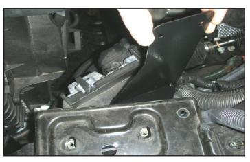
122. Lift up on the secondary battery tray and slide the intercooler reservoir tank bracket under the tray, lining up the holes on the bracket with the holes on the tray.
