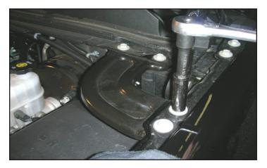
108. Remove the driver side fender to firewall brace with a 13mm socket wrench, to gain access to the fuse relay panel.
