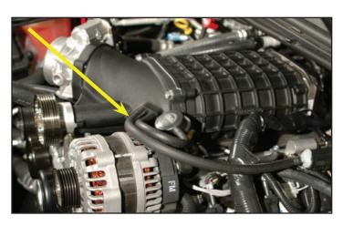
95. Route the front hose from the EVAP Solenoid to parallel the Bypass Valve hose and connect to the remaining barb on the supercharger nose.
