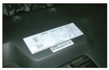
158. Place the belt/vacuum routing diagram onto the radiator support cover.
