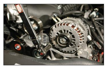
93. Using a 15mm socket wrench torque the two bolts to 40 ft-lbs. Verify that your torque wrench is set to ft-lbs.
