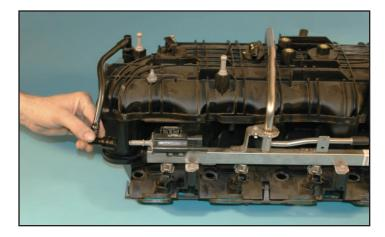
52. Disconnect the short EVAP pipe from the EVAP Solenoid on the stock intake manifold.
