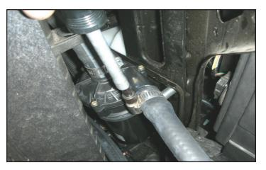
152. Using the last of the remaining 3/4" hose, attach one end to the outlet barb on to the intercooler pump.
