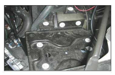
123. Using a 10mm socket wrench, re-install all bolts that were removed.
