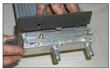
138. Align the bolts with the holes in the bracket.
