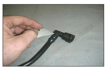
85. Take the rear EVAP hose from the stock manifold and carefully cut out the fittings at the ends of the hose.
