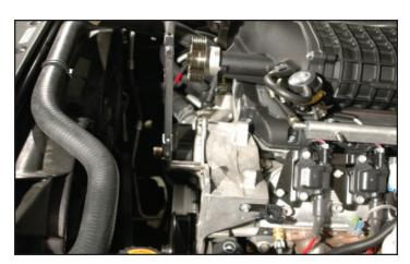
68. Re-installed the alternator/power steering bracket with all the factory hardware and torque to 40 ft-lbs with a 15mm socket wrench. Verify your torque wrench settings.
