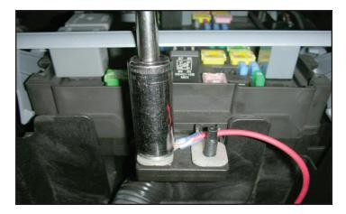
116. Using a 12mm socket wrench, and the nut provided, secure the fused red wire to the M8 stud.
