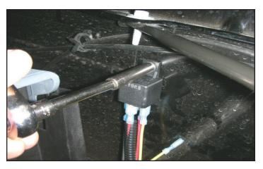
112. The intercooler relay harness is going to mount on the driver side inner fender just below where the fender support bracket is mounted. Use the self-tapping screw supplied to drill a hole, then use the screw to mount relay to fender.
