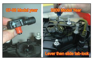
48. Remove the stock MAP sensor by removing the retaining clip with a screwdriver and then gently pulling up the sensor. Be careful not to damage the O-ring seal. NOTE: On 2009 model year this connector may have changed. To remove, insert a small screwdriver into the slot opposite the slide-tab lock. Lever the locking tab outward to release the lock, then slide the lock to remove.
