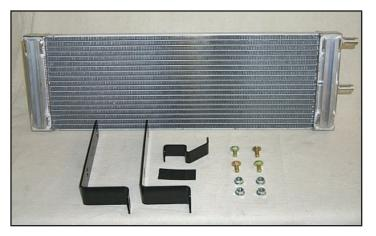
136. Here is the intercooler and its mounting components.
