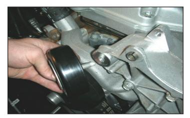
69. Using a 15mm socket wrench, remove the factory idler pulley.
