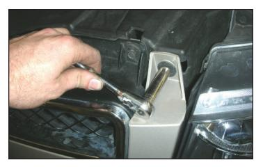
128. Using a 10mm socket wrench, remove the six bolts that secure the front fascia to the radiator support.
