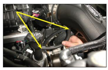
107. Attach the remaining 3/8" hose (left over from a previous step-about 9") from the right (passenger-side) valve cover to the barb on the bottom of the air tube.
