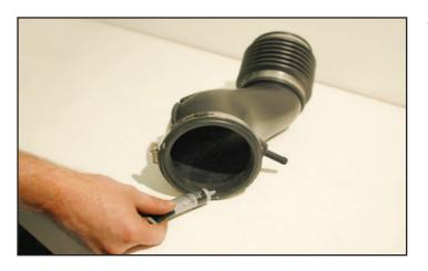
105. Using some of the O-ring grease supplied, apply a light coating of grease on the inside of the coupler.
