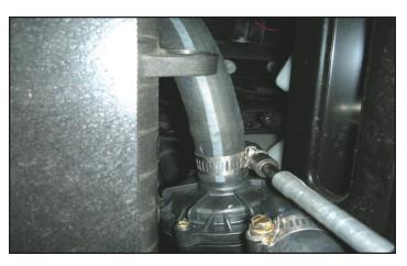
151. This hose will route directly to the inlet barb on the intercooler pump. Trim to fit, and secure the hose with the supplied #10 clamp. Note: Clamps may vary between squeeze style and screw style.
