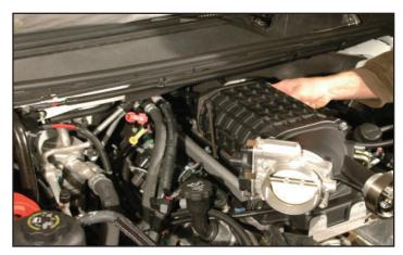
61. Insert the ten intake manifold bolts into position through the stand-off plates. Finger-tighten at this time ensuring complete alignment.
