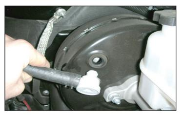
23. Remove the power brake hose and check valve from the booster. This hose will not be reused, but keep the check valve as you will be using it in a later step. Note: If vehicle is equipped with hydra-boost then the vehicle will not have this hose.
