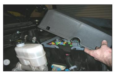
109. Pull back on the two tabs holding the fuse cover to the fuse box and lift the cover out of the vehicle.
