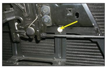
142. Remove the bolt located below and to the right of the hood latch with a 10mm socket wrench.
