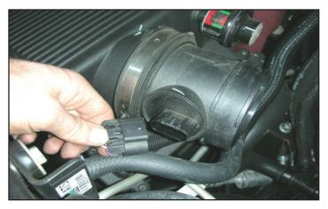
13. Unplug the electrical connector from the MAF sensor. NOTE: On 2009 and up model year vehicles, this sensor is located on the top surface, not the front surface shown in this picture, and the connection points toward the rear of the vehicle.
