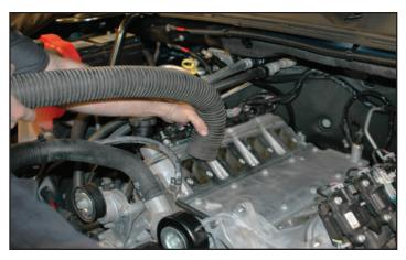
33. Using a vacuum cleaner remove any dirt of debris from the intake port area. Then tape over the intake ports. CAUTION! Be careful not to get any debris down the intake ports.
