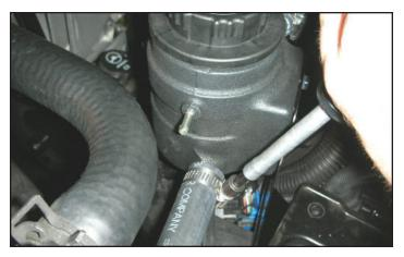
150. Put a piece of the remaining hose onto the other 3/4" barb (lower) on the intercooler reservoir and secure with a #10 clamp provided. Make sure you are using the supplied worm gear clamp.
