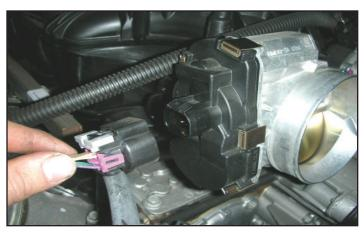
17. Disconnect all electrical and hose connection from the intake manifold. Start by unplugging the ETC connector from the throttle body.
