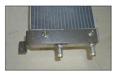
139. Torque the mounting nuts to 18 ft-lbs. Verify your torque wrench settings!
