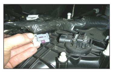
19. Disconnect the electrical plug from the MAP sensor located on the top of the intake manifold at the front. NOTE: On 2009 and up model year vehicles, this connector looks a little different. Disconnect by pressing down on the release tab on the top of the connector and pull free from the MAP sensor.
