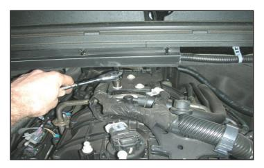
15. Using a 10mm socket wrench, remove the three bolts that secure engine cover support bracket to the intake manifold. This will not be re-used.
