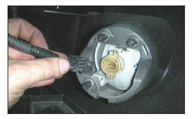
156. Plug the fog lamps back in on both sides of the vehicle.
