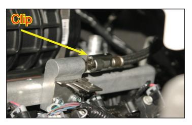
75. Replace the stainless steel safety clip that was removed earlier. NOTE: For 2007-2010 vehicles, you will use the EVAP bracket shown here, attached to the fuel manifold. Bend the single short tab down slightly to crate a tight fit with the EVAP solenoid. 2011 + vehicles use a flat EVAP bracket mounted further up on the fuel rail. Inspect factory fuel line for kinks or tight bends in braided section. If required push gently on fuel line near firewall to eliminate kinks/slight bends.
