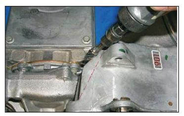
43. It will be necessary to make clearance on the alternator mount casting for the new manifold to fit properly. The new manifold should not touch the alternator mount. These modifications can be easily done with the mount in place.
