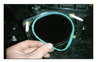
57. Remove the stock throttle body O-ring from the OEM stock manifold. Clean off any oil before installing the O-ring onto the supercharger inlet.
