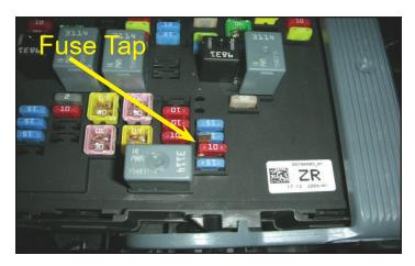
Install the supplied fuse t-tap onto the fuse and re-install the fuse back into the fuse box.
