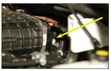
146. There are two ¾" hose barbs at the rear of the supercharger. Starting at the intercooler barb on the passenger side of the supercharger, take the supplied 4 x 36 x ¾" 90° molded hose and clamp the hose onto the intercooler barb using a #10 clamp. Run the hose forward toward the IC reservoir on the driver side of the radiator.
