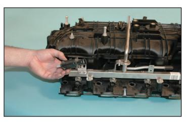
53. Remove the stock EVAP solenoid from the stock manifold by lifting up to free the unit from the mounting bracket.
