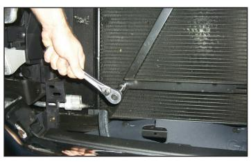
134. For model year 07-08 vehicles near the base of the fascia "A-Frame" support in front of the radiator is a bolted connection. Remove the two bolts at the base of the "A-Frame".
