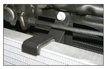
143. Install the upper mounting clamp onto the heat exchanger core using the bolt removed in the previous step. Tighten the bolt securely.
