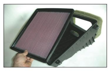
101. Take the new K&N air filter supplied in the kit, and install it into the air box.
