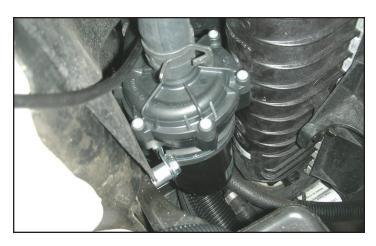
131. Locate the Adel clamp, and put it on the intercooler pump, then using the 6mm x 55mm bolt and the spacer supplied install the intercooler pump to the radiator support.
