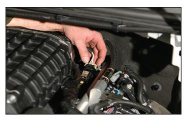
80. The MAP sensor can also be plugged back in. Sensor location is now at the rear of the manifold and no wire extensions are necessary.
