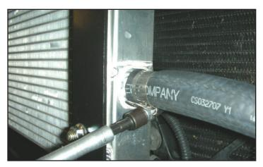
149. Route the hose that was just installed (in the previous step) through the radiator support and under the intercooler pump and connect it to the lower barb on the heat exchanger and secure it with the #10 clamp provided. Cut and install a section of the supplied split loom to protect the hose from chaffing at the radiator support.
