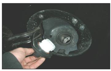
5. To relieve fuel pressure in the tank, remove the fuel cap.
