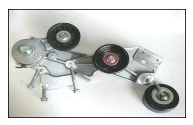
71. Here is the tensioner assembly showing where the specific bolts and where the factory idler goes.
