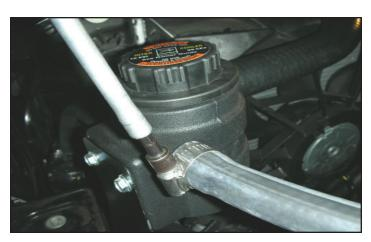
147. Route the hose just connected to the intercooler reservoir tank. Trim the hose to fit, connect it to the intercooler reservoir tank upper 3/4" hose barb. Make sure you are using the supplied worm gear clamp on the reservoir.
