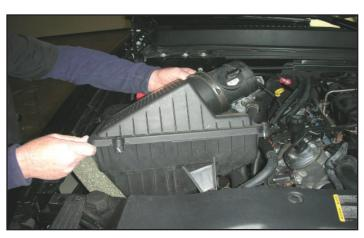
14. Firmly grasp the air intake box and pull up, removing it from the vehicle. The air box will be re-installed in a later step.
