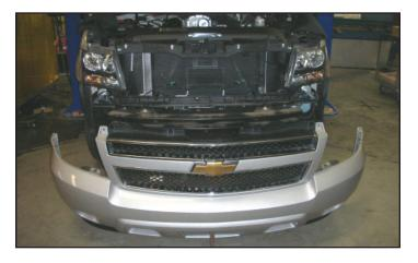
129. With the help of an assistant, carefully remove the front fascia and set aside where it will not be damaged.
