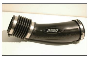
104. Assemble the bellows and coupler to the air tube. Note: The position of the clamp screws. The screws must be facing up so that you can install the assembly on the vehicle.
