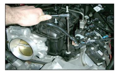
31. The intake manifold is now ready to be removed. Using an 8mm socket wrench, remove the ten bolts that secure the manifold to the engine.
