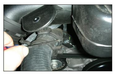
8. Disconnect the loom clamp from the upper radiator hose using a small flat blade screwdriver.
