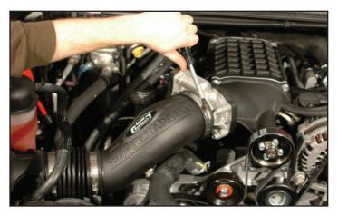
106. Push the bellows end of the air tube assembly on to the air box first, and then install the remaining end with the coupler on to the throttle body. Tighten all clamp screws securely.
