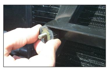
135. Mount the rubber shock-mounts supplied in the exposed holes. Tighten the mounts securely by hand only. For 09-10 vehicles, put two of the supplied washers between the shock-mount and cross member. Use the supplied nuts on the back of the cross-member.
