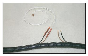
66. Cut the supplied white wire into two equal lengths and strip about ½" off all ends. Strip about 1/4" of insulation from the ends of the tan and the tan/black wires to the computer and the IAT white wires. Using the crimp/shrink connectors supplied, connect one white wire to the tan wire and the other white wire to the tan wire with black stripe that runs to the vehicles computer. The severed ends of the wires that run to the MAF will no longer be used.
