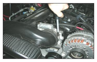
7. Using an 8mm nut driver or a flat blade screwdriver, loosen the two clamps, one at the throttle body and one at the MAF sensor.
