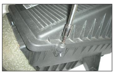
99. Using a T-25 Torx socket, remove the four screws that attach the air box lid to the lower half of the air box.
