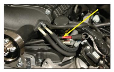
88. Route the battery positive (+) cable below the supercharger nose, behind the brake and PCV hose for later connection to the alternator.
