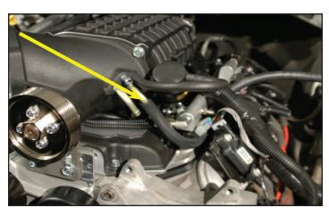
83. Route the other end under the coil bracket to the supercharger nose, and plug into the supercharger barb as shown.
