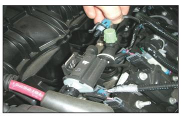
21. With the wiring harness out of the way, unplug the EVAP electrical connector from the solenoid.
