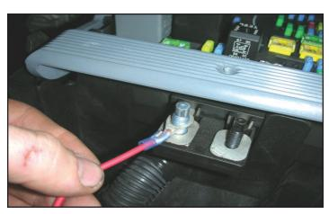
115. Next, take the fused red wire and cut off the 6mm eyelet connector and replace it with the supplied 8mm eyelet connector and install the wire onto the M8 stud in the fuse center.
