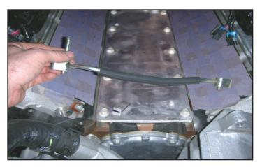
35. Remove the two bolts that secure the coolant vent pipe to the cylinder heads and remove the vent pipe from the engine, put aside for later re-installation. It's a good idea to put a piece of tape over all openings to avoid debris contamination.
