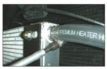
153. Finally route the hose to the upper barb on the driver-side of the LTR, secure with provided #10 clamp, and tighten. Cut and install a piece of the supplied split loom to protect this hose from chaffing at the radiator support.
