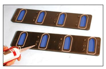
38. Put tape over the upper mating surface ports. Flip back over to the grommet-gasket side of the stand-off plates. Place a few dabs of black RTV adhesive on each of the assembled stand-off plates, splitting the bolt holes as shown.
