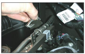
25. Remove the stainless steel safety clip from the fuel line. Do not discard. This will be reinstalled later on.
