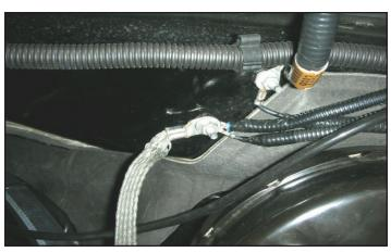
118. Crimp the supplied 6mm eyelet connector onto the ground (black wire) wire from the intercooler relay, install it onto the ground stud and re-install the factory nut.
