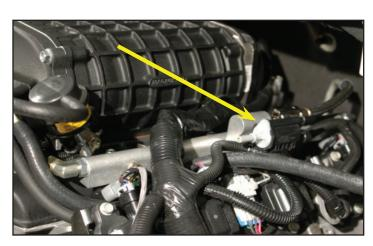
87. Install the OEM EVAP Solenoid on the mounting bracket on the driver side fuel rail manifold.
