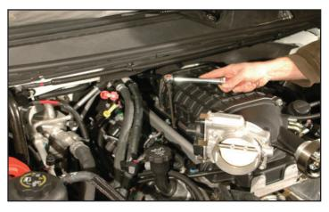
62. Using a rotating pattern tighten all ten intake manifold bolts. Torque all ten bolts gradually and evenly to a torque of 106 in-lbs. Note:
