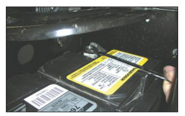
4. Disconnect the negative (-) lead of the battery cable. Cap or cover the terminal to protect against accidental contact with the battery post.
