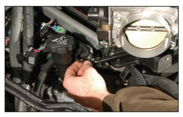
78. Remove the plastic loom clip from the wirelooms located next to the oil filler neck with a flat blade screwdriver.
