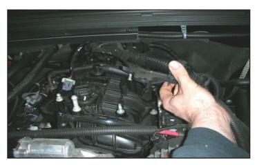
20. Now that all the electrical connections are free from the manifold, move the wiring harness out of the way by moving them over to the driver side of the engine compartment.
