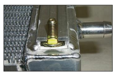
137. Install two of the round-headed carriage bolts supplied into both channels on the sides of the heat exchanger. The square portion of the bolt shaft must be aligned with the side of the channel.
