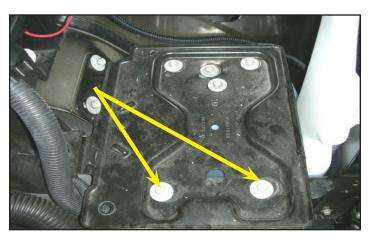
121. To install the intercooler reservoir tank bracket you must remove these two bolts, using a 10mm socket wrench.
