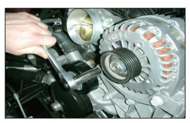
30. Using a 15mm socket wrench, remove the two bolts securing the alternator to the bracket and remove the alternator from the vehicle. This will be re-installed later on.
