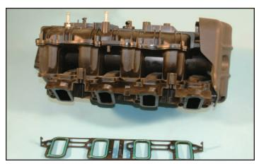
54. Remove the stock intake manifold gaskets from the OEM intake manifold.
