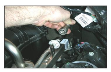
26. CAUTION! Always wear safety glasses when working with fuel. Continue on with the next three steps ensuring that the negative (-) battery cable is still disconnected. Using the fuel disconnect tool provided, remove the fuel line from the fuel rail. CAUTION! Fuel system may be under pressure. Avoid open flames or any source of ignition.
