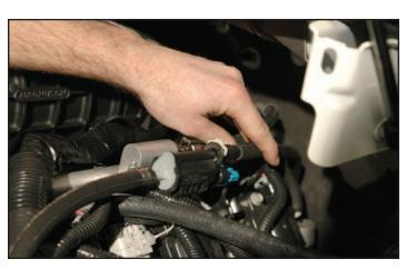
91. Plug in the end of the hose assembled five steps ago to the remaining (rear) barb on the EVAP Solenoid. Plug the other end onto the barb at the driver side rear of the engine from whence it was removed.
