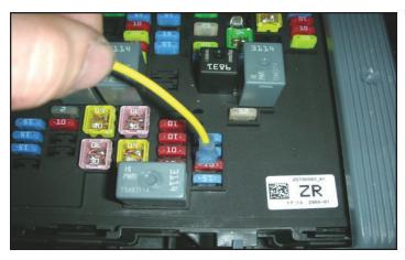
114. Take the yellow wire from the intercooler relay and connect the spade terminal end and install the wire onto the fuse tap installed earlier. (HVAC IGN)
