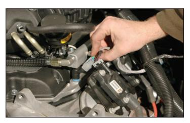
77. Take the eight fuel injector plugs and connect them to the eight fuel injectors. Note: Make sure that the connectors are seated on the injector and locked in place. Pull the harness connector to ensure a good contact.
