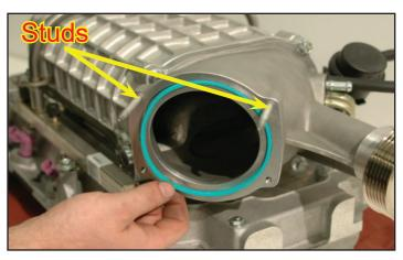
58. Install the two studs from the previous step into the supercharger intake tube using a #5 Torx socket. Then press the throttle body O-ring into the inlet tube groove as shown.
