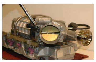
59. Install the throttle body using the stock hardware and torque to 106 in-lbs with a 10mm socket wrench. Verify your torque wrench settings.
