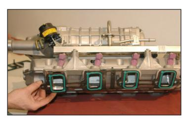
55. Now install the stock gaskets onto the new supercharger manifold.
