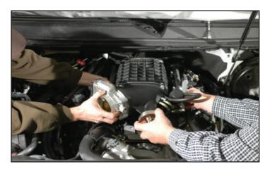
60. Upon complete curing of the adhesive, remove the temporary guide bolts and then the tape from the stand-off plates. Spray silicone or some mild soap and water solution on mating surface of the stand-off plate to lubricate. This makes the intake manifold slide around easily to help line up the holes. With the help of an assistant, carefully set the supercharger assembly into position.
