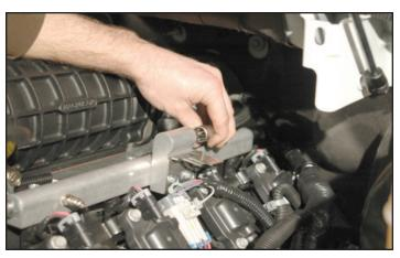
74. Push the fuel line connector on to the fuel manifold. Ensure that the fuel line is pushed all the way on. Pull on the connector to check that it is secure, you should not be able to remove the connector unless you use the removal tool.
