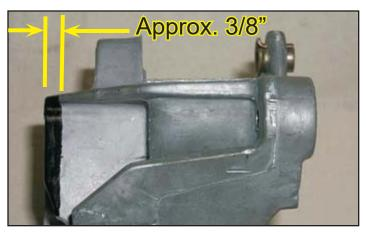
45. On the back surface of the alternator mount, remove the shaded area as shown.
