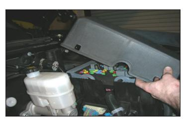
I19. Now, re-install the fuse cover onto the fuse center. (Be careful not to pinch any wires.)
