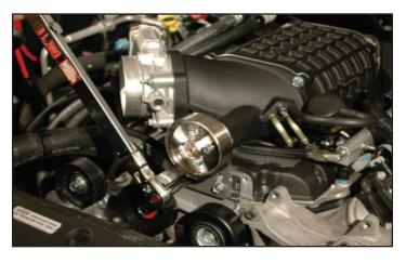
81. Install the supercharger nose support bracket with the two bolts provided. Torque bolts to 15-17 ft-lbs with a 12mm socket wrench. Verify your torque wrench settings.
