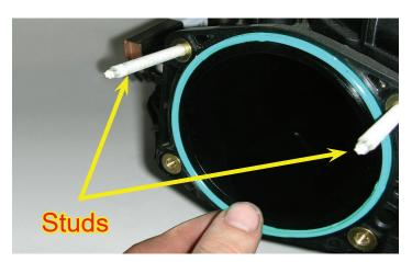
54. Remove the stock throttle body O-ring and studs from the OEM stock manifold. Clean off any oil before installing the O-ring onto the supercharger inlet.
