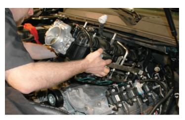
32. With all of the bolts removed, lift the intake manifold up and out of the vehicle and set aside. CAUTION: Take care not to drop any bolts, dirt or any debris into the intake ports.
