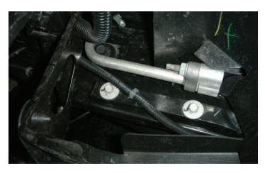
128. Using a 10mm socket wrench, remove the two bolts on the passenger-side of the "A" frame bracket that secures it to the lower radiator support. Repeat on the driver side of the "A" frame.
