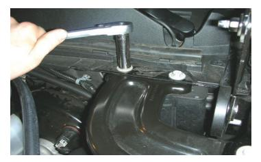
117. Re-install the fender to the firewall brace.
