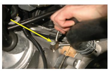
60. Install the supplied vent pipe using the stock hardware, torque to 106 in-lbs. **Note: Verify your torque wrench settings.**
