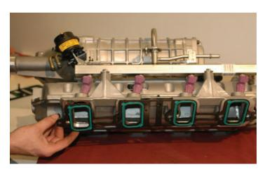
52. Now install the stock gaskets onto the new supercharger manifold.
