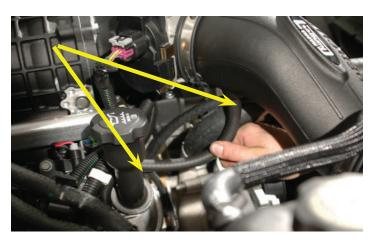
104. Attach the remaining 3/8" hose (left over from a previous step-about 9") from the right (passenger-side) valve cover to the barb on the bottom of the air tube.
