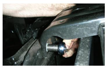
129. Remove the two upper bolts that secure the "A" frame bracket to the upper radiator support with a 10mm socket wrench.
