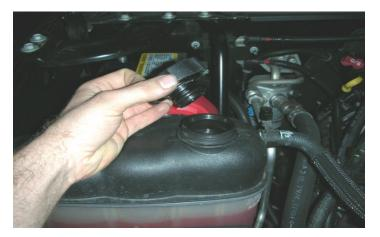
With a cool engine remove the radiator cap.
