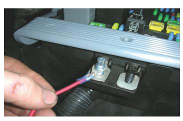
112. Next, take the fused red wire and cut off the 6mm eyelid connector and replace it with the supplied 8mm eyelet connector and install the wire onto the M8 stud in the fuse center.
