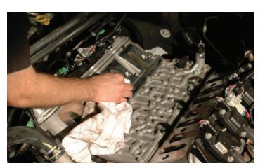
39. Remove the tape from the intake ports that was installed earlier. Clean off the receiving end of the heads using a suitable non petroleum based solvent (such as alcohol, lacquer thinner) to remove any residue. CAUTION!
