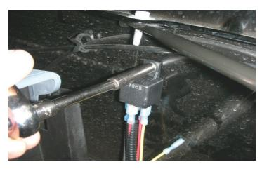
109. The intercooler relay harness is going to mount on the driver side inner fender just below where the fender support bracket is mounted. Use the self-tapping screw supplied to drill a hole, then use the screw to mount relay to fender.
