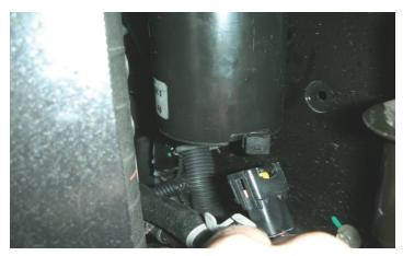
143. Route the electrical plug for the intercooler pump between the PCM and the fender well, through the radiator support and connect the plug to the pump.
