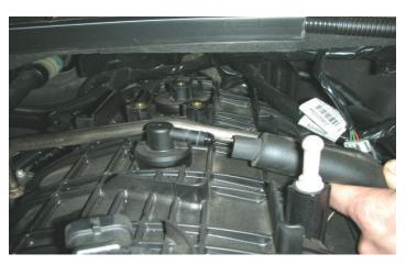
24. Next, remove the PCV hose from the top of the intake. Also, remove the other end of the hose from the rear of the valve cover. This will not be re-used. NOTE: On 2009 and up model year vehicles, this connector has changed. To remove, first the clip connector on the valve cover needs to be released and disconnected. Then rotate the entire assembly clockwise 90° (looking down on the intake manifold) then pull up as the twist lock is released.
