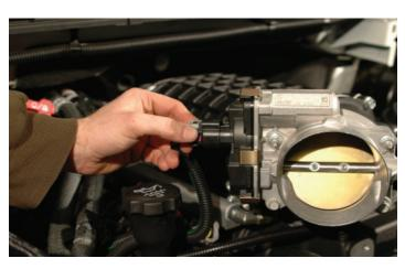
76. Plug the electrical connector for the ETC back into the throttle body.
