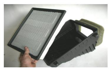
97. Remove the stock air filter from the air box.
