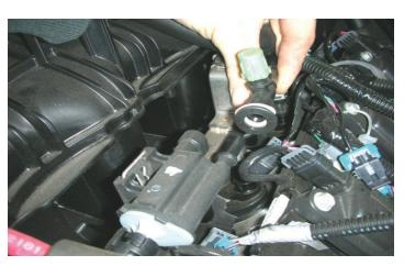
22. Remove the EVAP line from the solenoid by pressing in the gray retainer clip and pulling the line off of the solenoid. Repeat procedure for removing the other end of this line. Your vehicle may not have the test port (the green cap) shown in this picture.
