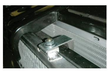
136. Install the two upper LTR brackets. Be sure the foam side is against the air conditioner condenser and secure it with the two M8 nuts provided.
