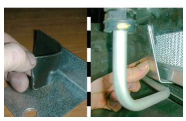
138. Cut and attach a strip of the adhesive backed rubber provided to the "LTR" bracket as shown. Slide the lower "LTR" bracket into place behind the "A" frame bracket.
