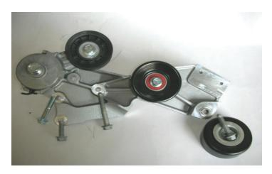
68. Here is the tensioner assembly showing where the specific bolts and where the factory idler goes.
