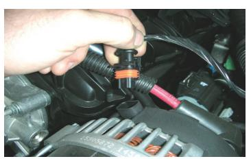
27. Before unbolting the intake manifold, remove the alternator. This should be done to ease the removal of the manifold. Start by disconnecting the electrical connector on the top of the alternator.
