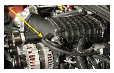
92. Route the front hose from the EVAP Solenoid to parallel the Bypass Valve hose and connect to the remaining barb on the supercharger nose.
