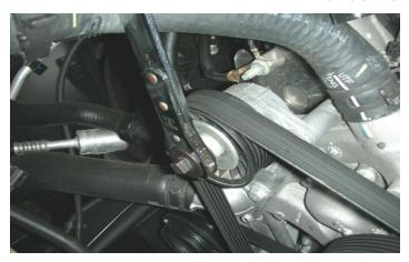
29. Remove the stock belt using a 15mm belt tensioner wrench on the tensioner pulley. The belt will be replaced with the longer belt provided in the kit.
