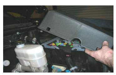
16. Now, re-install the fuse cover onto the fuse center. (Be careful not to pinch any wires.)
