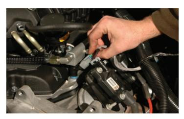
74. Take the eight fuel injector plugs and connect them to the eight fuel injectors. Note: Make sure that the connectors are seated on the injector and locked in place. Pull the harness connector to ensure a good contact.
