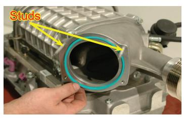
55. Install the two studs from the previous step into the supercharger intake tube using a #5 Torx socket. Then press the throttle body Oring into the inlet tube groove as shown.
