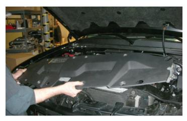
123. Remove the radiator support cover from the vehicle. Set aside to be re-installed later on.
