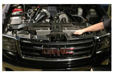
124. Remove the grille from the vehicle. There are four bolts to remove using a 10mm socket wrench. The grille is held in place with snapin fasteners, carefully release the retainers and then unsnap the upper bumper insert from the grille releasing the grille from the vehicle. Note: With the grille out, the intercooler pump and LTR mounting can now be done.
