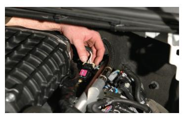
77. The MAP sensor can also be plugged back in. Sensor location is now at the rear of the manifold and no wire extensions are necessary.
