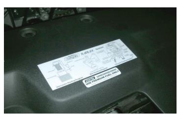
152. Place the belt/vacuum routing diagram onto the radiator support cover.
