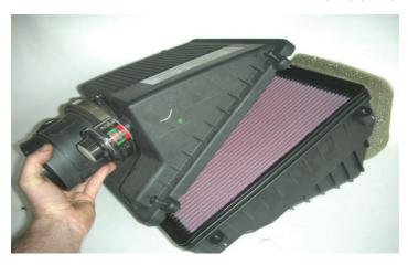
99. Re-install the air box lid and then install the air box assembly back into the vehicle.
