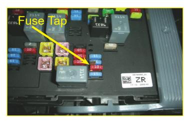
108. Install the supplied fuse t-tap onto the fuse and re-install the fuse back into the fuse box.
