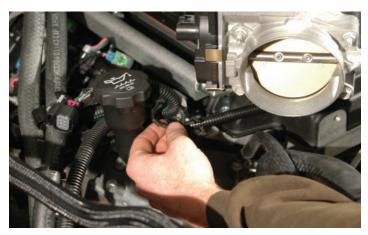
75. Remove the plastic loom clip from the wirelooms located next to the oil filler neck with a flat blade screwdriver.
