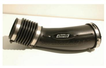
101. Assemble the bellows and coupler to the air tube. Note: The position of the clamp screws. The screws must be facing up so that you can install the assembly on the vehicle.
