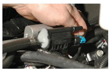
87. Plug in the electrical connection to the EVAP Solenoid.
