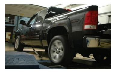
159. After the initial test drive gradually work the vehicle to wide open throttle runs, listen for any engine detonation (pinging). If engine detonation is present let up on the throttle immediately. Most detonation causes are low octane gasoline still in the tank. Install the provided "Use Premium Fuel Only" sticker to the inside of the fuel filler door.
