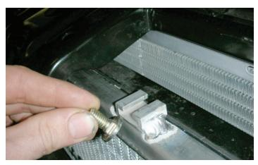
135. Slide the two M8 "T" bolts into the "T" channel on the LTR.
