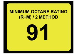
Your system requires the use of minimum 91 Octane gasoline fuel. This system is not compatible with E85 fuel.
