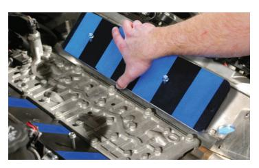
40. Use four of the provided manifold bolts in the existing holes to guide the stand-off plates into position with the grommet-gaskets facing down onto the heads. These bolts will NOT be tightened; they are for alignment purposes only.
