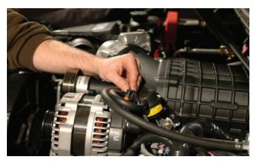
93. Plug in the Electric-Voltage sensor wire into the Alternator connector as shown.
