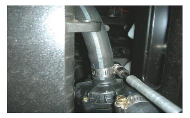
149. This hose will route directly to the inlet barb on the intercooler pump. Trim to fit, and secure the hose with the supplied #10 clamp.
