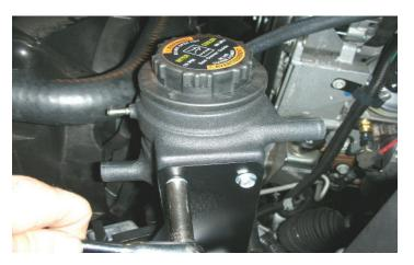
121. Mount the intercooler reservoir tank to the bracket using the three M6 X 12mm bolts. Tighten the bolts using a 10mm socket wrench.
