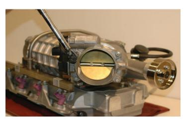
56. Install the throttle body using the stock hardware and torque to 106 in-lbs with a 10mm socket wrench. Verify your torque wrench settings.
