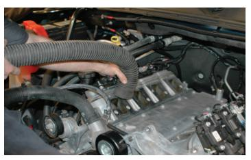
33. Using a vacuum cleaner remove any dirt of debris from the intake port area. Then tape over the intake ports. CAUTION! Be careful not to get any dirt down the intake ports.
