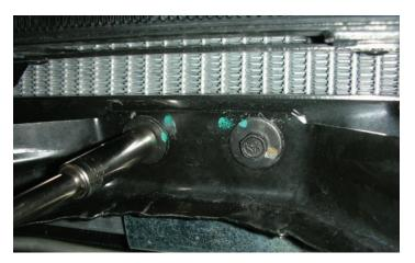
137. Using a 10mm socket wrench remove the two bolts located at the bottom of the "A" frame bracket.
