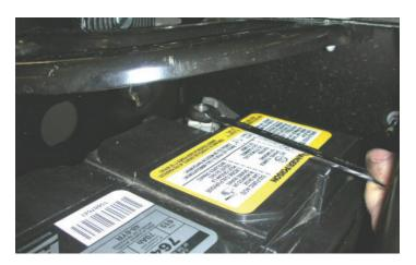
Disconnect the negative (-) lead of the battery cable. Cap or cover the terminal to protect against accidental contact with the battery post.
