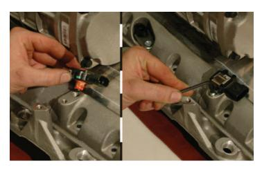
55. Spread some of the supplied Lubriplate lubricant on the MAP sensor seal (see inset photo), and press the MAP sensor into the provided hole in the supercharger manifold as shown. Using a 4mm Allen wrench, install the MAP sensor retaining clip with the provided 6mm button head screw as shown.
