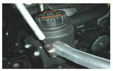
147. Route the hose connected in step #144 to the intercooler reservoir tank. Trim the hose to fit, connect it to the intercooler reservoir tank upper 3/4" hose barb, and tighten with the #10 clamp provided.
