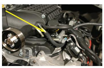
80. Route the other end under the coil bracket to the supercharger nose, and plug into the supercharger barb as shown.
