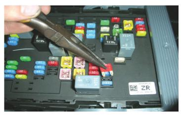
107. Remove the 10amp mini-fuse in the fuse box that is labeled HVAC-IGN. **NOTE: Fuse location may vary so verify by fuse name!**
