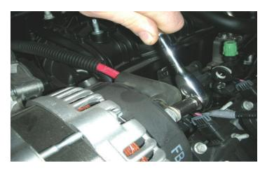
28. Using a 10mm socket wrench, remove the nut holding the positive (+) wire to the back of the alternator. Route the wire over towards the passenger-side fender, out of the way.
