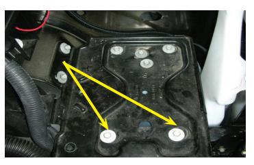
118. To install the intercooler reservoir tank bracket you must remove these two bolts, using a 10mm socket wrench.
