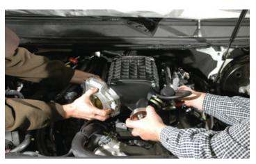
57. Upon complete curing of the adhesive, remove the temporary guide bolts and then the tape from the stand-off plates. Spray silicone or some mild soap and water solution on mating surface of the stand-off plate to lubricate. This makes the intake manifold slide around easily to help line up the holes. With the help of an assistant, carefully set the supercharger assembly into position,
