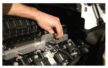
71. Push the fuel line connector on to the fuel manifold. Ensure that the fuel line is pushed all the way on. Pull on the connector to check that it is secure, you should not be able to remove the connector unless you use the removal tool.
