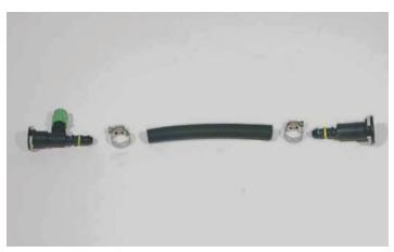
83. Cut a section of the 3/8" hose to 11" in length. Install the factory fittings removed in the previous step onto the ends.
