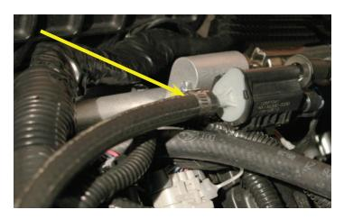
86. Cut a piece of the provided 3/8" hose to 16-1/2". Attach and clamp one end to the front barb on the EVAP solenoid.
