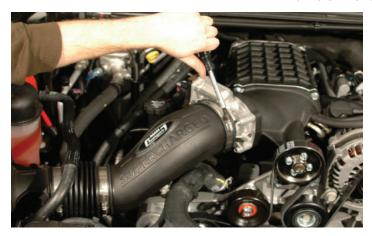
103. Push the bellows end of the air tube assembly on to the air box first, and then install the remaining end with the coupler on to the throttle body. Tighten all clamp screws securely.
