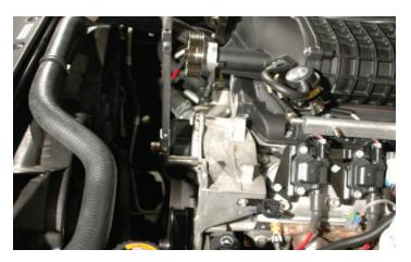
70. Torque all the bolts to 40ft-lbs with a 15mm socket wrench. Verify your torque wrench settings.
