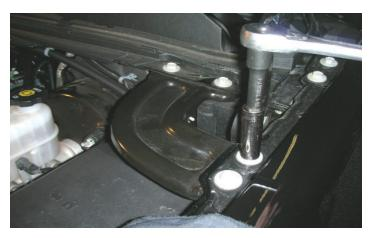
105. Remove the driver side fender to firewall brace with a 13mm socket wrench, to gain access to the fuse relay panel.
