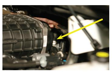
144. There are two ¾" hose barbs at the rear of the supercharger. Using a 4" x 36" x ¾" 90° molded hose, cut 1" off the short end. Starting at the intercooler barb closest to the passenger side of the vehicle, attach the short end of the 90° to the barb with a #10 clamp. Run the hose forward toward the intercooler reservoir. Note: Clamps may vary between squeeze style and screw style.
