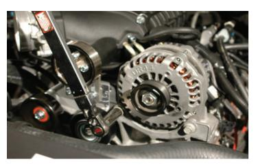
90. Using a 15mm socket wrench torque the two bolts to 40ft-lbs. Verify that your torque wrench is set to ft-lbs.
