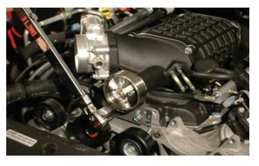
78. Install the supercharger nose support bracket with the two bolts provided. Torque bolts to 15-17ft-lbs with a 12mm socket wrench. Verify your torque wrench settings.
