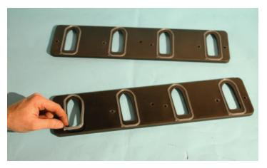
37. Press each grommet-gasket into the receiving groove on the stand-off plate. There is only one way they will fit. Just match the tab on the grommet to the corresponding point on the stand-off plate groove.
