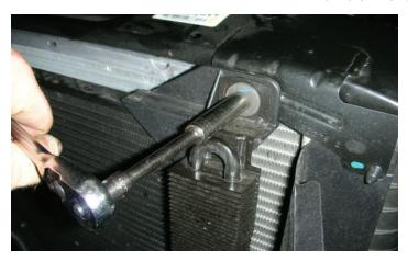
127. Using a 10mm socket wrench, remove the two bolts that hold the power steering cooler in place. The 2nd bolt (not pictured) is attached to the "A" frame bracket. Move the cooler aside for now.
