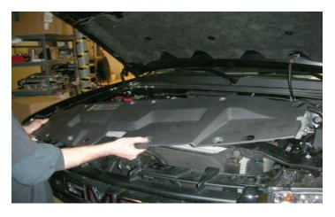
154. Reinstall the radiator support cover on the vehicle using the stock hardware.
