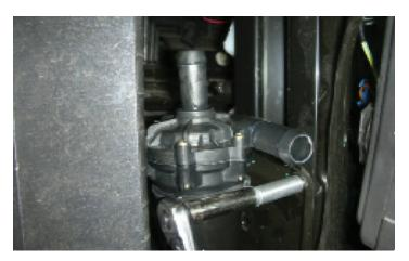
126. Locate the Adel clamp, and put it on the intercooler pump, then using the 6mm x 55mm bolt and the spacer supplied install the intercooler pump to the radiator support.
