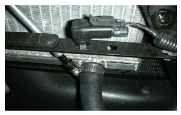
151. Finally route the hose to the remaining barb on the driver-side of the LTR, secure with provided #10 clamp and tighten.
