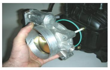
53. Using a 10mm socket wrench, remove the stock throttle body from the OEM intake manifold. Next, using a #5 internal Torx, remove the two mounting studs from the stock manifold.
