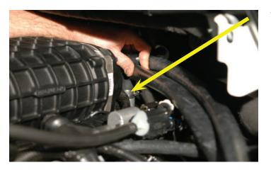
145. Using the supplied 4" x 60" x 3/4" 90° molded hose, attach a 3/4" hose coupling to the long end of the hose. Connect the short end to the remaining supercharger barb (it should be the one closest to the driver side of the vehicle) and secure it with a #10 clamp.
