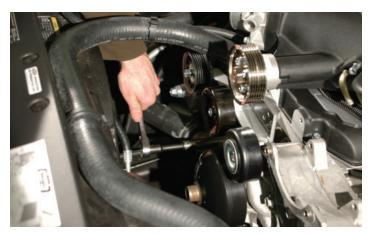
69. Install the tensioner assembly into the vehicle as shown.
