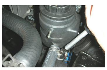
148. Put a piece of the remaining 3/4" hose onto the other 3/4" barb (lower) on the intercooler reservoir and secure with a #10 clamp provided.
