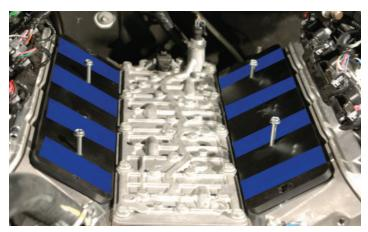
41. The two stand-off assemblies should look like this. Allow the adhesive to set completely before proceeding.
