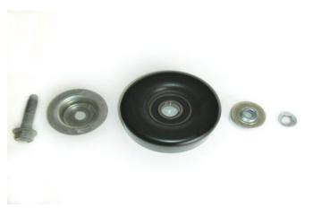
67. Using a soft hammer, knock the factory bolt loose from the idler pulley. The bolt retainer and stand-off (pictured here on the right side of the pulley), will not be re-used. Note: The bolt, dust cover and idler will mount to new tensioner bracket.
