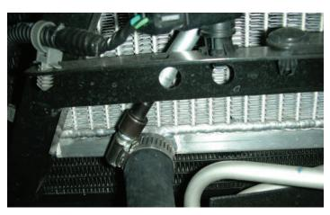
146. Connect one end of the provided ¾" hose to the hose coupling just installed. Route the hose through the radiator support and under the intercooler pump, trim to fit and connect it to the passenger side barb on the LTR. Secure all connections with the #10 clamps provided.
