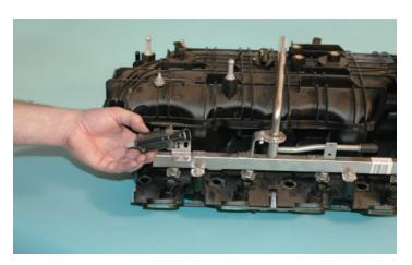
50. Remove the stock EVAP solenoid from the stock manifold by lifting up to free the unit from the mounting bracket.
