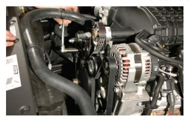
95. Using the belt routing diagram as a guide install the new belt provided. Slide the idler pulley down and torque to 40ft-lbs using a 15mm socket wrench. Verify your torque wrench settings. Finally remove the pin and release the tensioner. Make sure belt contacts all pulleys correctly.
