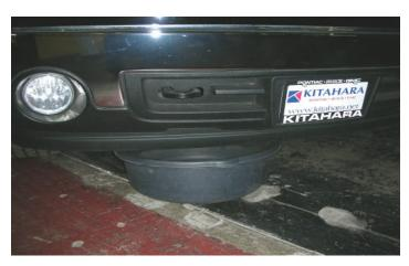
12. Place a drain pan under the front of the truck and disconnect the heater hose on the passenger-side on the water pump.
