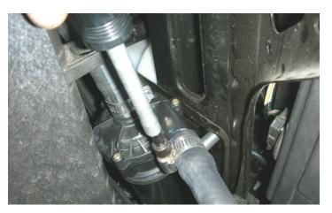
150. Using the last of the remaining ¾" hose, attach one end to the outlet barb on to the intercooler pump.
