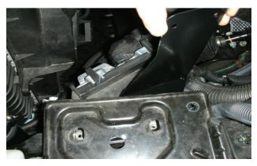
119. Lift up on the secondary battery tray and slide the intercooler reservoir tank bracket under the tray, lining up the holes on the bracket with the holes on the tray.
