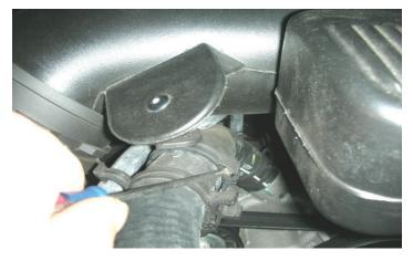
Disconnect the loom clamp from the upper radiator hose using a small flat blade screwdriver.
