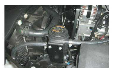
156. Refill radiator and intercooler system with vehicle manufacturer recommended coolant mixture. Let run for 5-10 minutes. Bleed system at "T" and at reservoir. Check system periodically for fluid level.
