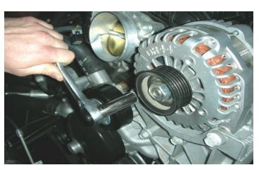
30. Using a 15mm socket wrench, remove the two bolts securing the alternator to the bracket and remove the alternator from the vehicle.
