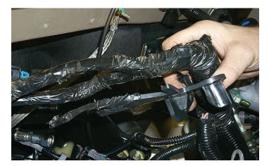
73. Remove the wiring harness from the original bracket
