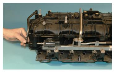
49. Disconnect the short EVAP pipe from the EVAP Solenoid on the stock intake manifold.
