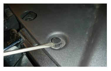
122. Using a flat blade screwdriver, remove the eight plastic pushpins from the radiator support cover.
