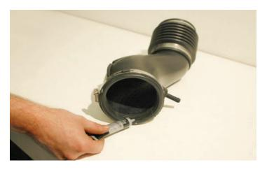
102. Using some of the O-ring grease supplied, apply a light coating of grease on the inside of the coupler.
