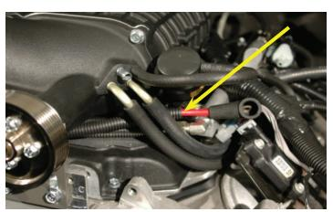
85. Route the battery positive (+) cable below the supercharger nose, behind the brake and PCV hose for later connection to the alternator.
