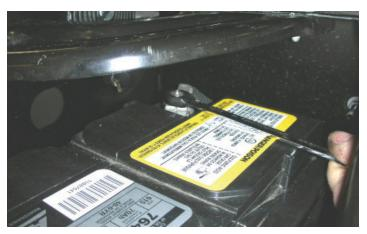
155. Re-connect the battery with a 10mm socket wrench.
