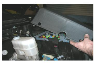
106. Pull back on the two tabs holding the fuse cover to the fuse box and lift the cover out of the vehicle.
