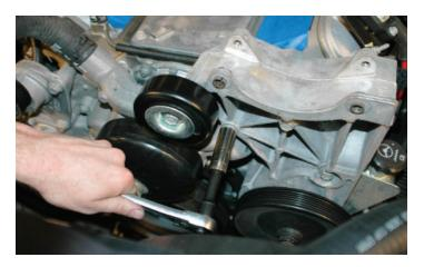
47. To make installation of the supercharger manifold easier, remove the alternator/power steering bracket from the engine block. Using a 15mm socket wrench, remove the four bolts on the front side and the bolt on the lower driver-side.
