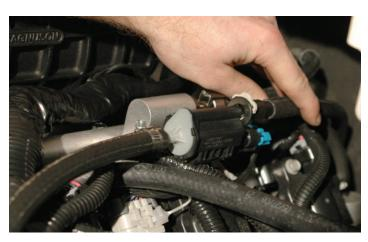
88. Plug in the end of the hose assembled in step #82 to the remaining (rear) barb on the EVAP Solenoid. Plug the other end onto the barb at the driver side rear of the engine from whence it was removed.
