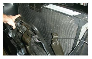
130. Move the "A" frame bracket forward to allow clearance for the LTR (heat exchanger) to be installed.
