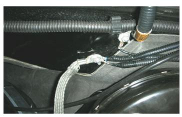
115. Crimp the supplied 6mm eyelet connector onto the ground (black wire) wire from the intercooler relay, install it onto the ground stud and re-install the factory nut.
