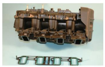
51. Remove the stock intake manifold gaskets from the OEM intake manifold.
