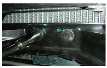
139. Re-install the factory hardware and tighten the two bolts.
