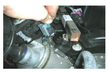
18. Unplug the eight fuel injector plugs by pulling up on the gray tab and then pushing in on the release tab.
