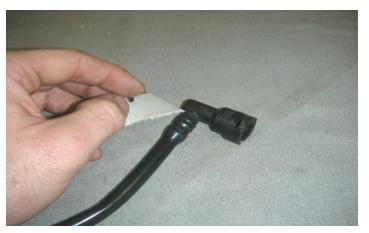
82. Take the rear EVAP hose from the stock manifold and carefully cut out the fittings at the ends of the hose.
