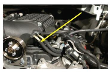
81. Cut a section of the provided 3/8" hose to 25" in length. Plug one end into the PCV barb at the back of the driver-side valve cover. Route the other end under the coil bracket and plug into the hose barb on the supercharger as shown.
