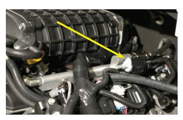
84. Install the OEM EVAP Solenoid on the mounting bracket on the driver side fuel rail manifold. NOTE: The electrical connection of the Solenoid should be pointing toward the firewall.
