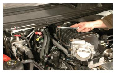
59. Using a rotating pattern tighten all ten intake manifold bolts. Torque all ten bolts gradually and evenly to 106 in-lbs. Note: Make sure your wrench is set to torque to in-lbs, not ft-lbs.
