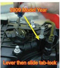
48. Remove the stock MAP sensor by removing the retaining clip with a screwdriver and then gently pulling up the sensor. Be careful not to damage the O-ring seal. NOTE: On 2009 model year this connector may have changed. To remove, insert a small screwdriver into the slot opposite the slide-tab lock. Lever the locking tab outward to release the lock, then slide the lock to remove.
