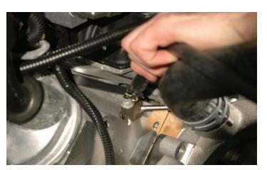
61. Install the supplied steam vent hose and tighten using the stock spring clamp.
