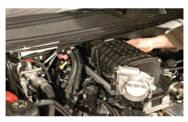
58. Insert the ten intake manifold bolts into position through the stand-off plates. Finger tighten at this time ensuring complete alignment.
