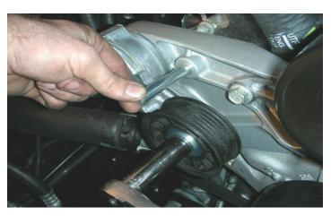
94. Use a 15mm socket wrench to lever the tensioner all the way down, then insert the pin provided into existing hole on the tensioner bracket to hold the tensioner in the compressed position.
