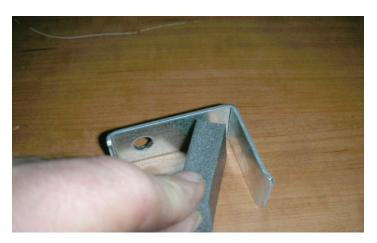
134. Locate the two upper LTR brackets and apply the supplied ½" foam to the brackets.
