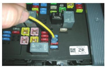
111. Take the yellow wire from the intercooler relay and connect the spade terminal end and install the wire onto the fuse tap installed earlier. (HVAC IGN)
