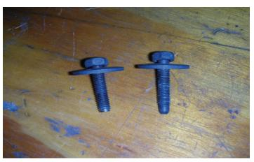
141. Before installing the power steering reservoir to "A" frame the lower bolt needs to be shortened so it doesn't interfere with the LTR. This can be done with a hacksaw or a suitable grinding tool.
