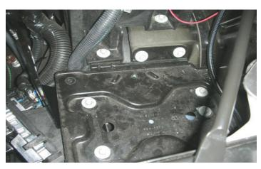
120. Using a 10mm socket wrench, re-install all bolts that were removed.
