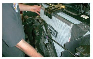
133. Carefully slide the LTR in between the "A" frame bracket and the air condition condenser. The LTR will go under the top of the "A" frame-mounting bracket.
