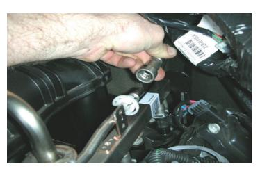
26. CAUTION! Always wear safety glasses when working with fuel. Continue on with the next three steps ensuring that the negative (-) battery cable is still disconnected. Using the fuel disconnect tool provided, remove the fuel line from the fuel rail. CAUTION! Fuel system may be under pressure. Avoid open flames or any source of ignition.
