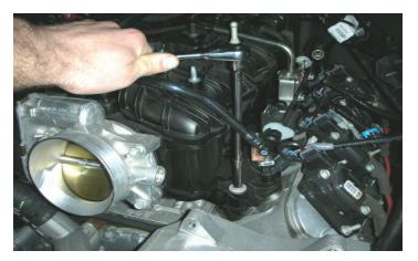
31. The intake manifold is now ready to be removed. Using an 8mm socket wrench, remove the ten bolts that secure the manifold to the engine.
