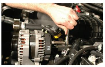
91. Ensuring that the battery is still disconnected, connect the battery positive (+) cable you routed in a previous step to the back of the alternator and secure the nut with a 10mm socket wrench.
