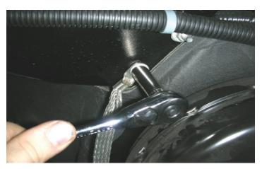
114. With a 10mm socket wrench, remove the nut securing the ground cable to the firewall.
