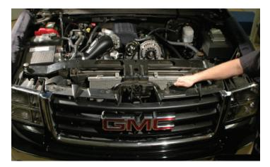
153. Re-install the grille on the vehicle using the stock hardware.
