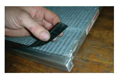
132. Cut the supplied 3/32" rubber strip into two 22 ½" long pieces. Apply the rubber strip to the end tanks on the LTR.
