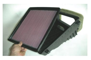
98. Take the new K&N air filter supplied in the kit, and install it into the air box.
