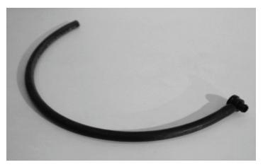
79. Cut a section of the provided 11/32" brake hose to 26" in length. Install the stock check valve on one end, and plug the check valve into the brake booster.
