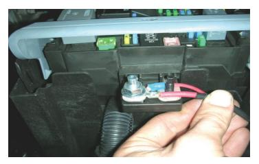
113. Using a 12mm socket wrench, and the nut provided, secure the fused red wire to the M8 stud.
