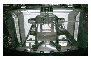
140. Using all the factory hardware, re-install the "A" frame to the support bracket.
