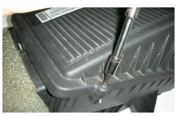
96. Using a T-25 torx socket, remove the four screws that attach the air box lid to the lower half of the air box.
