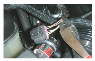
62. Locate the MAF electrical plug, pull back the flex loom about 12", and cut the tan wire and the tan w/black stripe wire about 2" from the MAF connector.
