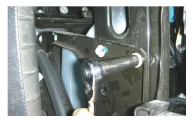
125. Using a 10mm socket wrench, remove the bolts shown, this is behind the drivers' side headlight, it is bolted to the radiator support.
