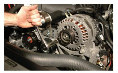
89. Next, re-install the alternator using the factory hardware.
