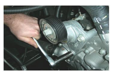
42. With a 15mm socket wrench, remove the three bolts that hold the tensioner to the water pump and remove the tensioner. Notes: The tensioner won't be re-used, but one long stock bolt, and the short stock bolt will be re-used. \*Some 08-09 tensioners only have the two long bolts. We will still use one of those and will supply a new bolt to take the place of the short stock bolt that wasn't installed originally.
