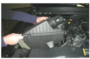
14. Firmly grasp the air intake box and pull up, removing it from the vehicle. The air box will be re-installed in a later step.
