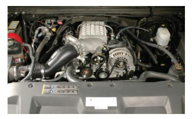
157. Start the vehicle for 5 seconds and shut off, once again check for fuel leaks and fansupercharger belt alignment. Check radiator and intercooler reservoir.
