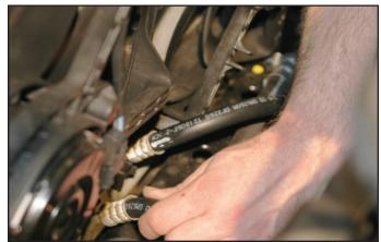
43. Using a medium flathead screwdriver, push down on the top locking pins to release the upper Fan Shroud mount.
