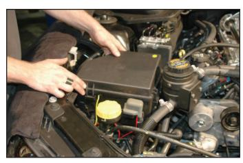
192. Remove the inlet coupling from the inlet air tube and install it on the throat of the throttle body.
