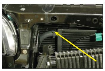
84. There are three provided transmission cooler offset brackets. Attach one to the upper passenger side bolt hole (place a provided washer between the bracket and frame for this hole) where the transmission cooler was originally mounted using the provided bolt. Attach one to the driver side bolt hole from where the transmission cooler was originally mounted.
