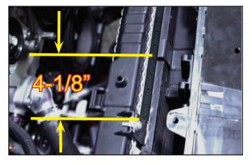
81. Next, trim the rubber seal in the two spots as shown. This will allow the seal to re-install around the Heat Exchanger brackets.
