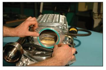
121. Install the Throttle Body on the supercharger using a 10mm socket wrench, torque the bolts to 106 in-lbs. Make sure you are using the correct settings for your torque wrench.
