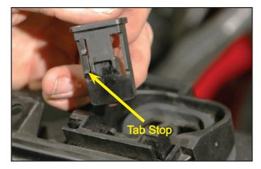
74. From inside the slot where the lock tab was removed, use the small flathead screwdriver to lever the final locking tab inward, allowing the upper radiator mount to be pulled up and free of the frame.
