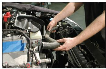
39. Remove the coolant overflow tube from the hose barb just below the radiator cap, unclip from mounts and coil up on the passenger side of the vehicle out of the way.
