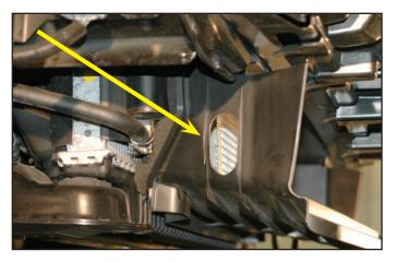
170. Cut a 46" section of the supplied 3/4" hose and connect one end to the lower heat exchanger barb using the provided clamp. Route the hose through the holes, up over the lower radiator hose.
