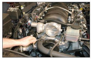
21. Pull the vacuum brake hose free from the power brake booster.
