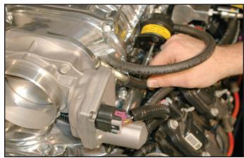
147. Cut 20" of 11/32" brake hose supplied; attach the stock check valve on one end.
