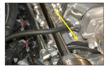
157. Ensure that the wire loom does not contact the jack-shaft and that the wires are covered completely.
