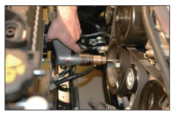
52. Using a 24mm socket, remove the large bolt and drill guide from the engine.
