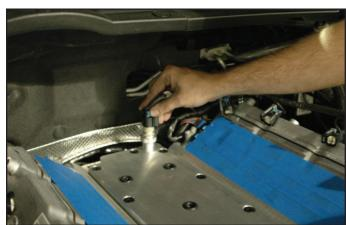
71. Using a medium flathead screwdriver, pry up on the radiator release tabs. They will slide up easily until they hit a "stop".
