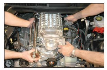
125. Remove the split loom spacers from the intake manifold bolts so that the bolts can drop down to engage the threads on the heads.
