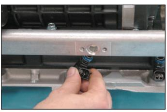
115. Lubricate the upper O-rings of the stock injectors, align and carefully press the fuel rails down onto the installed injectors.
