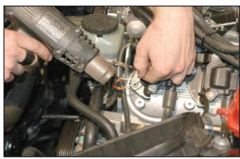
156. Re-place the split loom to the MAF plug. Cut a piece of split loom (supplied) to cover the new wires under the supercharger inlet (approximately 19") to the IAT sensor wire ends.
