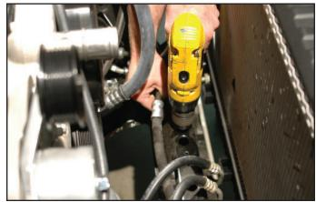
93. With the radiator mounted back in its stock location, you can now re-install the electric fan assembly.
