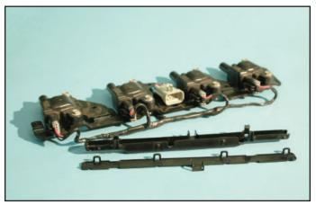
105. Trim the plastic cowl at the center of the run as shown and described. From the center seam, trim off 4-1/4" on the driver side. From the center seam, trim off 3" on the passenger side.
