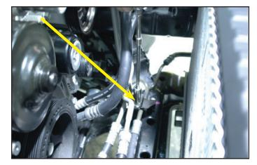
46. Remove the transmission cooler hard-line mounting bracket bolt from the driver side frame rail using a 10mm socket.
