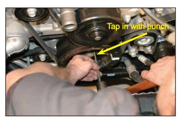
56. Install the new supplied factory GM Harmonic Balancer bolt.
