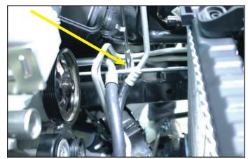
47. Using a 24mm socket and an impact hammer, remove the Main Harmonic Balancer bolt. This will not be reused. Sometimes using a heat gun or MAP gas torch on the surrounding pulley material helps it to break free from the Loctite used during initial installation. Don't heat the bolt itself and always use care using open flame around engine compartments and combustible material.
