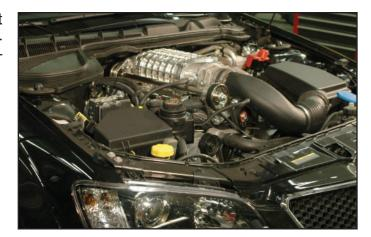
206. Test-drive the vehicle for the first few miles under normal driving conditions (**Do not perform any wide open throttle runs**). Listen for any noises, vibrations, engine misfire or anything that does not seem normal. The supercharger does have a slight whining noise under boost conditions, which is normal.
