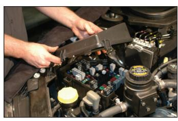
180. Remove the HVAC ignition fuse (slot F-37), verify the fuse by fuse name, in some instances the fuse may be in a different slot.
