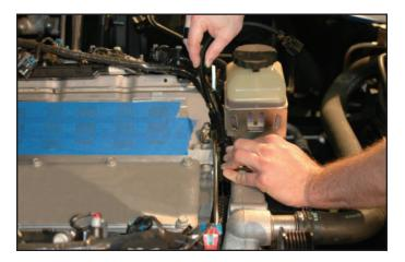
101. Disconnect the main coil connector from the coil rail.
