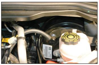
149. The other end of this hose connects to the vacuum barb on the supercharger inlet as shown.
