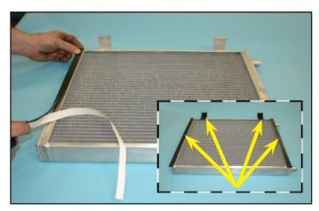
80. Pull back on the top of the radiator toward the engine, slide the Heat Exchanger down in front of the A/C Condenser, hooking the two top brackets onto the condenser. Locate the new Heat Exchanger so that there is 4-1/8" between the existing AC condenser mount to the existing radiator and the new "hook" shaped mounting bracket on the passenger side of the heat exchanger. Be sure not to pinch the small hose coming from the windshield wiper reservoir between the heat exchanger and condenser.
