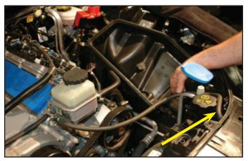
41. Disconnect the Fan Plug from the Fan Shroud housing.
