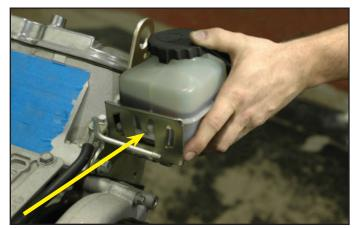
107. Remove the two stock reservoir bracket mounting bolts using a 15mm socket.
