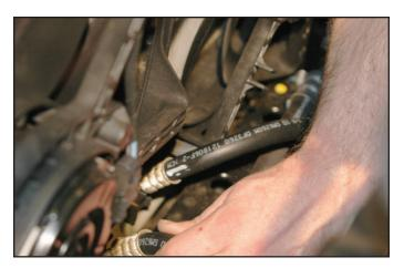
96. You can now re-connect the coolant overflow hose back to the hose barb on the radiator neck.
