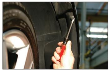
27. For ease of work you can remove the remaining pins and completely take the fender well liners out completely, or you can just bend the panels out of the way as you work.
