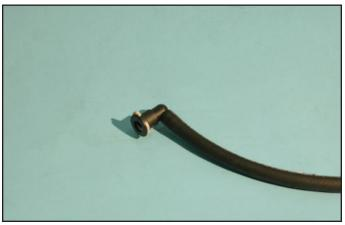
141. Thread the open end of the 40" (5/16") hose under the front of the supercharger assembly, below the throttle body, and back along the coil bracket. Connect the right angle end to the EVAP solenoid as shown.
