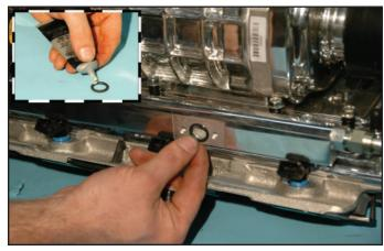
123. Install the fuel supply manifold on the fuel rail, and torque the 106 in-lbs. Verify your torque wrench settings.
