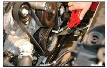
51. Insert the supplied reamer into the drill, and using a small amount of oil, ream the holes clean until reamer bottoms out in the holes.
