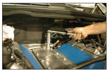
61. Remove the eleven valley cover bolts using a 13mm socket and set aside.
