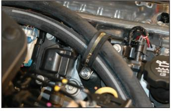
137. Loosely add zip ties to hold the hoses together, and add strips of split loom to prevent chafing on the fuse box.
