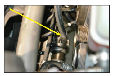
172. In step #83 you installed a 59" section of the supplied 3/4" hose to the upper heat exchanger barb using the provided clamp. Route the hose to follow the bottom heat exchanger hose through the hole in the cowl and into the engine compartment. This photo has the transmission cooler removed for clarity.
