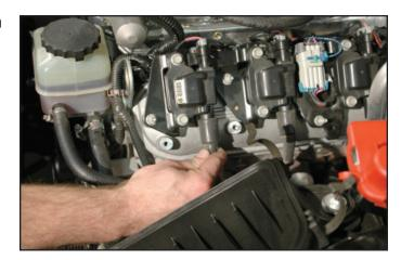
134. Attach the fuel line to the fuel manifold on the driver side of the supercharger. Be sure to attach the safety clip as well. Verify that you have a good connection. You should NOT be able to remove the fuel line without using the fuel line removal tool.
