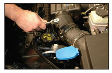
10. Depress the locking tabs on the PCV Vent tube on the passenger side hose barb and pull the connection free.
