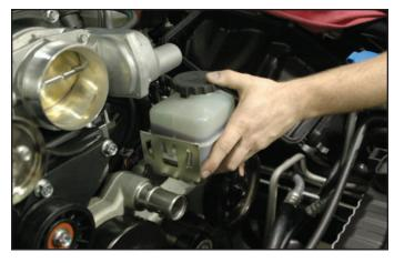
128. Use a flat blade screwdriver to push on and re-engage the metal locking tab of the bracket over the lip of the reservoir bottle.
