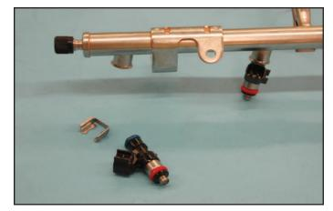
114. Use a 10mm socket wrench to remove the fuel rail bolts connecting the supplied fuel rails to the new intake manifold. You may leave the fuel lines (front and back) attached. Lift the rails up to allow the injectors to be installed. Use the supplied Lubriplate lubricant to lube the O-rings of the stock injectors and insert the eight stock injectors into the new manifold below the fuel rails. Point the electrical connections outward.
