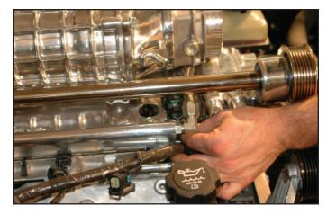
130. Plug the fuel injector plugs to the injectors on each side of the engine. Make sure to route and stuff the wiring to avoid moving components.
