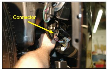
199. Bolt the fascia to the fender with the two connectors on each side and use the factory push-pins to attach at all points (4-each side). If you removed the fender well in step 27, then reattach at this time reversing the procedure.
