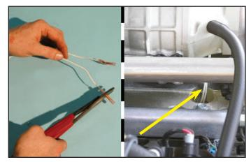
153. Uncover the wire loom to the MAF connector that hooks to the air box. Cut the brown with-white stripe, and the brown with-red stripe about 2" from the connector. The wire ends at the connector are abandoned and can be taped off should you wish.
