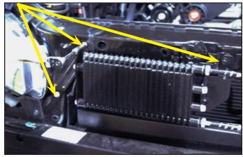
79. Apply the two ½" x 15" and the two 1" x 3" rubber strips to the Heat Exchanger as shown.
