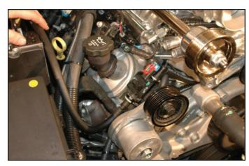
144. The other end of this hose connects to the supercharger hose barb as shown. Add zip tie at the heater hoses near the oil fill cap.
