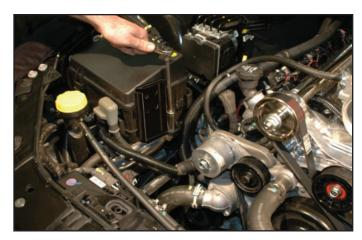
164. This is the intercooler reservoir mounting bracket. The bottom hole mounts to the bolt post for the fuse box where you just removed the nut. From a straight out mount it will need to rotate approximately 30 degrees clockwise. As such the bracket will hit the accessory bracket. Mark the bracket as shown by scribing an estimated notch to be removed.
