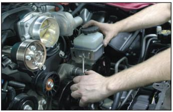
129. Plug in the MAP sensor electrical connector.
