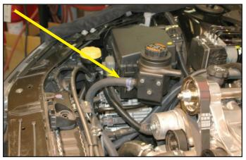
177. Cut an 8" section of the 3/4" hose and connect between the intercooler reservoir and the supercharger hose barb as shown. Clamp with the supplied hose clamps. Make sure you use a supplied worm gear clamp on the reservoir.
