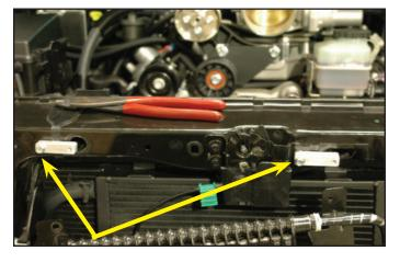
85. The passenger side plastic air deflector will need to be modified to mount the lower transmission heat exchanger offset bracket. Use dykes or cross cutters to cut a notch for the bracket. This will be at approximately 45 degrees from a horizontal plane.
