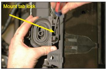
75. This picture shows the mount lock being removed. Repeat on other upper radiator mount. The radiator can now be pivoted backward toward the engine block for heat exchanger installation.
