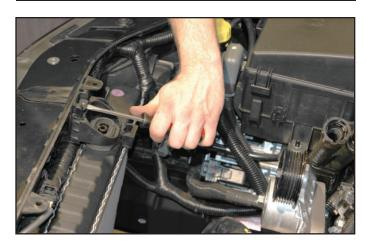
72. This stop is accessed from the front side of the release tab, and using a small flathead screwdriver you depress the stop allowing you to pull the radiator mount lock free from the upper radiator mount.
