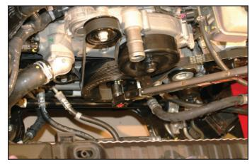
49. Using a small or angled 3/8" drill and the supplied drill bit, insert the drill into the two guide holes and drill to the second step of the drill bit. Be sure that you drill all the way to the second step, and use with suitable cutting oil. (Caution: Wear safety glasses)
