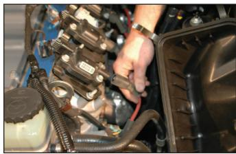
103. Remove five 10mm bolts from the coil brackets on each side, and remove the coil brackets from the engine to be modified below.
