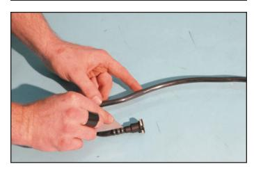
140. Cut a piece of the supplied 5/16" hose to 40" long and install the right angle fitting removed in the prior step. No clamp is necessary.
