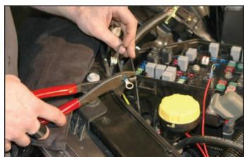
187. Use a 13mm wrench to remove the fuse mount bracket bolt. Re-attach the bolt incorporating and grounding the black lead wire.
