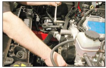
59. Disconnect the oil pressure sensor connection at the rear of the valley cover.
