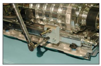
124. Remove the tape from the heads and lubricate with silicone spray (non petroleum base lubricant). Get another pair of hands to help, and carefully lift the supercharger assembly into the engine.
