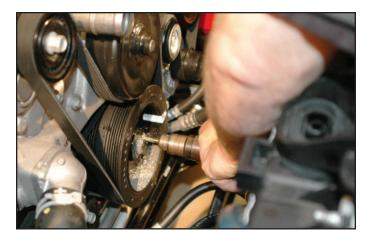
50. Using compressed air, blow the drill shavings out of the holes. (Caution: Wear safety glasses, and make sure that debris doesn't blow into surrounding openings...such as the thermostat housing etc.)
