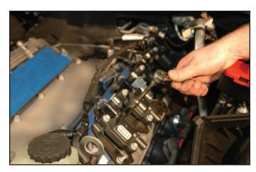
104. Remove the plastic wire loom covers from the coil bracket assemblies. Do this procedure on both sets of coils.
