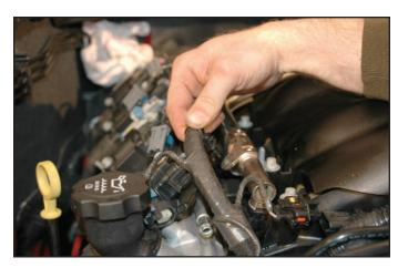
16. Remove the EVAP link by squeezing the yellow saw-tooth tabs and pull free from both ends, put aside for later use.
