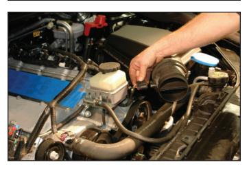
36. Unclip the five spring clips that hold the Airbox cover in place.
