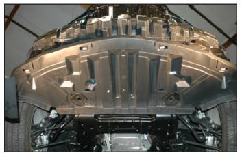
197. Re-install the front end fascia using the stock hardware (2-bolts, and 2-push pins) on the top surface.
