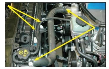
98. Locate the ETC connector on the engine harness. This will need to be extended with the supplied extension harness.
