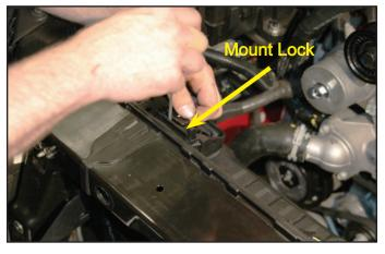
73. This picture is a closeup of the locking tab that needs to be depressed to allow the mount lock to be removed.
