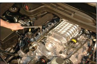
127. Slide the power steering reservoir back onto the relocated mounting bracket, guide the tongue of the reservoir into the receiving angles of the bracket.
