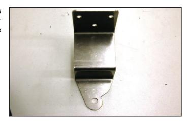
166. The top section of the existing accessory bracket will rub against the reservoir bottle and must be modified as well. From the outside forward edge, scribe a line back to the rear bend angle. This section will need to be removed. Use a cutting wheel, saw or suitable file to take this section out. Make sure you also dress the surfaces to eliminate any sharp edges.
