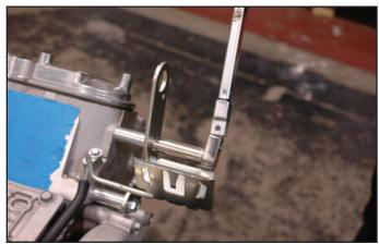
111. Remove the MAP sensor from the stock intake manifold.
