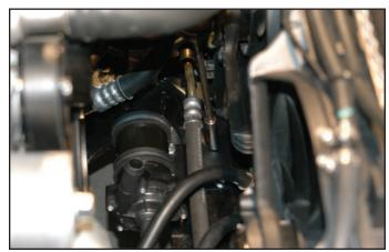
163. To mount the intercooler reservoir you will use the fuse box mounting bracket and need to modify the existing accessory bracket. Remove the nut with a 13mm socket.
