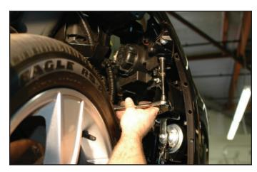
200. Use the four 7mm bolts to bolt the fascia through the "splash shield".
