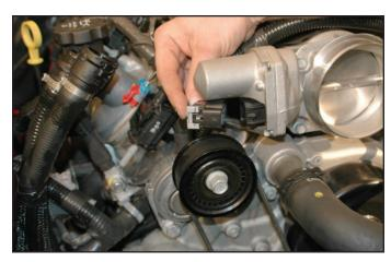
20. Unbolt the four bolts of the throttle body using a 10mm socket wrench and remove the throttle body, put aside for later use.
