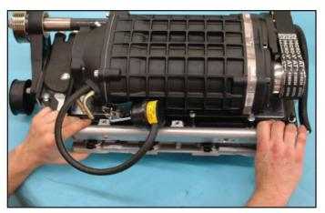
116. Reinstall the fuel rail bolts and torque to 106 in-lbs. Verify your torque wrench is correctly set to inch-pounds.
