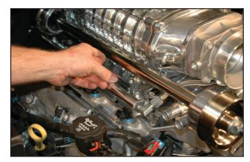
126. After an initial hand tightening, torque the bolts down to 106 in-lbs. Make sure you check your torque wrench settings. Rear passenger side bolt is difficult with a torque wrench, you may have to use an open-end wrench to reach this bolt or preferably an open-end crows-foot wrench to connect to your torque wrench. To allow more clearance in the work environment, you may want to remove the driver-side fuel rail.
