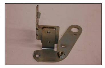
110. Place the provided bolts through the holes of the bracket, insert the provided spacers and bolt the bracket back onto the engine. Torque the bolts to 35-40 ft-lbs. Verify your torque wrench settings.
