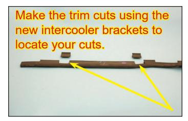
82. Now re-install the modified rubber seal onto the condenser. Refer to steps 71 thru 75 to reinstall the plastic upper radiator mounts to secure the radiator back in place; then reinstall the bracket locking tabs.
