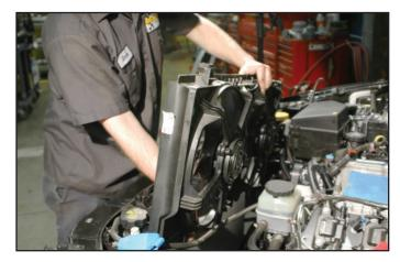
94. Plug the electrical connection back into the fan assembly.
