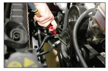
54. Insert the two supplied hardened roll pins into the drilled holes.
