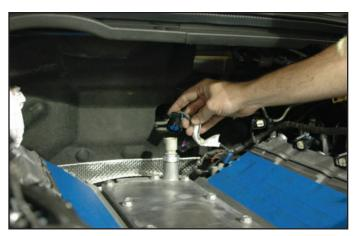
60. Remove the oil pressure sensor from the valley cover using a 6-point 1-1/16" socket or wrench, put aside for later re-installation.
