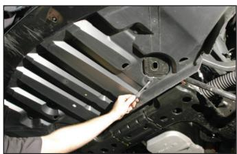
31. Remove the two push pins and two 10mm bolts from the top of the front end panel connecting the front end fascia to the upper radiator support.
