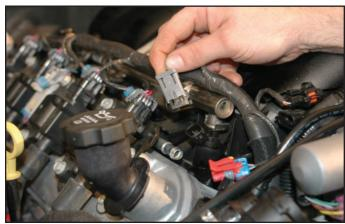
15. Pull the injector wire loom free from the stock intake manifold fuel rail mounting holes.
