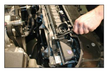
44. Pull the Fan Shroud assembly free from the vehicle and put aside for later re-installation.
