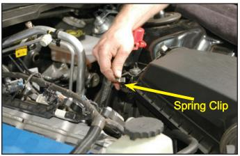
37. Remove the cover, put aside to reinstall later.
