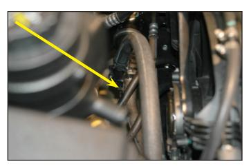
176. Route the hose to the intercooler reservoir and connect to the hose barb as shown using the supplied worm gear clamp.
