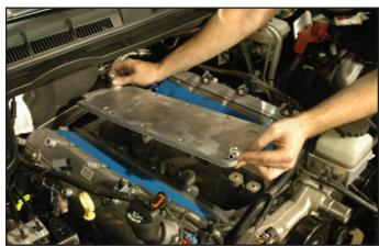
63. Verify the integrity of the existing valley cover gasket, and that it is correctly positioned on the valley surface.
