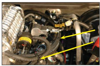
151. Cut a 16" section of the supplied 3/8" hose. Connect one end to the hose barb on the passenger side, front-above valve cover. The other end will connect to the inlet tube to be installed later.
