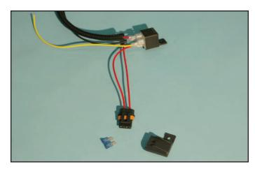
184. Zip tie intercooler relay to wire bundle adjacent to the coolant reservoir fill cap.
