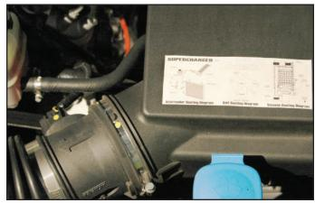
205. Start the vehicle for five seconds and shut off, once again check for fuel leaks and fansupercharger belt alignment. Check radiator and intercooler reservoir levels.
