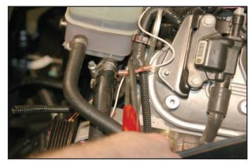
155. Heat shrink your connections to avoid moisture contamination and ensure a good connection.
