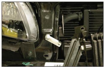
87. Completely remove the existing transmission cooler mounting bracket from the driver side of the transmission cooler. Using a saw or grinder modify the bracket as shown. You're taking off approximately 5/8" from the tab with the upper mounting hole all the way down to the bend in the bracket.
