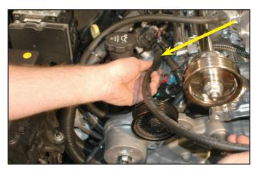
152. Near the front on the passenger side of the supercharger are the two IAT wires exiting the intercooler lid. Attach wire splice connectors to these IAT plug wire ends as shown in the first image. Route the wires from passenger side under the supercharger inlet.
