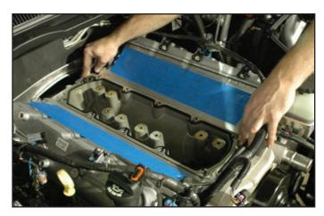
64. Remove the existing O-ring seals from the OEM valley cover, and place in the O-ring grooves of the new provided valley cover.
