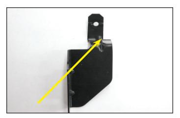
88. Attach the bracket back on the transmission cooler. Using the original bolts, bolt both mounting brackets to the just installed offset mounting brackets. Tighten all bolts using a 10mm socket being careful not to strip threads. NOTE: Cooler lines may still require a little bending to clear the heat exchanger and any other interference areas.
