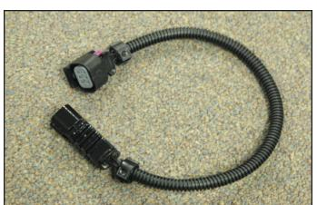
100. Plug the extension into the existing ETC connector, route the wires adjacent to the existing wiring harness to the driver side of the engine.
