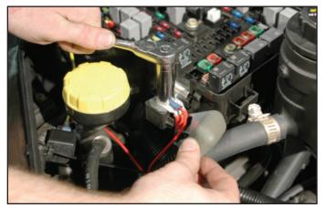
189. Drill a 1/8" diameter hole for the new intercooler pump wire to route to the fusewith-fuse-tap, probably in slot F-37. Thread the yellow wire through the new hole, THEN attach the supplied connector.
