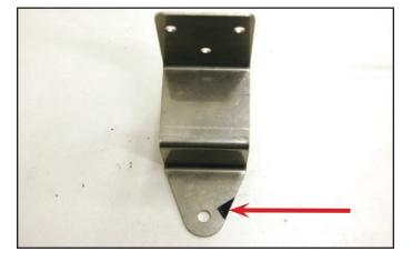
165. Test your fit and adjust as necessary. This is the modified-notched intercooler reservoir bracket, we curved the edges to eliminate any sharp surfaces.
