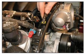
17. Remove the end of the PCV hose from the intake manifold on the passenger side by squeezing the locking tabs and pull free. This will not be reused.
