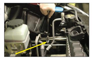
90. Reinstall the transmission cooler hardline on the crossover rail also inserting the new provided spacer between the frame and the bracket using the provided bolt. Tighten using a 10mm socket.
