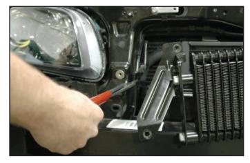
86. Attach the remaining heat exchanger offset bracket to the existing bolt hole where the transmission cooler was originally mounted.
