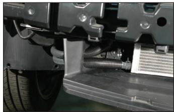
175. Cut 31" of the remaining 3/4" hose and connect one end to the water pump inlet barb using the supplied clamps.
