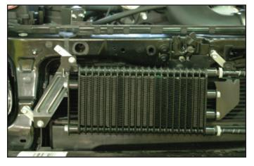
89. Reinstall the transmission cooler hardline on the driver side frame rail inserting the new provided spacer between the frame and the bracket using the provided bolt. Tighten using 10mm socket.
