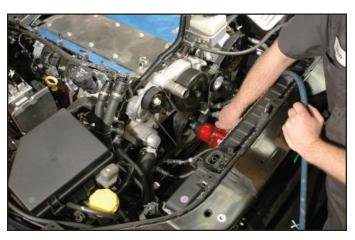
48. Install the supplied drill guide using the supplied bolt and tighten to 30 ft-lbs with a 24mm socket and torque wrench.
