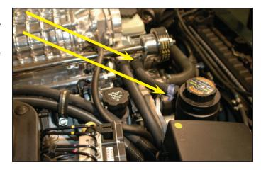
178. Use the supplied zip ties to anchor hose bundles, and sections of split loom to protect hoses from chafing edges.
