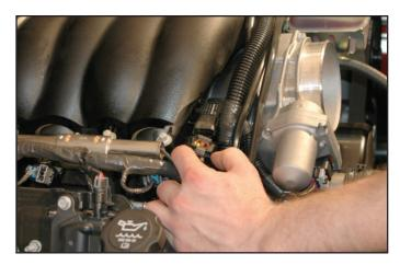
14. Disconnect the eight Injector plugs on each side of the engine.
