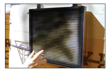
78. Using a 10mm socket, remove the three M6 transmission cooler bolts from the fascia frame mounting brackets.
