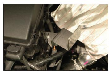
168. Attach reservoir to the mounting bracket with the three supplied bolts. Ensure that there is no reservoir bottle to existing bracket contact.
