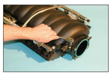
112. Use a 10mm socket wrench to unbolt the stock Fuel Rails from the stock intake manifold.
