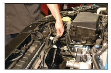
42. Push down on the top of the Transmission Heat Exchanger hoses so that they disconnect from the mounting clips of the lower Fan Shroud housing.
