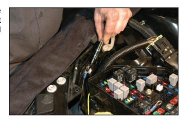
188. Remove the hot lead nut from the front of the fuse box with a 13mm wrench. Add the new hot lead wire and replace the nut.
