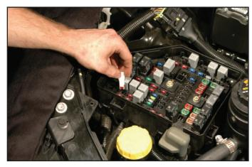
181. Slip the supplied fuse tap over one leg of the OEM 10Amp fuse from the last step.
