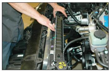
83. Cut a section of the 3/4" hose to 59" in length. Connect one end of the hose to the top barb of the just installed intercooler heat exchanger and clamp using the provided clamp. Run this hose down behind the frame and temporarily out the front of the radiator cowl at the bottom-passenger side.
