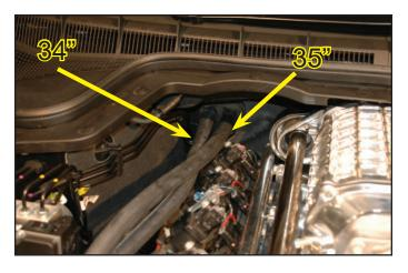
136. Using the supplied 6 x 45mm bolts, 1" spacer, and double hose clamp, install the clamp with the mount hole facing down over the just installed two heater hoses. Slide the bolt through the clamp, and put the spacer on the bottom of the bolt. Install the bolt into the second hole of the coil bracket on the passenger side (the one left out in step 131). Torque bolt to 106 in-lbs.
