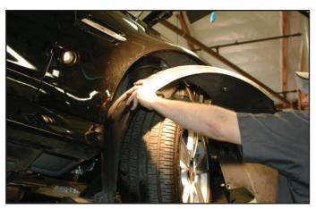
28. As the case may be, bend the panel toward the rear of the vehicle. Then use a 10mm socket to remove the two front end bolts on each side of the vehicle holding the front body panel to the upper fender section. This shows the fender well removed completely.
