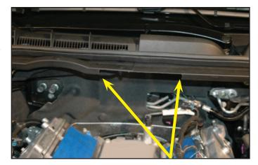
106. The power steering reservoir mount will need to be spaced-outward to maintain clearance with the new throttle body location. Remove the power steering reservoir by levering out on the metal locking tab, then slide the bottle up to remove.
