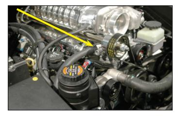
174. Cover hoses passing through plastic cowl with sections of the supplied split loom to avoid chafing and wear.
