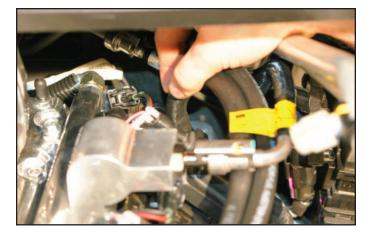
146. Connect the other end to the front of the supercharger barb on the driver side as shown.
