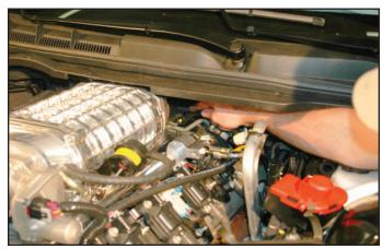
143. Cut 20" of the supplied 5/16" hose and install the remaining end (removed in step 139) onto the EVAP Solenoid as shown.
