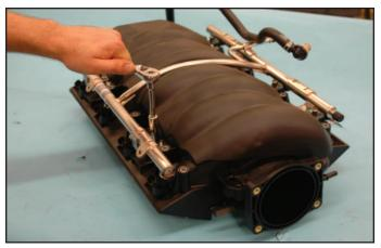
113. Unsnap and remove the clips holding the fuel injectors to the stock fuel rails, and remove the injectors. Note: There will be fuel leakage from the injectors and fuel inside the fuel rails. Take care to have an appropriate catch pan and shop rags handy, then dispose of the fuel collected and any rags used properly.
