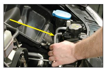
40. Reroute the secondary coolant to crossover tube out of the way. You can bend it to run out the other side of the radiator cap.
