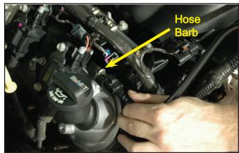
11. Use the 7mm socket to loosen the clamps holding the air intake tube to the throttle body and remove the air intake tube. This assembly will not be reused.
