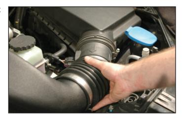
194. Connect the other end of the inlet tube to the supercharger inlet. Tighten all clamps.
