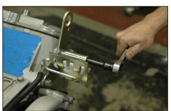
108. Mark the bracket as shown in the picture. On the edge closest to the passenger side bolt, make a mark adjacent to the bolt witness mark. The material to the outside of your mark will have to be removed.
