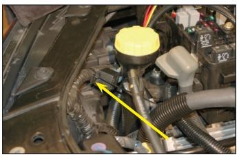
185. Route the intercooler control plug wires down along the hoses, zip tie as handy and plug into the intercooler pump receptacle.
