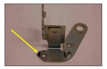
109. Use a grinder or suitable file to remove the material. Your final result should look like this. Dress the edges to avoid sharp surfaces.
