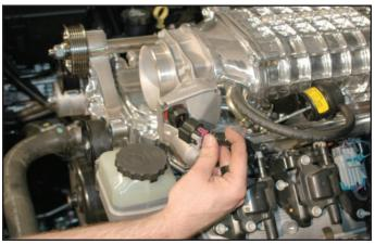
133. Attach the stock plug connectors back on to the coils on the coil brackets.
