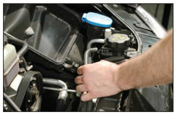
97. Now re-install the upper radiator hose and secure in place with the stock clamps. The coolant overflows can now be relocated to the stock locations and clips on the radiator fan shroud.
