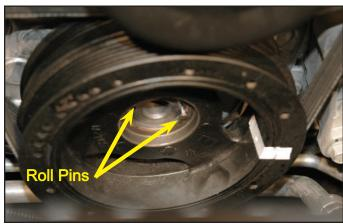
55. The use of a small hammer and punch may be necessary to tap the pins in. Make sure that the pins are in far enough that they do NOT touch the balancer bolt.
