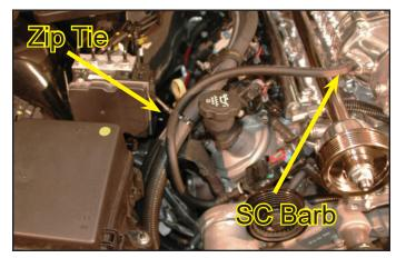
145. Cut 20" of the 3/8" hose, install on the PCV valve barb at the rear on the driver siderear valve cover as shown.
