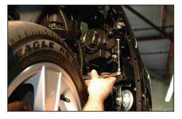
29. On the passenger side of the vehicle, front of the fender well, unplug the connector that splits to go to the parking lights (fog lights), and the side marker illuminating reflector.
