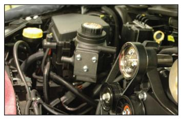
169. At the front-bottom-passenger side of the plastic radiator cowl, drill two 1-1/4" holes through the plastic cowl for the heat exchanger hoses as shown. Connect the holes by cutting the plastic between them, clean and dress the hole to remove sharp edges.
