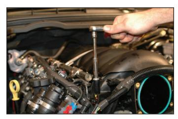
24. Remove the stock intake manifold and put aside, you will be taking some parts off from the bench.
