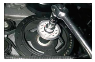
58. Using a 15mm socket on the Tensioner Pulley bolt, spring the pulley down to remove tension on the drive belt and remove the belt when tension has been released.
