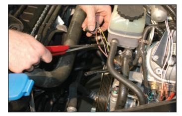
154. Crimp the wires you just cut from the MAF connector, to the IAT sensor wires you routed under the supercharger inlet in step 159. The selection of the wire to connect to either terminal is of no consequence.
