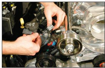
131. Re-attach the modified coil brackets to each side of the engine using the stock hardware. Do NOT install the second bolt back on the passenger side at this time. Torque all remaining bolts to 106 in-lbs. Again, verify your torque wrench settings. Reattach the main coil connector at this time (removed in step 101).
