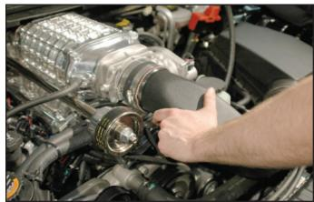
195. Connect the other end of the hose installed in step 151 to the barb on the air tube near the throttle body.
