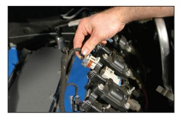
102. Disconnect all plug wires from the coils.
