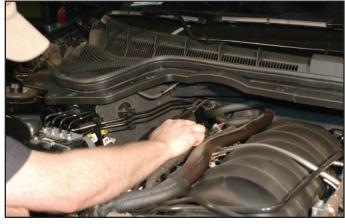
9. Use a 7mm socket to loosen the clamps holding the air bellows to the MAF Sensor.
