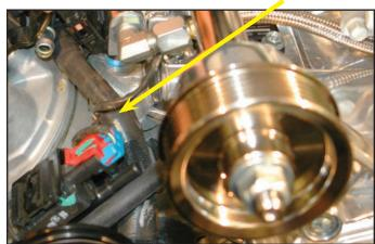
139. Use a sharp blade and split the ends of the EVAP lines and remove the three fittings.
