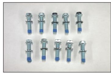
17. Install the supercharger to the heads using the 10 bolts from the last step and torque them to 108 in-lbs. following the order given here and in a larger image at the back of this manual. Gradually work your way up to 108 in-lbs. and ensure that supercharger pulley still spins freely after full torque is applied.
