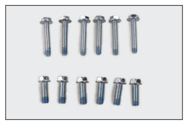
Reinstall the charge air coolers with the 6 M5x35mm bolts that have Loctite 242 applied and torque them to 70 in-lbs.
