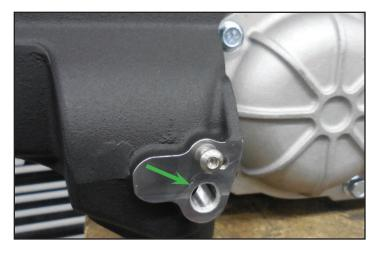
14. Clean the mating surfaces on the heads and supercharger housing prior to installation. Get some assistance when installing the supercharger on the engine. Ensure that gaskets are installed at all 8 ports of the supercharger as shown below.
