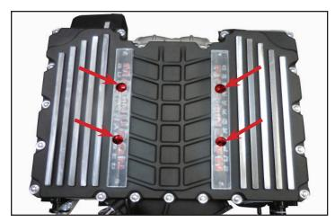
6. Remove the three M6x20mm flange head bolts (red arrows) holding the coolant manifold assembly at the front of the supercharger and pull the manifold out. Repeat this process on the other coolant manifold assembly.
