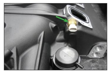
16. Install the provided seal washers on 10 supplied M6x35mm flange bolts and apply Loctite 242 to these bolts.
