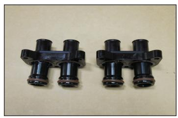
21. Reinstall the coolant manifolds with the 6 M6x20mm flange bolts that have Loctite 242 applied and torque them to 108 in-lbs.
