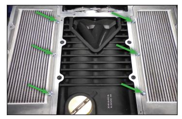
20. Gather the coolant manifolds shown that were removed earlier. Relube all the O-rings with the provided Super Lube prior to reinstalling the coolant manifolds. Carefully rock the tubes in place to prevent the O-rings from being damaged.
