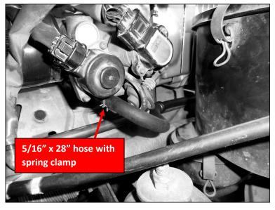
25) Install the 5/16" x 28" from the last step onto the throttle body at the location shown and secure with a provided spring clamp.
