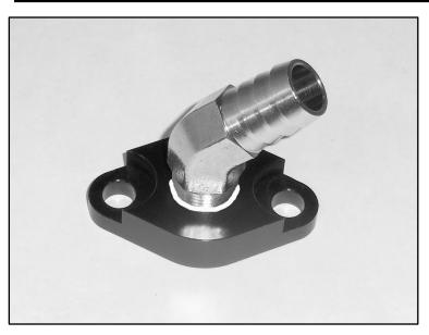
15) Apply Teflon thread sealant to the supplied 45° brass fitting and install it to the supplied heater pipe flange. Clock the fitting as shown.
