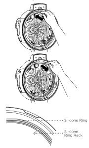
To remove the silicone ring, gently pull it outward, section by section, from the silicone ring rack. The ring can be installed with either side facing up. To reinstall, press it down into the rack section by section, (see image above).
