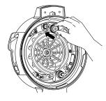
NOTE: Prior to each use, make sure the silicone ring is well-seated in the silicone ring rack and the anti-clog cap is mounted properly on the pressure release valve.
