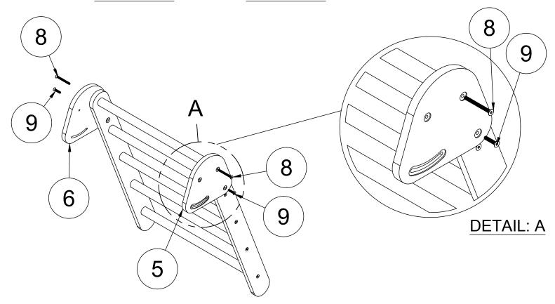
4. Install second Leg Set to Leg Brackets using two- 2-3/4" Bolts.
