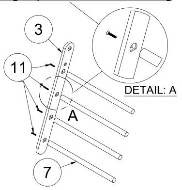
2. Insert top-<u>Dowel</u> and attach **Leg-A** using four-**1-1/2" Bolts**
