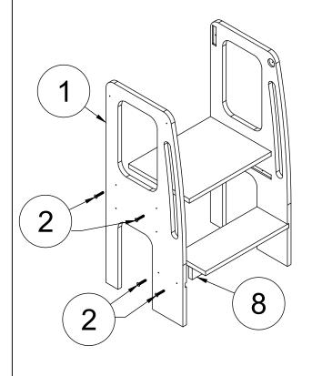
3. Install <u>Front-bar</u> and <u>Back-Dowel</u> using four-1-1/2" bolts.
