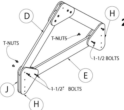
2. Attach Wall Bracket Front-(H) and Wall Bracket Back-(J) to each side of Roof Rail-(D) using 2-T-nuts from Bag #1 and 2-1-1/2" Bolts from Bag #2.
