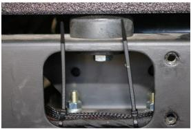
4. Unroll the long rear cable, plug it into the rear harness just installed. Run the cable under the chassis up threw one of the rubber grommets that was cut. Secure the harness using the supplied Cable Ties.
