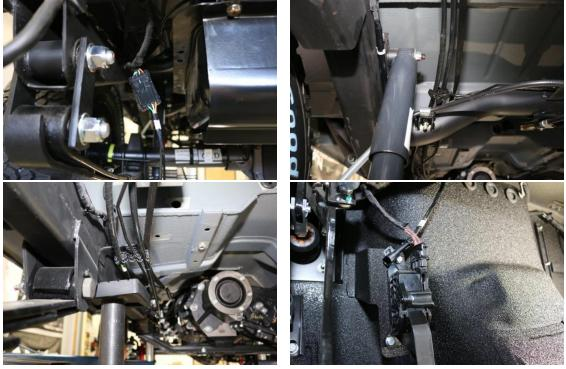
5. Mount the Control Unit under the grommets using two self-tapping screws provided and Plug the Rear Harness in.
