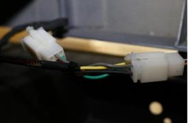
3. Run the other side of the Harness through the bumper over to the passenger side and plug in-line. Secure with cable ties.
