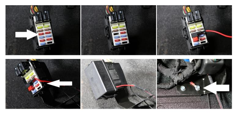
Run the power wire down the slot on the right side and reinstall the fuse cover. Remount the fuse box and using the mounting screw attach the black ground wire as shown.
