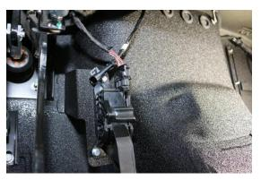
5. Mount the Control Unit as shown under the grommets using two self-tapping screws provided and Plug the Rear Harness in.
