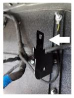
7. Remove the fuse cover and find the 10-amp fuse # F28 as shown and remove.
