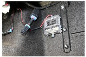
3. Remove the Grommet closest to the relay and cut a slit with a razor blade, remove the fuse and fuse cover and run through the firewall, through the grommet and to the battery, re-install grommet.
