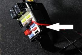
9. Run the power wire down the slot on the right side and reinstall the fuse cover. Remount the fuse box and using the Fuse Mounting screw attach the black ground wire as shown.
