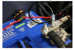
5. Re-install the fuse and cover on the holder and mount on the fire wall with the screw provided. Verify there is no wire or other item on the inside that the self tapping screw can damage or penetrate.
