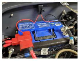
6. Plug the 2-Way power Connector into the Relay 2-way Connector. Run the other end with the fuse over to the fuse block on the passenger side under the dash. To make it easy to work and see the fuses there is a tab on the right side that can be pushed in to release the fuse box, more information can be found in your Instruction Book. Also, it can be removed by removing the 2 screws at the bottom of the bracket, one screw must be removed later to attach the ground wire.
