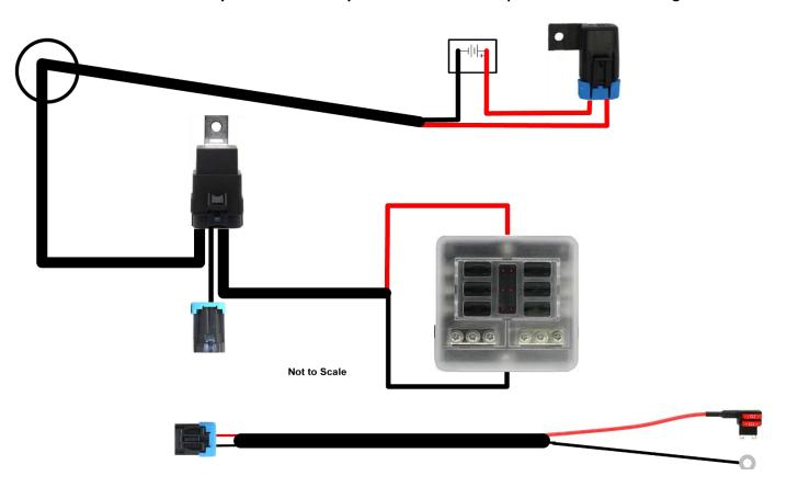
1. Mount the fuse block under the dash on the passenger side as shown with the screws provided. When drilling the 4 mounting holes make sure not do damage the wire harness on the other side.
