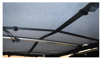
9. Secure (1) right side and (1) left side rear hook and loop straps around Fore Aft ROPS Bar behind "B" Pillar.
