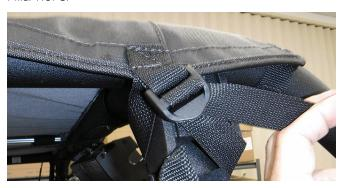
11. Make any final centering adjustments, then tighten all straps, stow (3) roof traps in supplied Strap Keepers.
