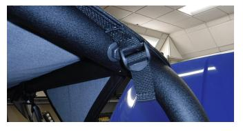
6. Install Center Bow above ROPS with foam facing up, then secure front and rear with hook and loop flaps around bow.
