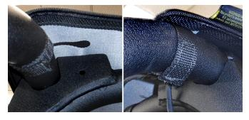
10. Secure (1) right side and (1) left side Rear Corner Straps to "B" Pillar ROPS.
