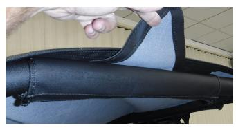
5. Secure (1) right side and (1) left side Front Corner Straps to "A" Pillar ROPS on outside of Fore Aft ROPS Bars.
