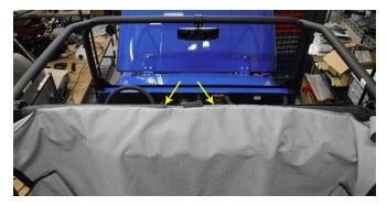
3. Lay Bikini Top forward, toward front ROPS Bar, making sure rear right and left protective flaps are positioned to protect top from "B" Pillar bolt heads.
