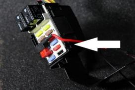
10. Run the power wire down the slot on the right side and reinstall the fuse cover. Remount the fuse box and using the Fuse Mounting screw attach the black ground wire as shown.
