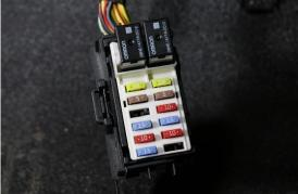
9. Plug the fuse adapter into F28 as shown below.
