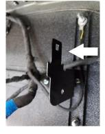
8. Remove the fuse cover and find the 10-amp fuse # F28 as shown and remove.
