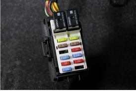
10. Plug the fuse adapter into F28 as shown below.
