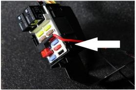
11. Run the power wire down the slot on the right side and reinstall the fuse cover. Remount the fuse box and using the Fuse Mounting screw attach the black ground wire as shown.
