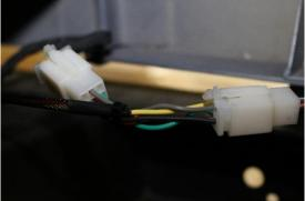
2. Run the other side of the Harness through the bumper over to the passenger side and plug in-line. Secure with cable ties.
