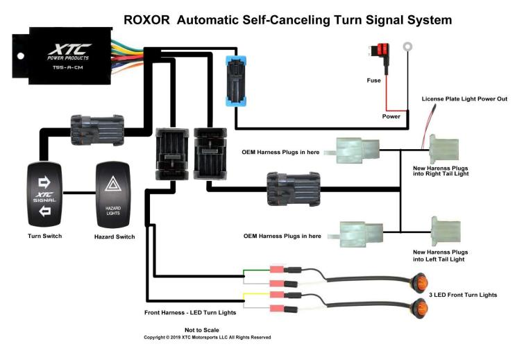
**Dielectric Grease** – We have included a packet of grease. Just like the OEM we recommend using Dielectric Grease on all switch terminals and on the white non-sealed factory connectors on the rear tail lights, this helps keep the water out and it also reduces corrosion and increases reliability! You do not need to put the grease on our four pin **SEALED** Connectors. Open the grease and put on the switch terminals and the connector terminals.
