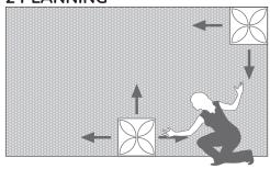
Use a level to mark lines on the wall to ensure straightness and accuracy. Allow cut panels to fall in more inconspicuous areas like corners and the bottom of a wall. If working from the center out, panels that fall at edges may need to be cut. Plan your design well to ensure desired results. Remember, measure twice and cut once.
