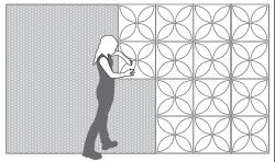
Once panels are in place, apply pressure around the perimeter of the panel and other touchpoints to the wall to lock in place. When all the panels are installed, apply pressure to the entire flat surface to achieve a full bond. After rolled re-positioning is not possible.
