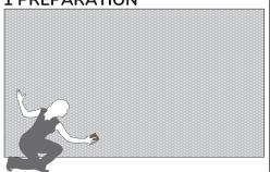
Wall Flats are made to install over a relatively flat and smooth surface that is clean, dry and free of loose debris. A strong bonding primer should be applied to the wall prior to adhesion of the Wall Flats
