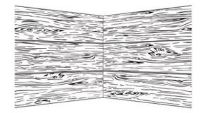
NOTE: If the wall is not 90°, you may need to cut the boards at an angle (MITER) to get a tight fit.
