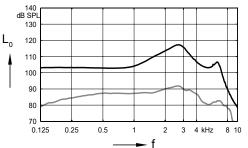
Max. Output sound pressure level  $(L_1 = 90 \text{ dB})$
