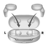
The hearing instruments are automatically turned off and start charging. The charging status is shown for 7 seconds. If the status LEDs do not light up when you insert the hearing instruments, check the following:
