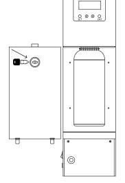
Fill the bottle with scenting oil and 3 place it back onto the machine
