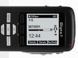
Especially convenient for lefthanded users: Display rotation thanks to the movement sensor which also makes for automatic file storage in case the device should fall to the ground. This mode also ensures that the Digta 7 exits the sleep mode as soon as you pick it up.
