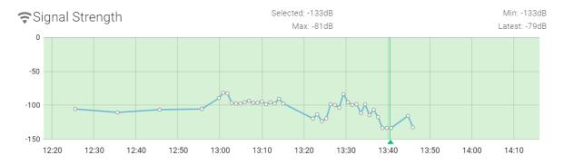
LTE-M received signal strength before Sony intervention. Note the mSafety wearable is capable of communications with signal strength lower than -135dBm, which is significantly more sensitive than a mobile phone.
