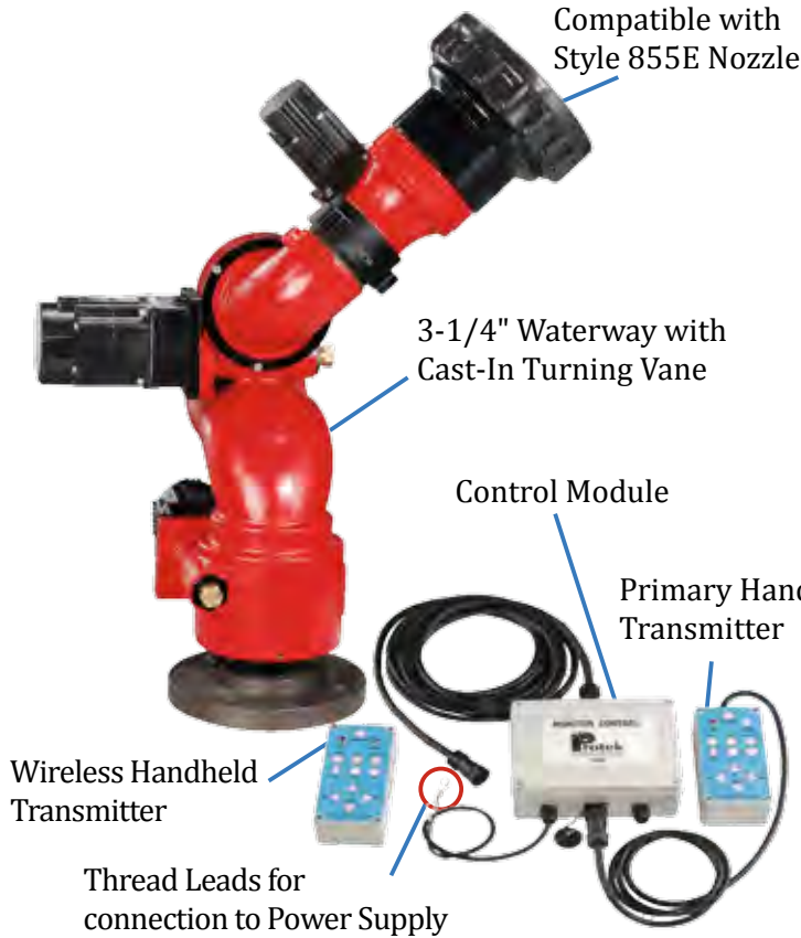
Style 935 monitor shown with standard accessories: Style 855E nozzle, control module, connection cables, panel mount primary transmitter and wireless handheld transmitter
